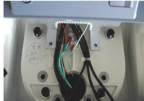
Figure 4-40 Removing cable tie
