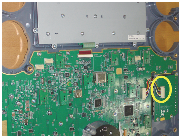
Figure 8-164 Disconnecting TGC BOARD CABLE
