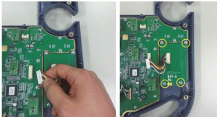
Figure 8-78 Unscrewing 4 screws of TGC control circuit board
