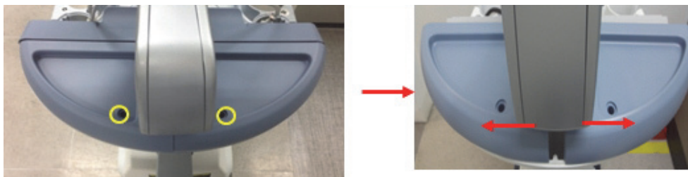
Figure 8-185 Unscrewing 2 screws to remove SPEAKER COVER LEFT/RIGHT
