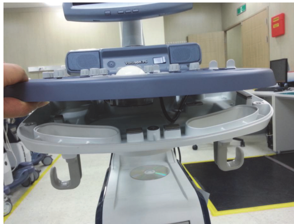
Figure 8-66 Lifting up main keyboard assy
