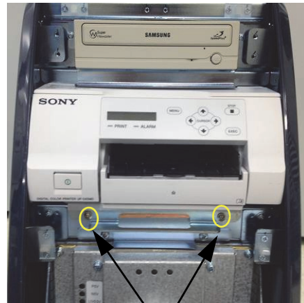
2 screws (2159634 -screw BH M4X10)
