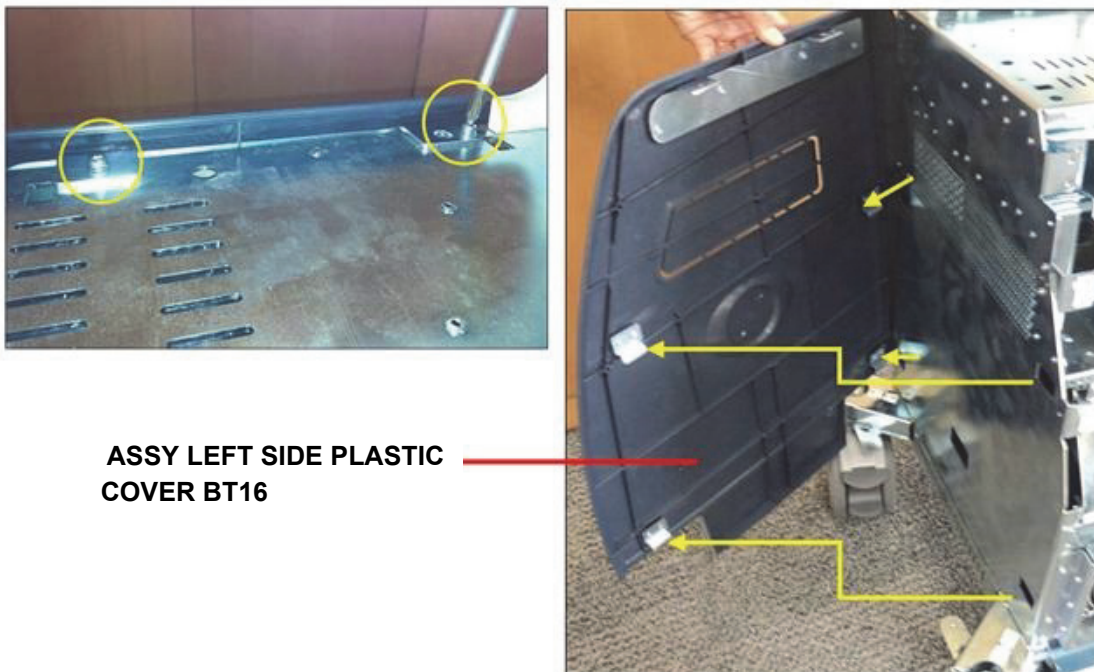
Figure 8-151 Removing the ASSY LEFT SIDE PLASTIC COVER BT16
