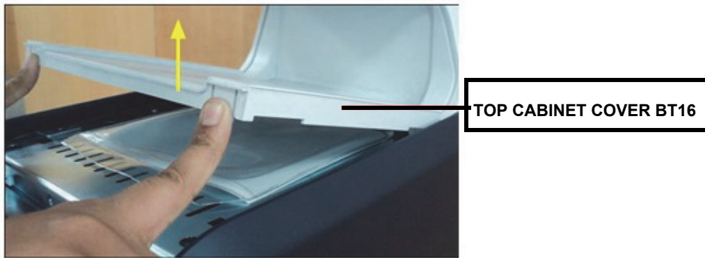
Figure 8-27 Removing the TOP CABINET COVER BT16
