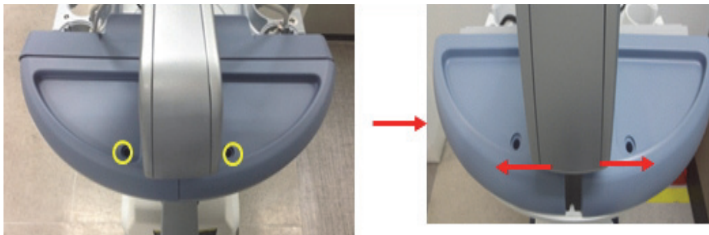
Figure 8-52 Unscrewing 2 screws to remove SPEAKER COVER LEFT/RIGHT
