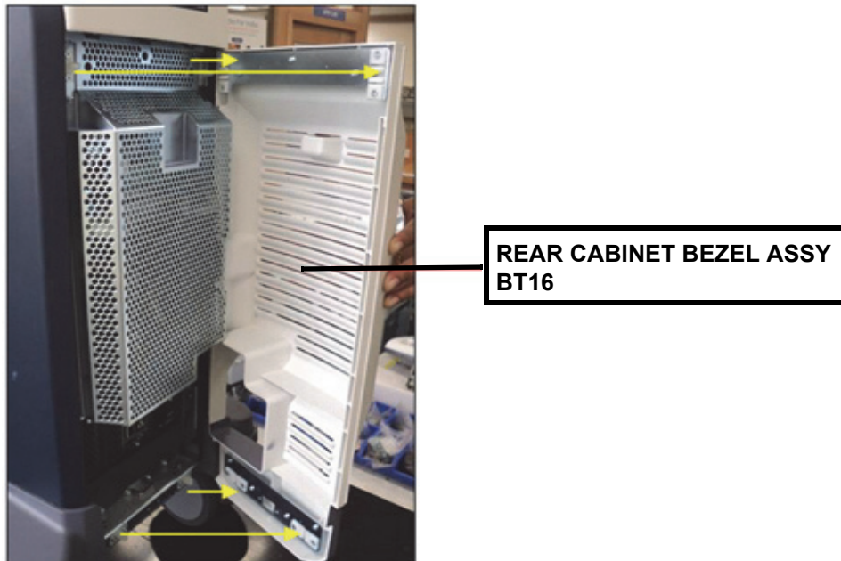
Figure 8-36 Removing the REAR CABINET BEZEL ASSY BT16
