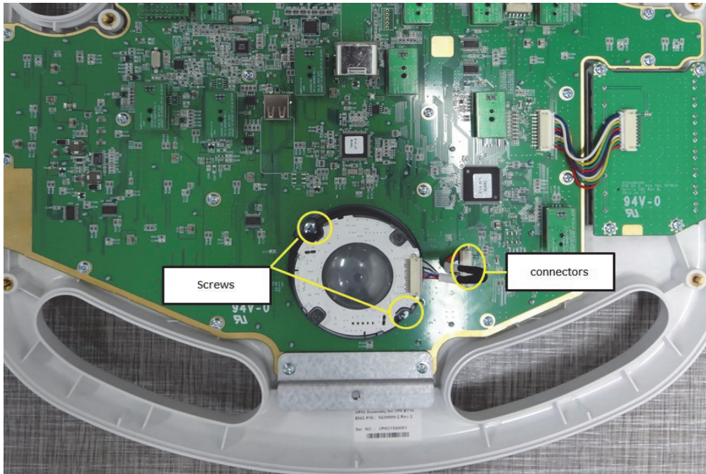
Figure 8-163 Connecting the cable to the connector and screwing the trackball
