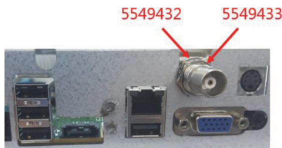
Figure 8-242 Removing the nut and washer
