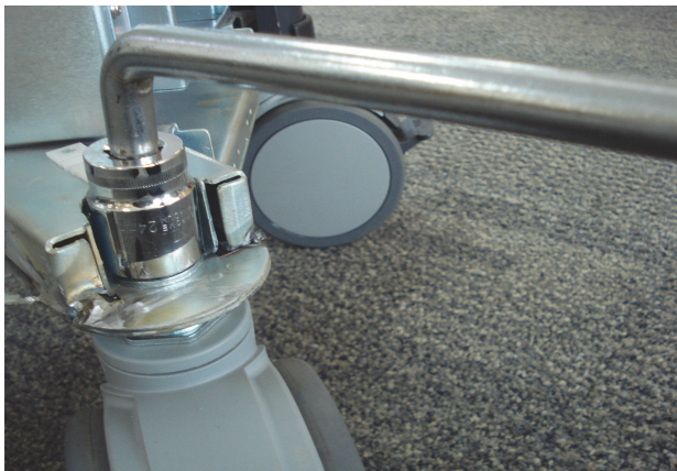
Figure 8-177 Unscrewing the NUT
