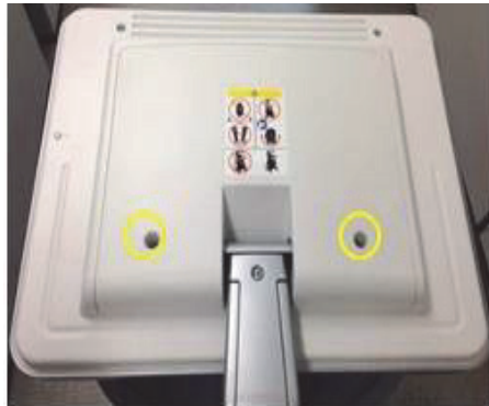
Figure 4-63 Screwing 2 screws to assemble MONITOR CABLE COVER
