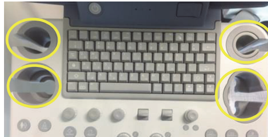
Figure 8-147 Removing the 5 PROBE HOLDERS
