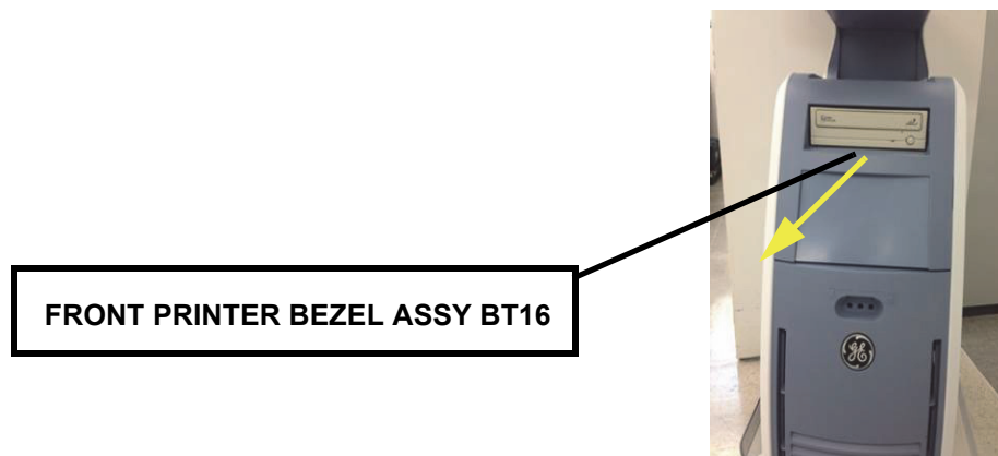
Figure 8-120 Removing the FRONT PRINTER BEZEL ASSY BT16
