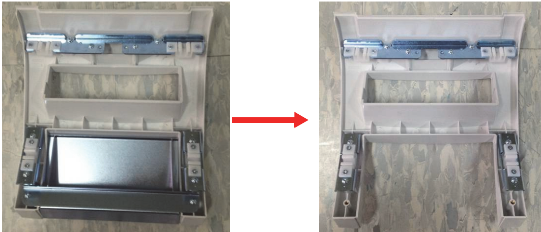
Figure 8-216 Disassembling PRINTER DUMMY COVER PLATE BT16
