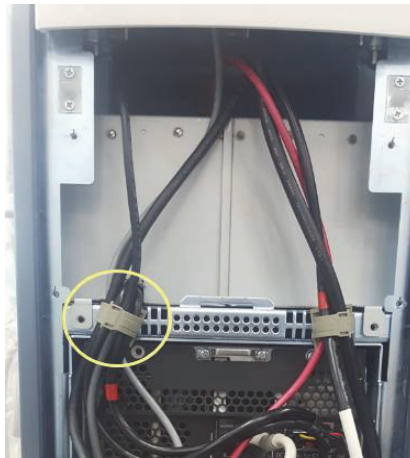
Figure 8-263 Untying cable clamp to unroute WIRELESS LAN Cable
