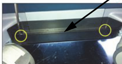
Figure 8-124 Removing the TRAY SIDE CABINET BT16
