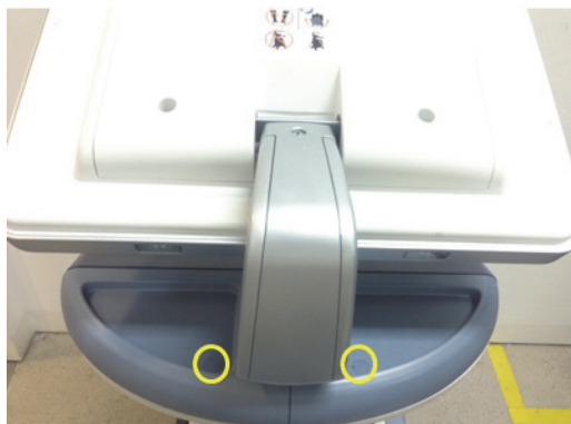
Figure 8-105 Removing 2 RUBBER CAPS on SPEAKER COVER LEFT/RIGHT
