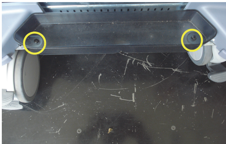
Figure 8-178 Unscrewing 2 screws and remove SIDE CABINET TRAY BT16
