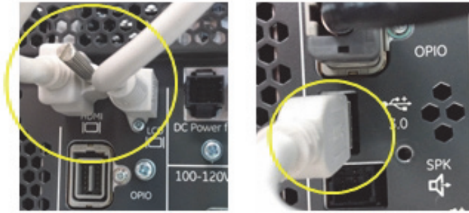
Figure 8-118 Disconnecting Monitor cables
