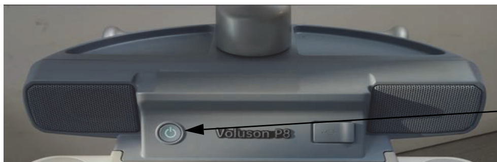
Figure 3-14 On/Off Button on Control Panel
