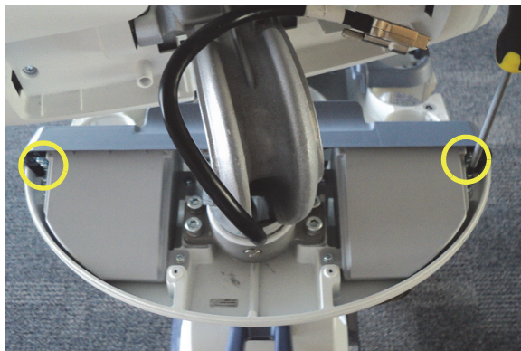
Figure 4-56 Screwing 2 screws and assembling the upper keyboard assembly
