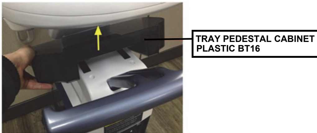
Figure 8-32 Removing the TRAY PEDESTAL CABINET PLASTIC BT16
