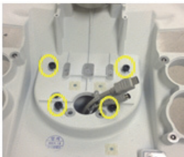
Figure 4-48 Assembling the keyboard base
