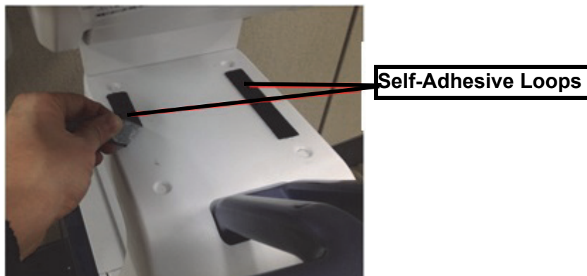
Figure 8-33 Removing the two Self-Adhesive Loops
