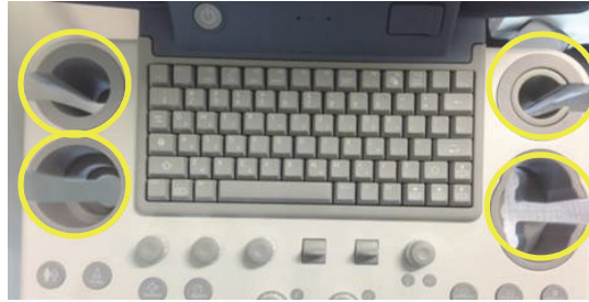
Figure 8-65 Removing 5 probe holders
