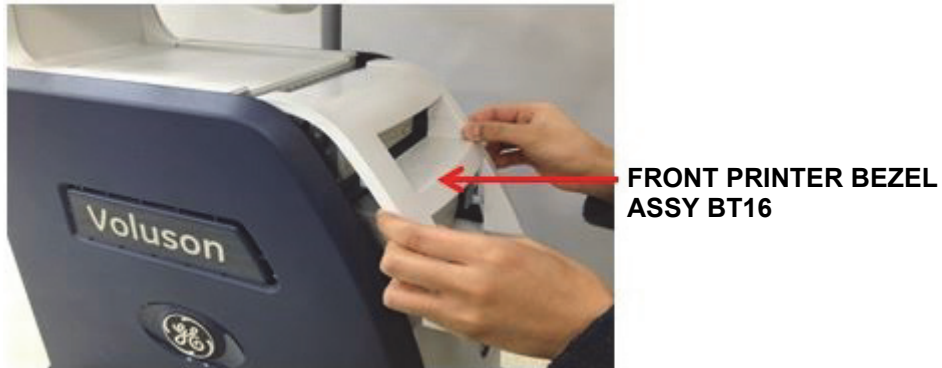
Figure 8-109 Removing the FRONT PRINTER BEZEL ASSY BT16
