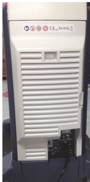
Assemble REAR CABINET BEZEL ASSY BT16, power cord and POWER CORD FIX BRACKET
