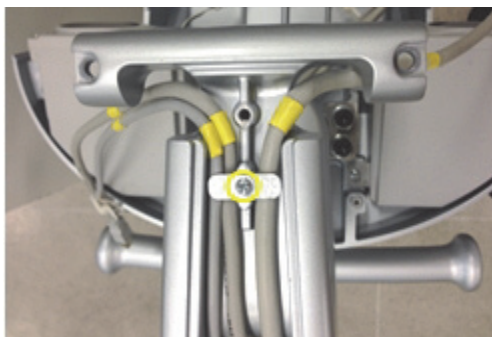
Figure 4-50 Routing the cables and screw 1 screw to re-assemble MONITOR CABLE FIX BRACKET
