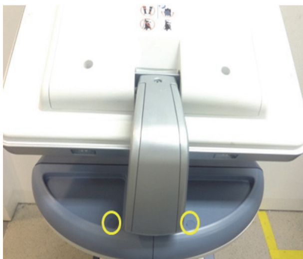
Figure 8-184 Removing 2 RUBBER CAPS on SPEAKER COVER LEFT/RIGHT
