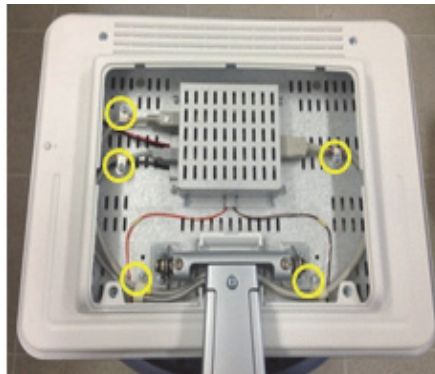
Figure 8-102 Unscrewing 5 screws to disconnect the LCD Cables
