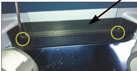
Figure 8-173 Removing the SIDE CABINET TRAY BT16
