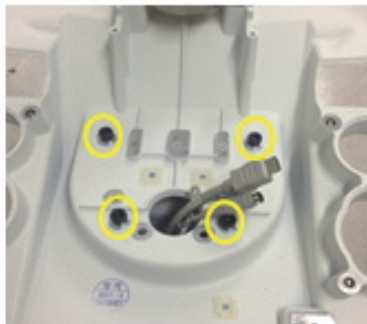
Figure 4-44 Unscrewing 4 screws to disassemble keyboard base
