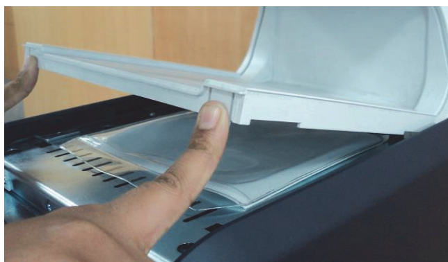
Figure 8-11 Disassembling the Top Cabinet Cover
