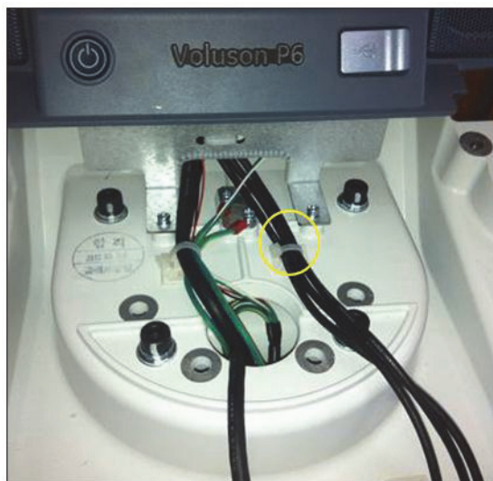
Figure 8-134 Cutting the CABLE TIE by nipper
