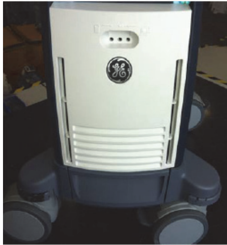
Figure 8-145 Removing the FRONT CABINET BEZEL ASSY BT16
