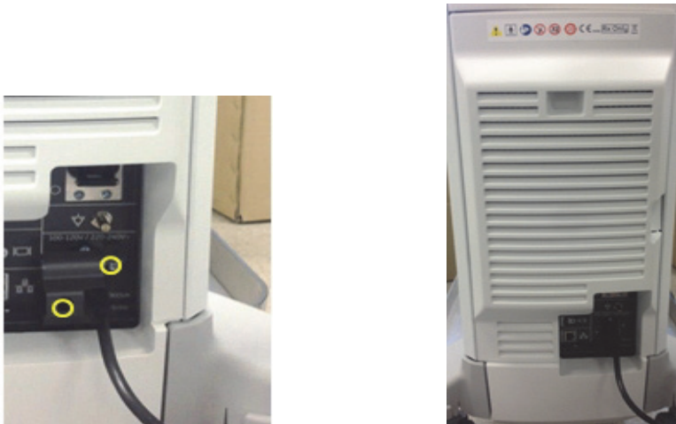
Figure 8-217 Disassembling REAR CABINET BEZEL ASSY BT16
