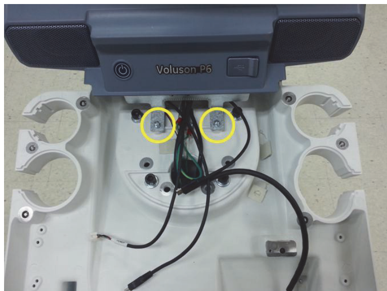
Figure 8-86 Unscrewing 2 screws on the system body
