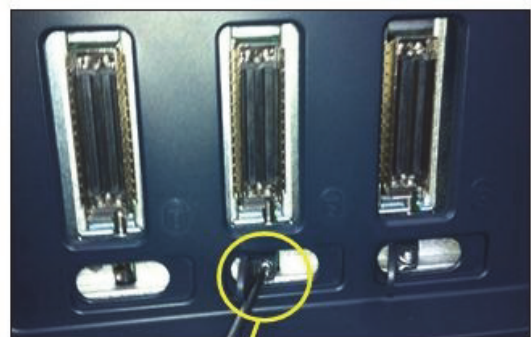
Removing second RS Knob
