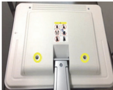
Figure 8-101 Unscrewing 2 screws to remove the MONITOR REAR CABINET BEZEL ASSY BT16
