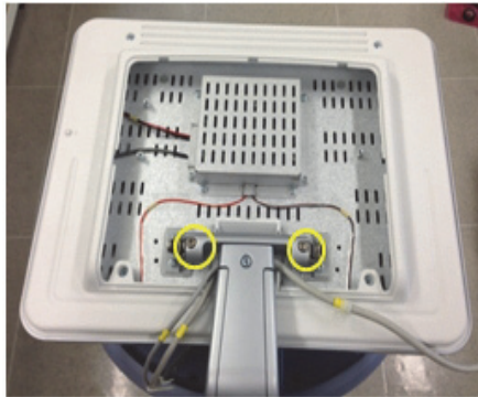
Figure 8-93 Unscrewing 2 hexagonal screws to separate MONITOR
