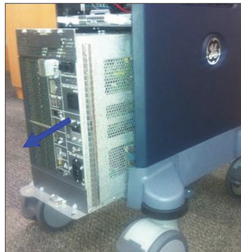
Figure 8-144 Unscrewing 4 screws and removing the NEST BOX
