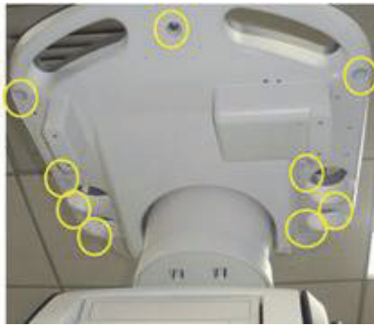
Figure 4-59 Screwing 9 screws under the KEYBOARD BASE
