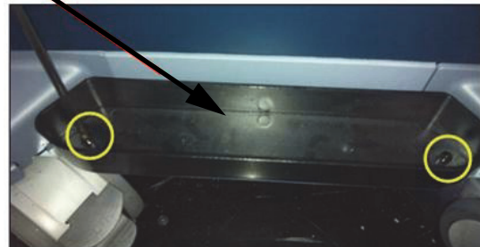
Figure 8-173 Removing the SIDE CABINET TRAY BT16
