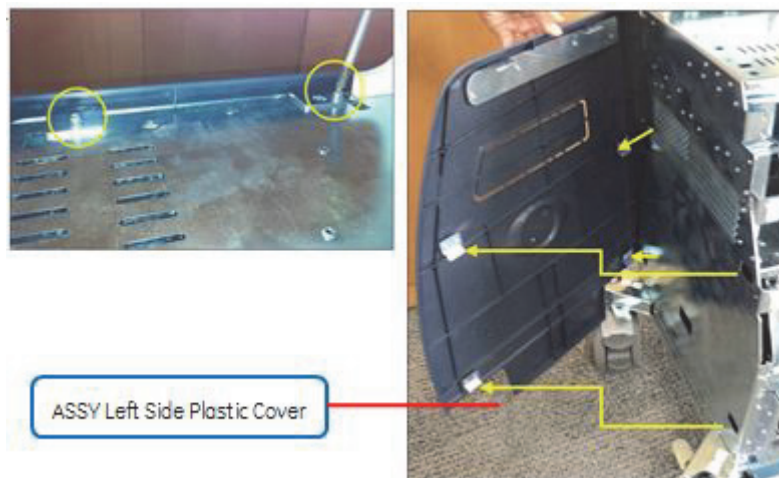
Figure 8-125 Removing the ASSY Left Side Plastic Cover
