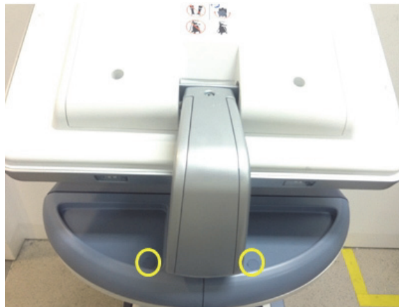
Figure 4-29 Removing the RUBBER CAPS
