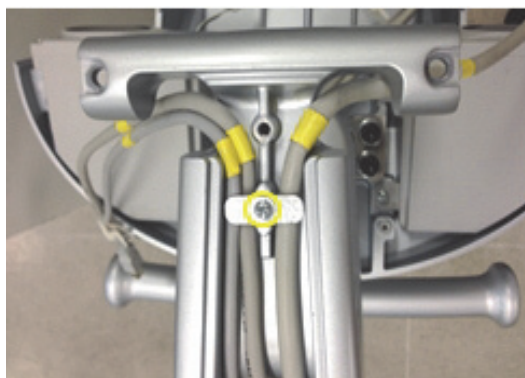
Figure 4-33 Unscrewing 1 screw to remove MONITOR CABLE FIX BRACKET
