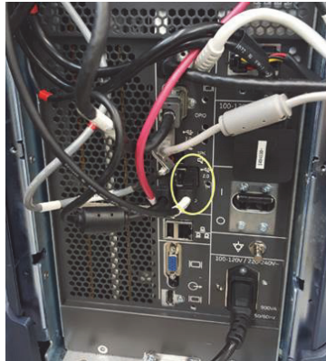
Figure 8-262 Disconnecting WIRELESS LAN cable from NEST BOX
