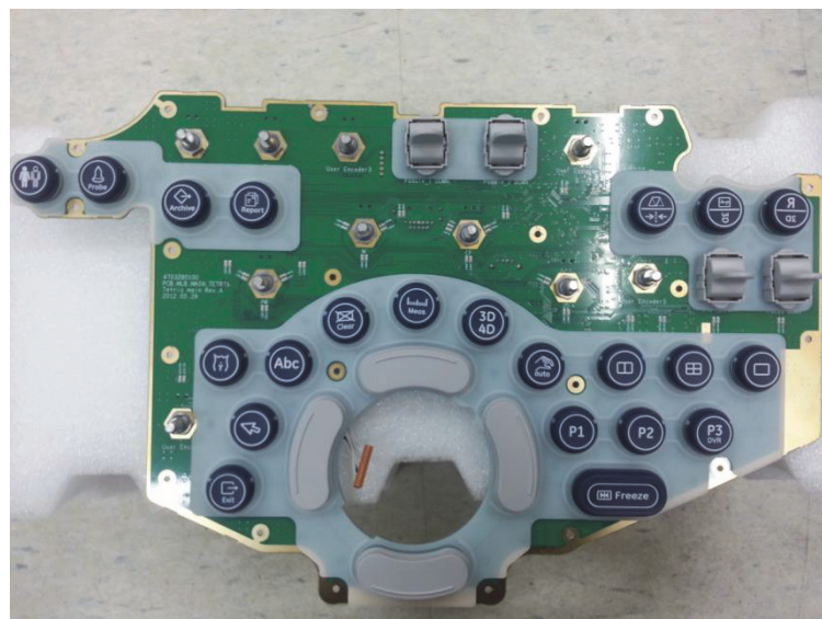
Figure 8-71 Removing the button
