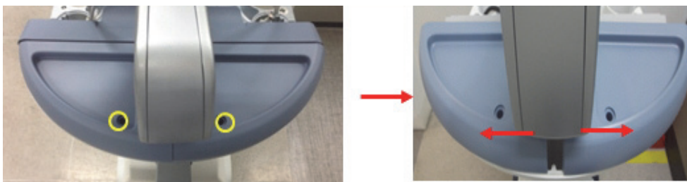
Figure 8-106 Unscrewing 3 screw to remove SPEAKER COVER LEFT/RIGHT
