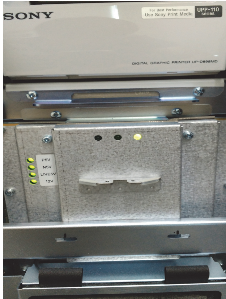
Figure 7-6 Check green LED on backplane
