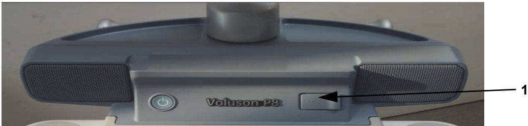
Figure 5-17 External I/O Connectors - on the TOP OPIO
