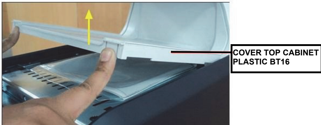
Figure 8-154 Removing the COVER TOP CABINET PLASTIC BT16
