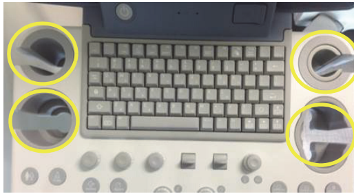
Figure 8-73 Removing 5 probe holders
