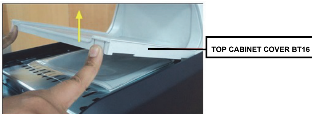
Figure 8-29 Removing the TOP CABINET COVER BT16
