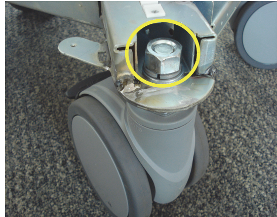
Figure 8-177 Unscrewing the NUT
