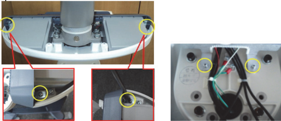
Figure 8-135 Unscrewing 4 screws to remove upper keyboard assembly
