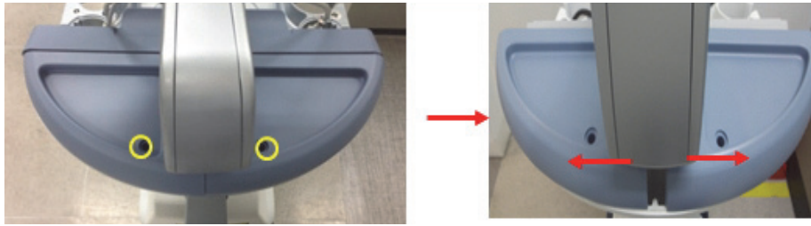
Figure 8-96 Unscrewing 2 screws to remove SPEAKER COVER LEFT/RIGHT
