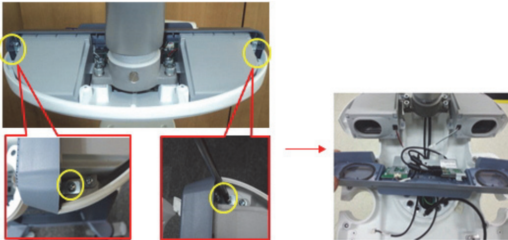
Figure 8-53 Removing Upper keyboard Assy
