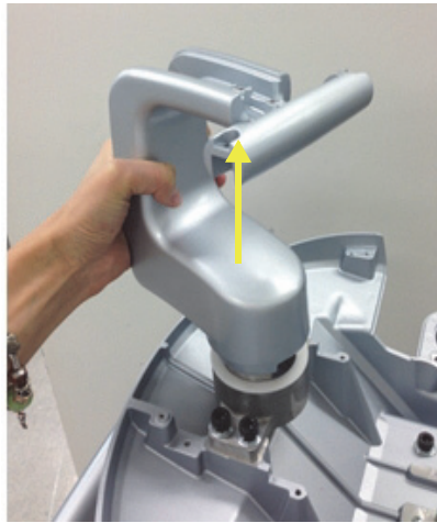
Figure 8-100 Pulling out the LCD ARM from the LCD ARM HOLDER
