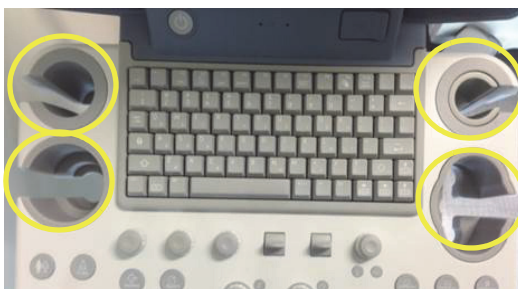
Figure 8-158 Removing 5 probe holders
