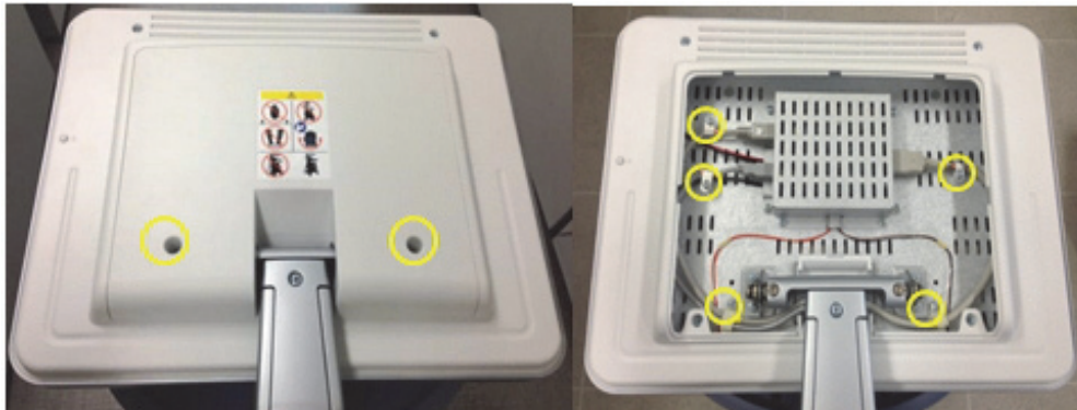
Figure 4-31 Removing the MONITOR CABLE COVER and cables
