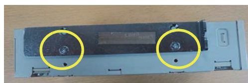
Figure 8-210 Removing the SIDE STRIPS
