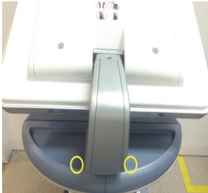
Figure 8-51 Assembling 2 RUBBER CAPS on SPEAKER COVER LEFT/RIGHT
