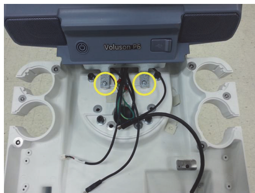
Figure 8-50 Unscrewing 2 screws on the system body
