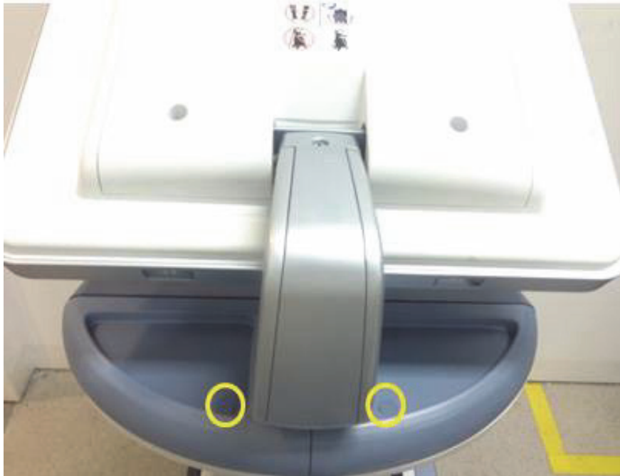
Figure 4-62 Assembling 2 Rubber cap on speaker cover left/right
