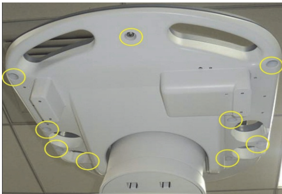
Figure 8-132 Unscrewing 9 screws located on the bottom of the OPIO
