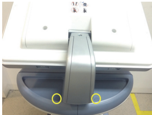
Figure 8-95 Removing 2 RUBBER CAPS on SPEAKER COVER LEFT/RIGHT
