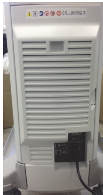
Figure 8-116 Disassembling power cord and REAR CABINET BEZEL ASSY BT16
