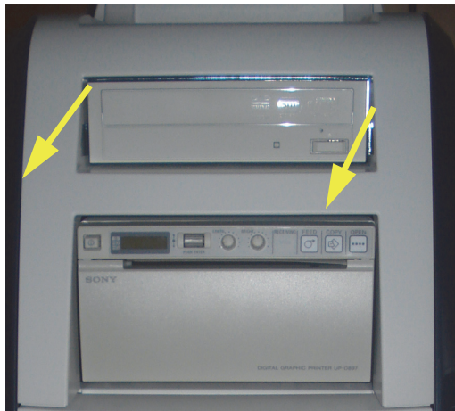
Figure 8-207 Removing FRONT PRINTER BEZEL ASSY BT16
