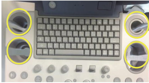
Figure 8-83 Removing 5 probe holders
