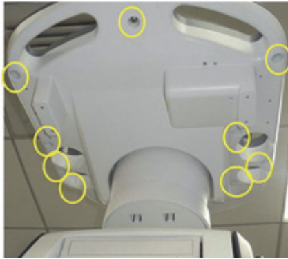
Figure 4-34 Unscrewing 9 screws under the keyboard base
