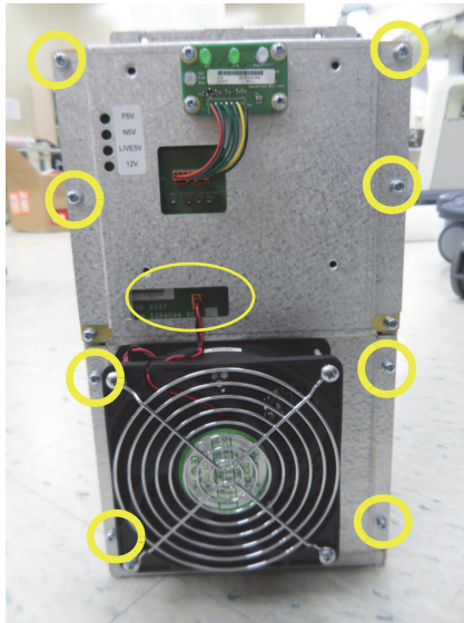
Figure 8-205 Removing fan connector and unscrewing 8 screws
