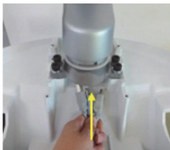
Figure 4-49 Re-assembling LCD cables through the LCD ARM.
