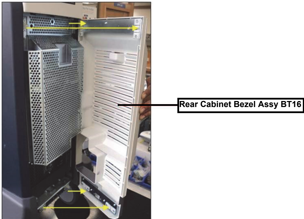
Figure 8-171 Removing the Rear Cabinet Bezel Assy BT16
