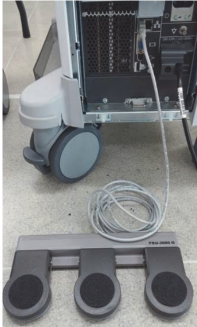
Figure 3-10 Footswitch connection scheme
