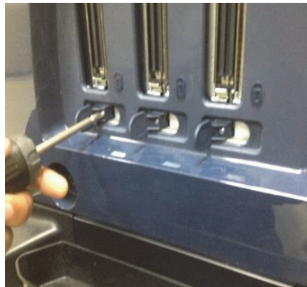
Figure 8-248 Removing 3 RS Knobs
