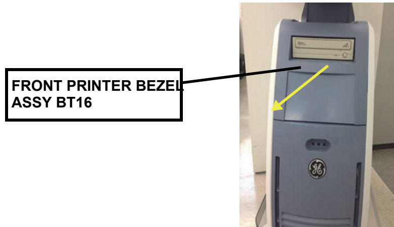
Figure 8-169 Removing the FRONT PRINTER BEZEL ASSY BT16
