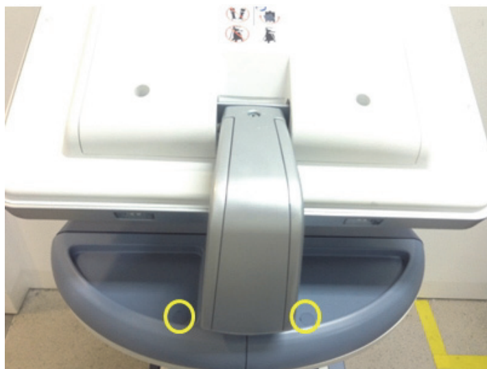
Figure 8-61 Removing 2 RUBBER CAPs on SPEAKER COVER LEFT/RIGHT
