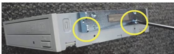
Figure 8-210 Removing the SIDE STRIPS
