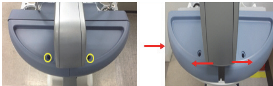
Figure 8-62 Unscrewing 2 screws to remove SPEAKER COVER LEFT/RIGHT
