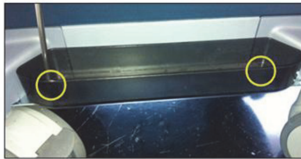
Figure 8-152 Removing the Tray Side Cabinet
