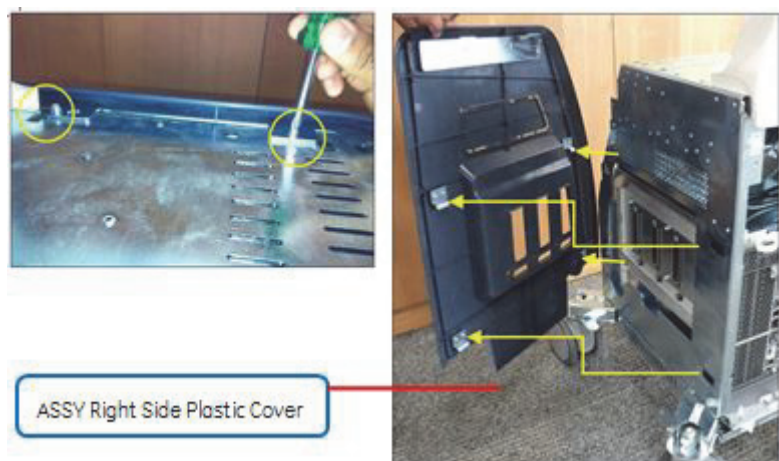
Figure 8-126 Removing the ASSY RIGHT SIDE PLASTIC COVER BT16
