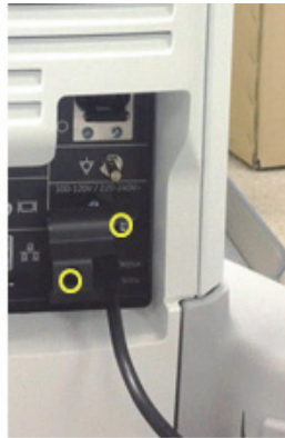
Figure 8-115 Unscrewing 2 screws to remove POWER CORD FIX BRACKET
