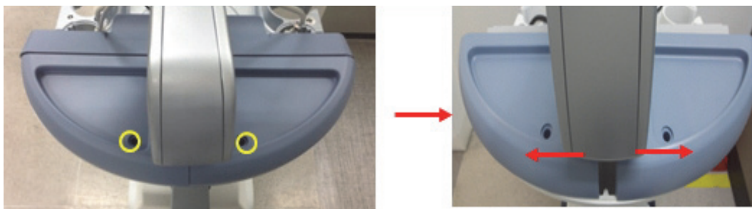
Figure 4-30 Unscrewing 2 screws to remove SPEAKER LEFT and RIGHT
