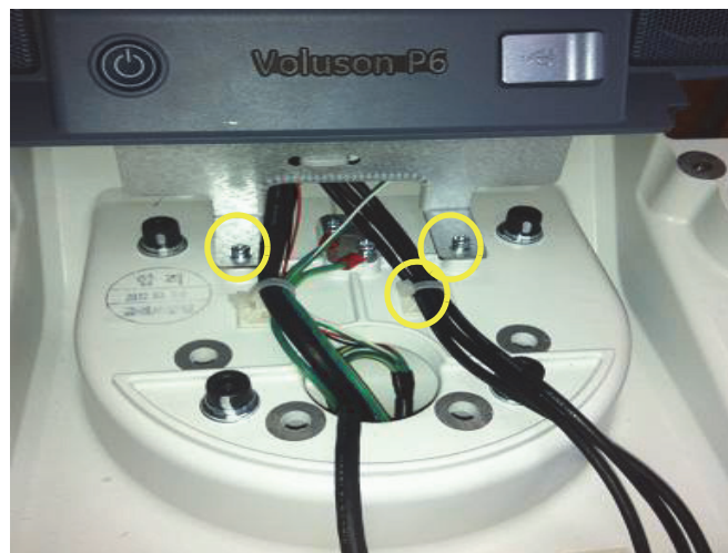
Figure 8-60 Unscrewing 2 screws and removing cable tie on the system body
