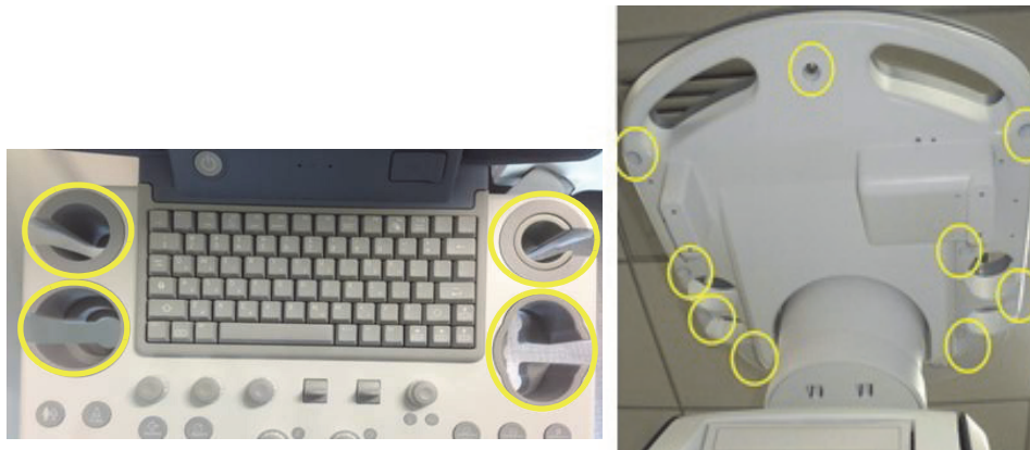
Figure 8-251 Removing 5 Probe holders and unscrewing 9 screws below the keyboard base
