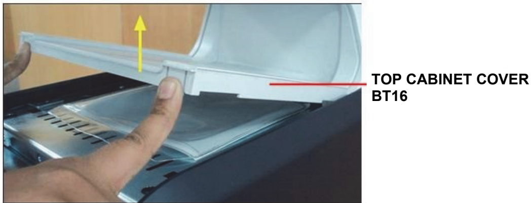
Figure 8-180 Removing the TOP CABINET COVER BT16
