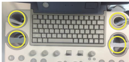
Figure 8-38 Removing 5 probe holders
