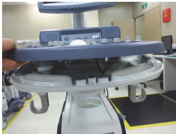
Figure 8-84 Lifting up main keyboard assy
