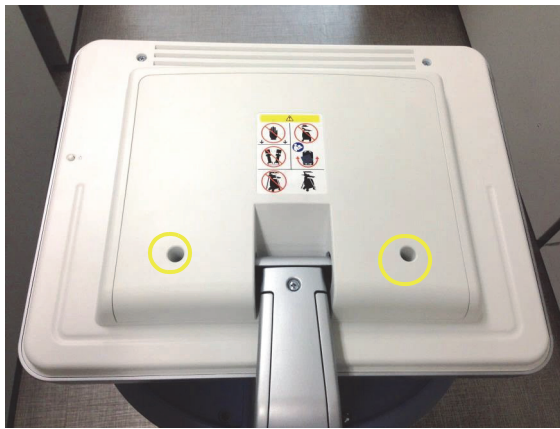
Figure 8-91 Unscrewing 2 screws to remove the Monitor REAR CABINET BEZEL ASSY BT16
