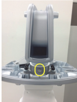
Figure 8-99 Unscrewing LCD ARM STOPPER SCREW
