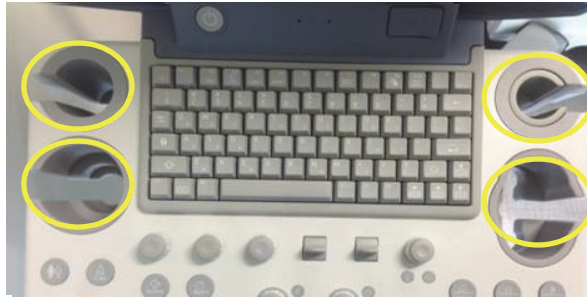
Figure 8-131 Removing the 5 probe holders
