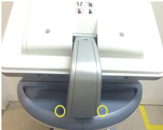
Figure 8-129 Removing 2 RUBBER CAPS on SPEAKER COVER LEFT/RIGHT
