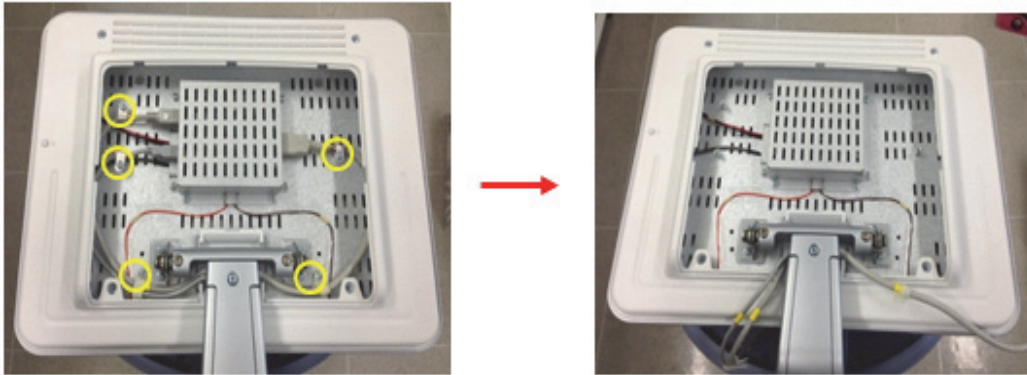
Figure 8-92 Unscrewing 5 screws to disconnect the LCD cables
