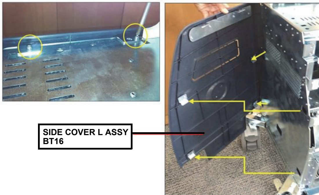
Figure 8-174 Removing the SIDE COVER L ASSYBT16
