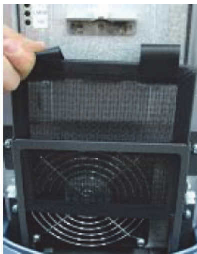
Figure 8-146 Removing the AIR FILTER
