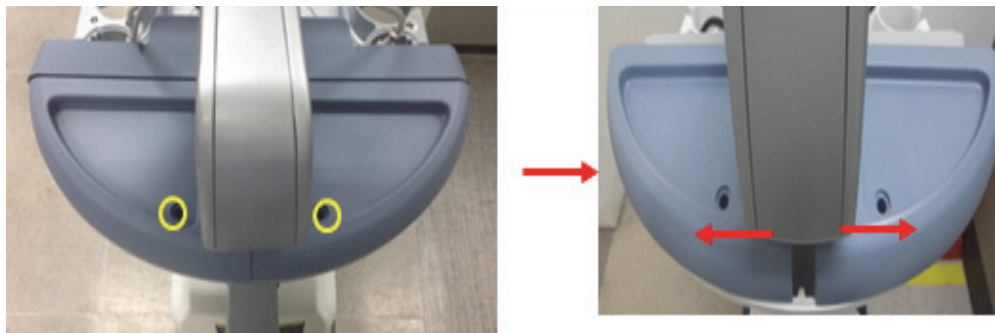
Figure 8-88 Unscrewing 2 screws to remove SPEAKER COVER LEFT/RIGHT
