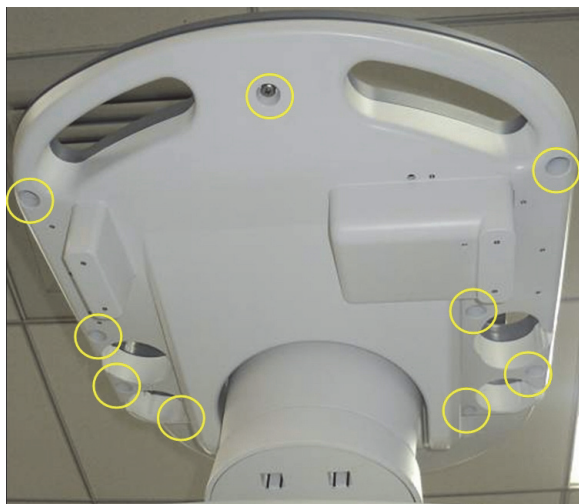
Figure 8-107 Unscrewing 9 screws at the bottom of the OPIO
