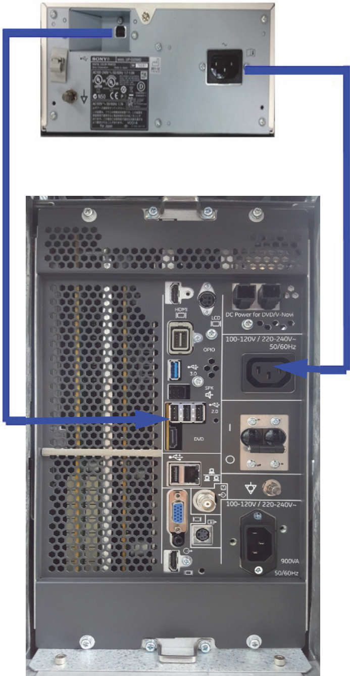
Figure 3-7 Color Printer connection
