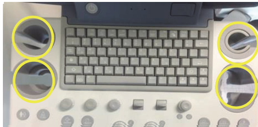
Figure 4-35 Removing 5 probe holders
