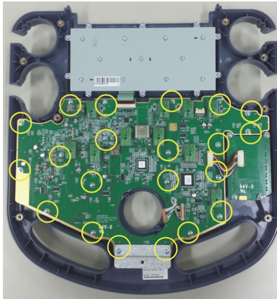
Figure 8-70 Lifting up the main keyboard circuit board after unscrewing 21 screws and disconnecting TGC cable
