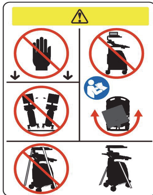
Figure 1-1 Monitor caution label (on rear of the Voluson™ P8/Voluson™P6 system)
