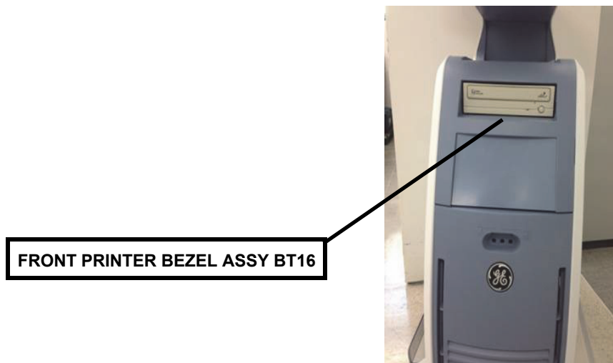
Figure 8-28 Removing the FRONT PRINTER BEZEL ASSY BT16
