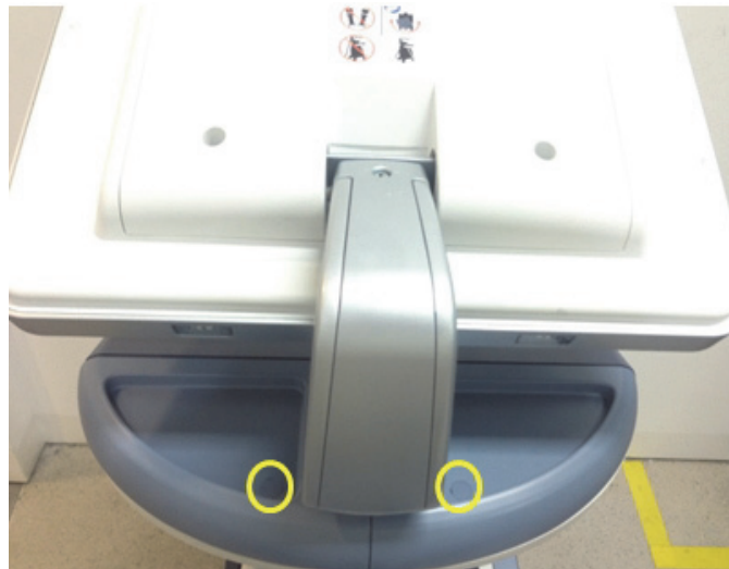
Figure 8-87 Removing the RUBBER CAPS
