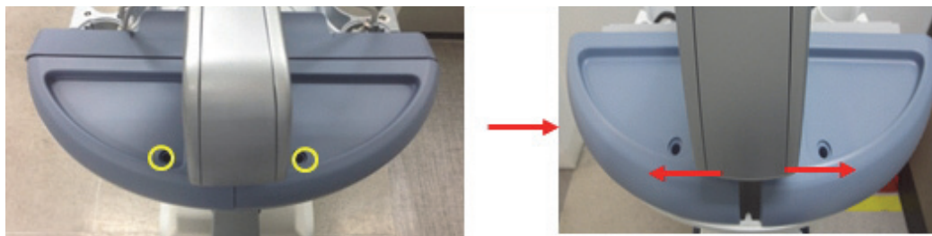
Figure 8-130 Unscrewing 2 screws to remove SPEAKER COVER L/R
