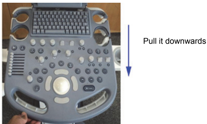
Figure 4-36 Removing lower keyboard assembly
