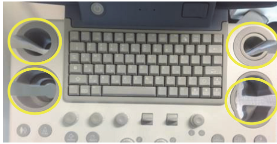
Figure 8-57 Removing 5 probe holders
