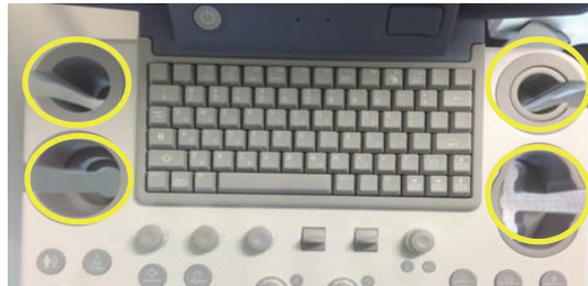
Figure 4-60 Assembling 5 probe holders
