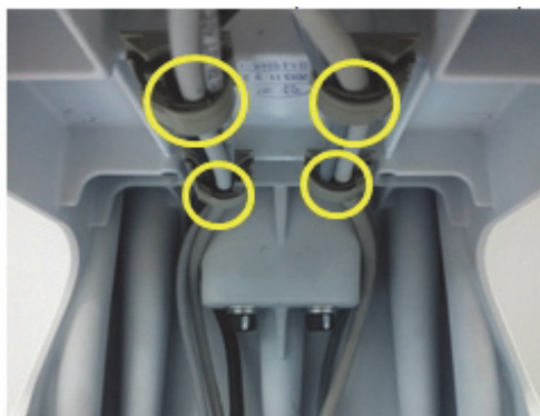
Figure 8-114 Untying the cable clamps
