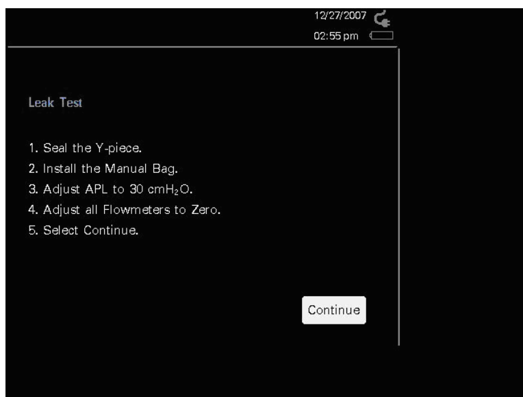
FIGURE 6-16 Leak Test Setup
