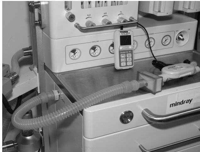
FIGURE 5-9 Connecting the Flow Analyzer
