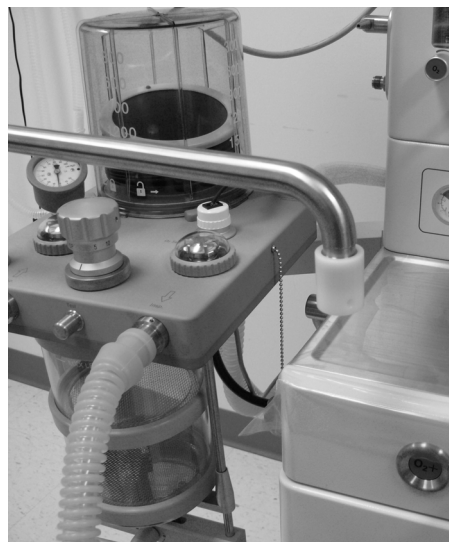
FIGURE 5-3 Blocking the Bag Port
