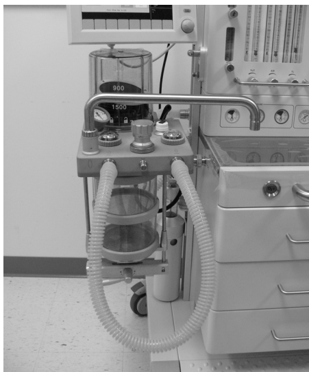
FIGURE 5-2 Connecting the Respiration Tube
