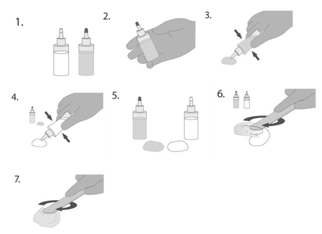
Mix the components on a piece of scrap paper. Use a scrap piece of metal or wood to mix the two liquids. Read the package for specific mixing instructions. Mix the two liquids thoroughly.
