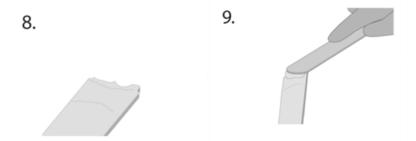
Gently push the two broken ends of plastic together. Hold until the glue is firm. Avoid gluing your glove or skin to the plastic. Wait at least 24 hours to use the part.
