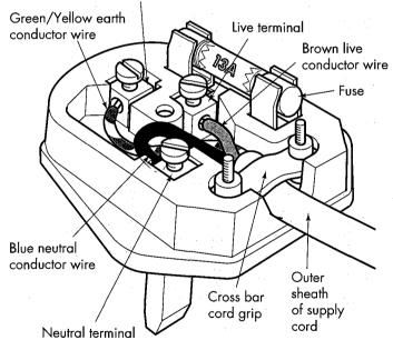
Figure 6: How to wire a plug
