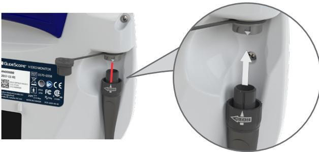
3. To disconnect the video cable from the monitor, rotate the connector ring in the direction of the release arrow, and then remove the connector from the port.
