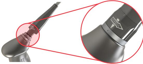
2. To disconnect the scope from the video cable, hold the scope in one hand, twist the cable's locking collar in the direction specified by the arrow on the collar, and then pull. The scope disconnects from the cable.
