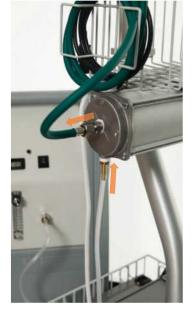
facing the machine): a hose barb inlet threaded fitting outlet to be connected to the CCV's DISS port via the provided hose. When not in use, both ports should be plugged, the inlet by leaving the provided flexible silicone hose attached for quick access, and the outlet by the provided red plastic cap. Keeping the ports plugged will prevent any cleaning fluid from entering the reservoir, which would then pose a danger to the patient as fumes or vapors could be inhaled.
