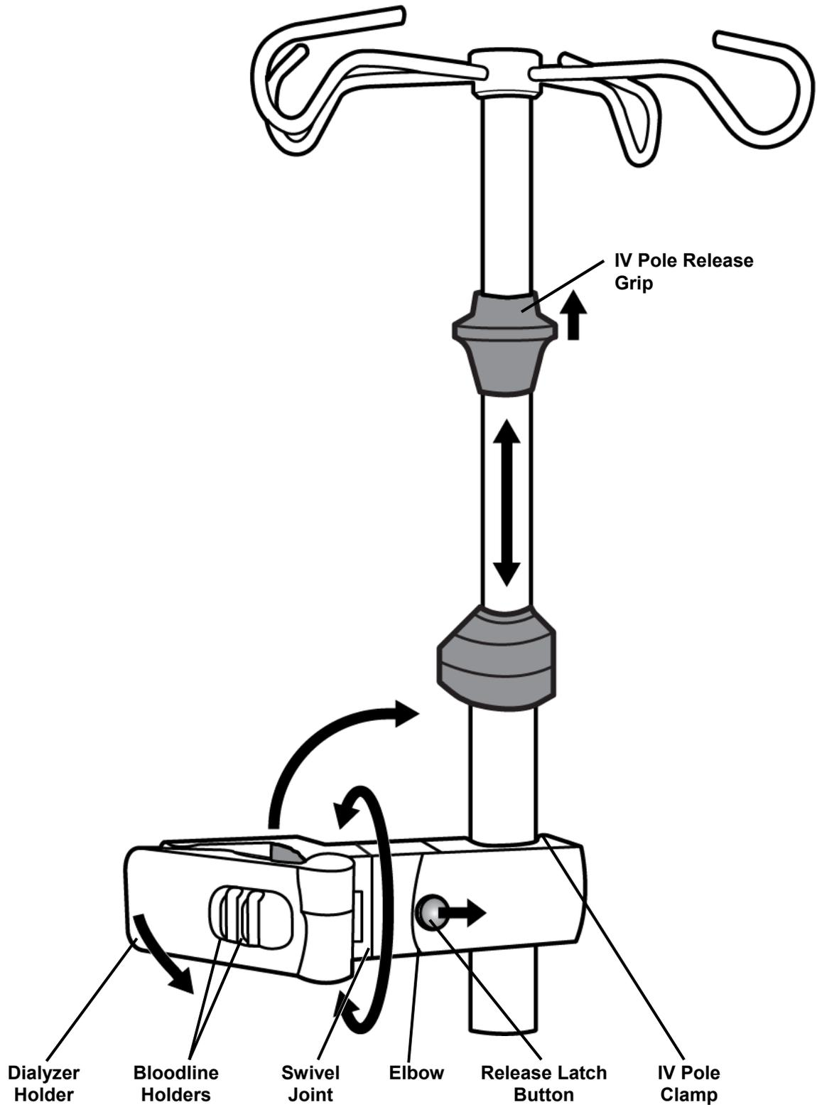
Figure 16 – The IV Pole and Dialyzer Holder
