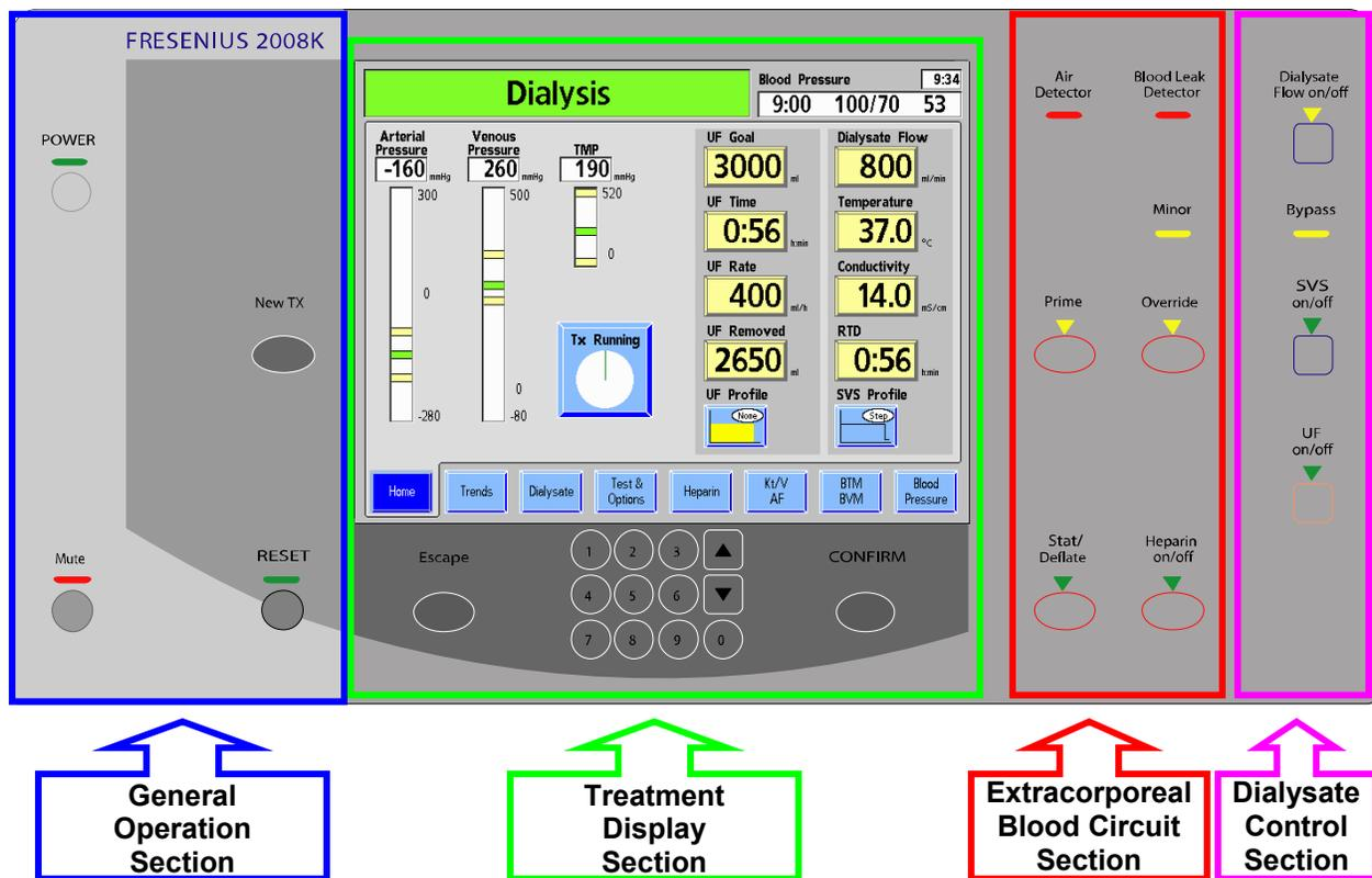
Figure 3 – The Components of the Control Panel
