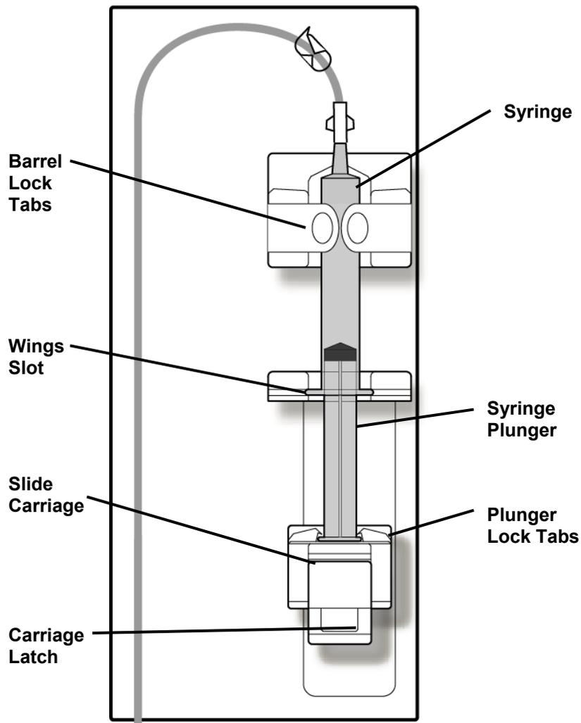
**Figure 42 – The 2008K Heparin Pump Module with Syringe Loaded and Connected**
