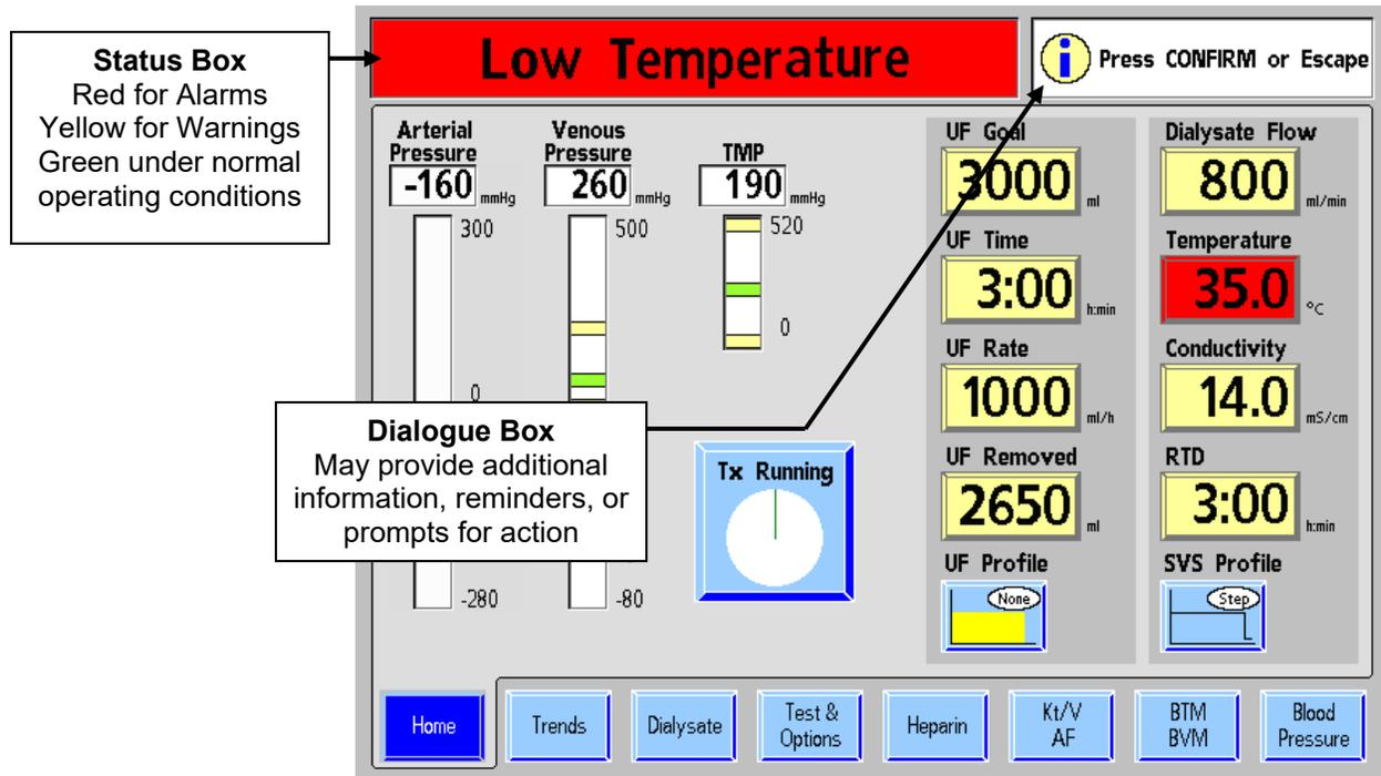
**Figure 63- Status Box and Dialogue Box during an Alarm Event**
