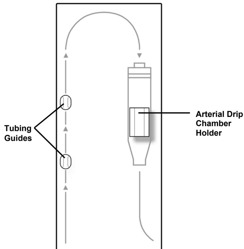
**Figure 9 – The Arterial Drip Chamber Module**
