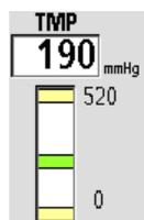
After a time delay for stabilization, the alarm limits are automatically set at  $\pm 60$  mm Hg for conventional dialyzers, and  $\pm 40$  mm Hg for high flux dialyzers. The alarm window automatically adapts for gradual increases in TMP caused by increasing blood viscosity resulting from ultrafiltration.
