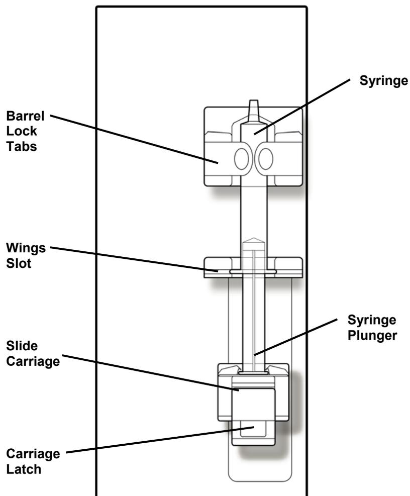
Figure 11 – The Heparin Pump Module (shown with syringe)
