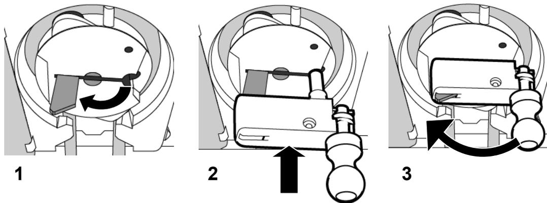
**Figure 55 – Inserting the Blood Pump Crank**
