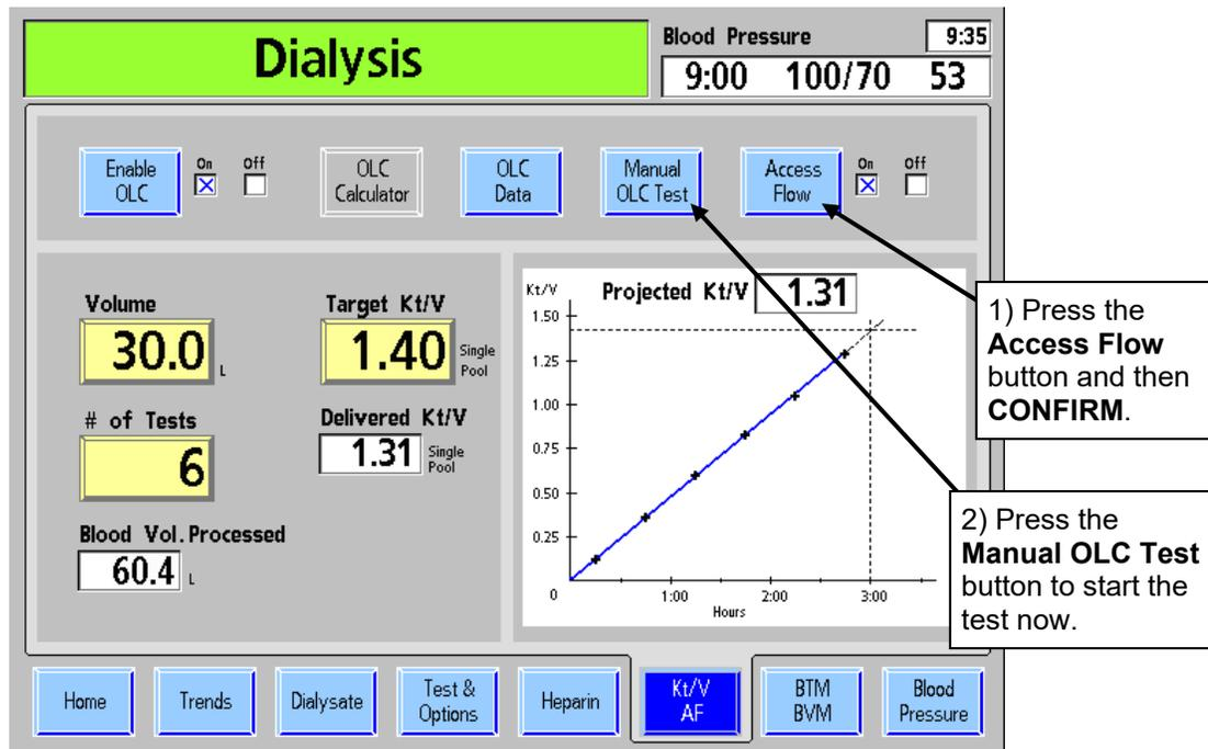
**Figure 50 – Starting an Access Flow Test**
