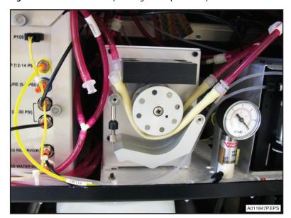
Figure 6.10 Peristaltic Pump Tubing with Open Clamp
