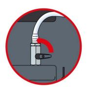
▶ Open the drain cock by turning it anticlockwise (90°). Allow the heat transfer liquid to drain off.
