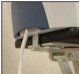
1. To secure the traction unit to the traction stand, loosen the clamp from the traction unit. Fit the traction unit to the stand and tighten the clamp up onto the stand.
