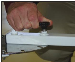
Position the adjustment knob of the Traction Unit Stand to the desired degree of the Pivot Plate.
