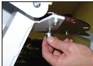
Attach the two supplied 9/16" ESNA nut and tighten with a 9/16" wrench.
