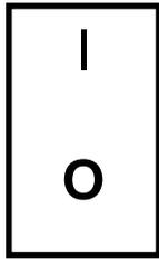
**Supply mains On/Off** isolating switch
