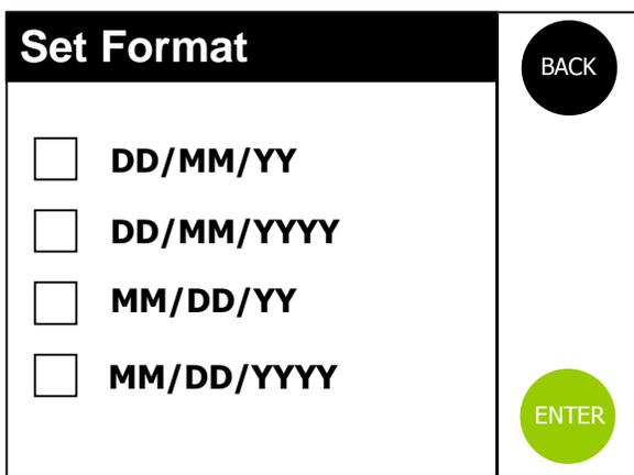
**Should the format of the date be wrong, by selecting the “Set Format” menu and by pressing “ENTER”** the “**Set Format**” menu will be displayed. Touch the box that matches the correct format. A tick will appear to confirm your selection. Press “**ENTER**” a confirmation screen will pop up and after a few seconds the screen will revert back to the “**Time Date Menu**”
