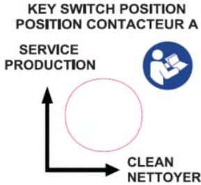
For safety a key is provided to operate the unit and prevent the unit accidentally being placed into a clean. This label identifies the position of the key. When approved/trained to do so always refer to the "**Chemical cleaning and heat disinfection instructions**" if unsure about when and how to use this key.
