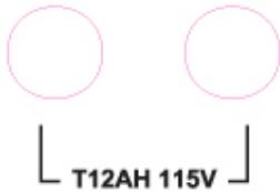
**This label identifies the position of the unit's two external fuses. UNDER NO CIRCUMSTANCES** try to remove or replace these fuses, always refer to your Healthcare provider. Refer to **Section 11.1.2** for Fuse details
