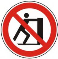
**No Pushing:** The unit has been designed as a stationary device during normal operation. Do not push the unit when in operation as this may cause the integral tilt detector to shut the unit down.
