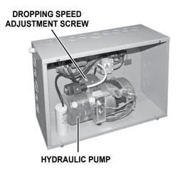
boom hydraulic pump adjustments
