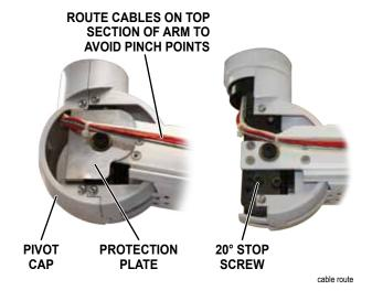
Figure 5-30. AFC Arm Limit Stops
