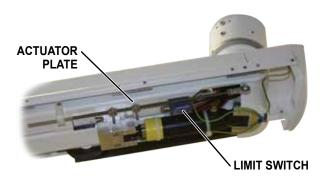
Figure 5-9. Up Limit Switch Adjustment
