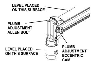
Figure 5-32. Eccentric Cam Adjuster
