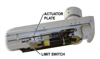
Figure 5-10. Down Limit Switch Adjustment
