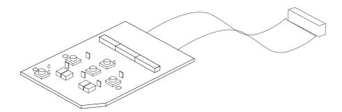
All the push-buttons are mounted on the CPU board together with the LEDs and the three bar-graphs for pressure display. Also mounted here is the four 7-segment displays for the rise time and backup rate displays (PV 102+).
