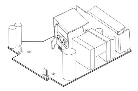
The power supply unit is fed primarily with mains power via the mains power inlet to the internal AC/DC converter. Secondly, the power board can be fed with 12–24 DC via the external battery input.
