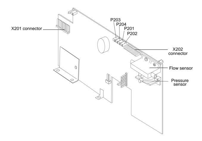
The MDA (motor drive assembly) board comprises the driver stage for the blower motor, the pressure sensor, the flow sensor, the hour counter and the D-shell connector for serial communication.
