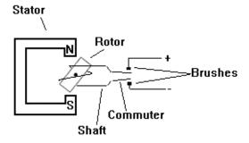
In general, the engineer in the field will not be called upon to rebuild an electrical motor. Almost every major city in the developing world has a shop that can accomplish this task. However, most motors use carbon brushes to make electrical contact with the electro-magnets on the
