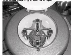
The simplest centrifuges have a single speed motor, a mechanical timer and a rotor that holds the samples at a preset angle of 20 to 40 degrees. For user safety, the lid of the centrifuge should have an interlock on it so that the unit will not spin with the lid in the up position.
