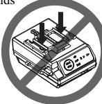
Do not manipulate the pump rocker with your finger—it can damage the mechanism.
