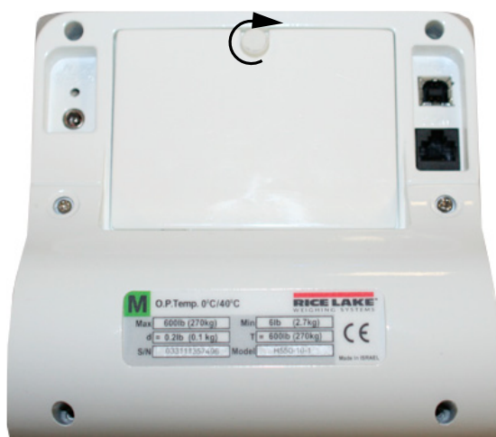
Figure 2-3. Secure Battery Cover Panel
