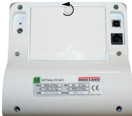
Figure 2-1. Uninstall Battery Cover Panel
