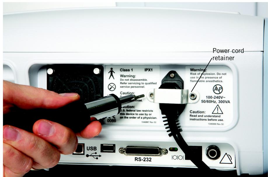
Figure A-4: Installing the power cord retainer
