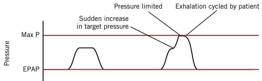
Figure 6-2: PPV waveform – Max P limit
