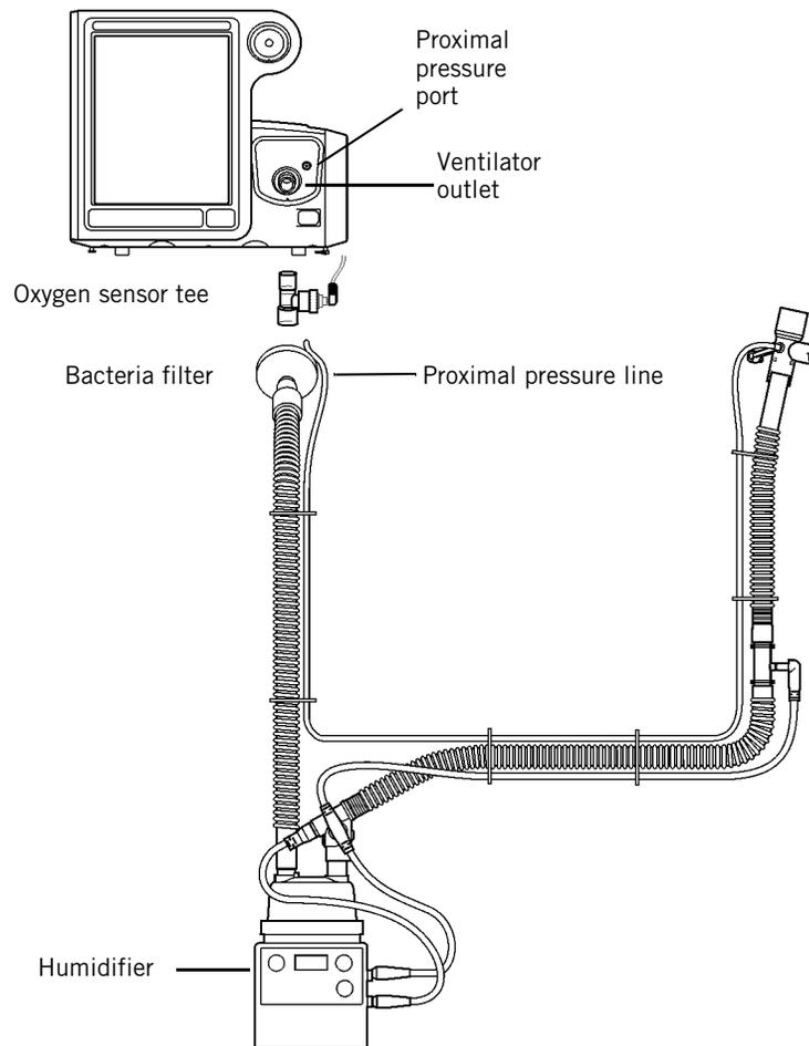
*Figure 5-1: Noninvasive patient circuit, with heated-wire and humidification*
