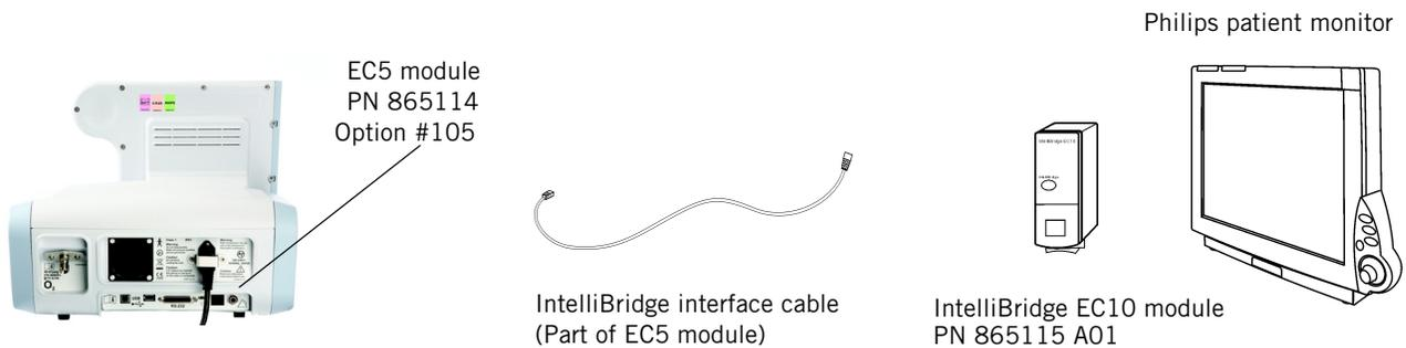
Figure B-3: Connect via IntelliBridge to a Philips patient monitor
