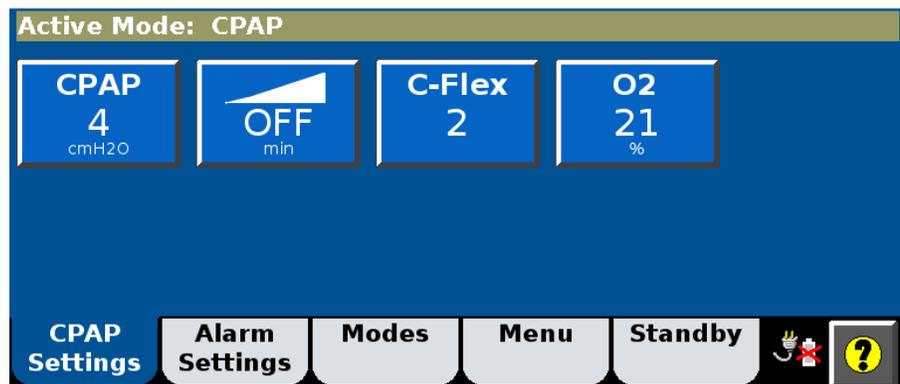
Figure 4-6: CPAP controls
