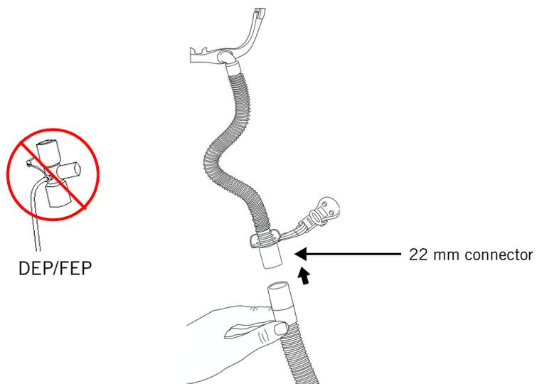
Figure 7-2: High flow nasal cannula, 22 mm connection
