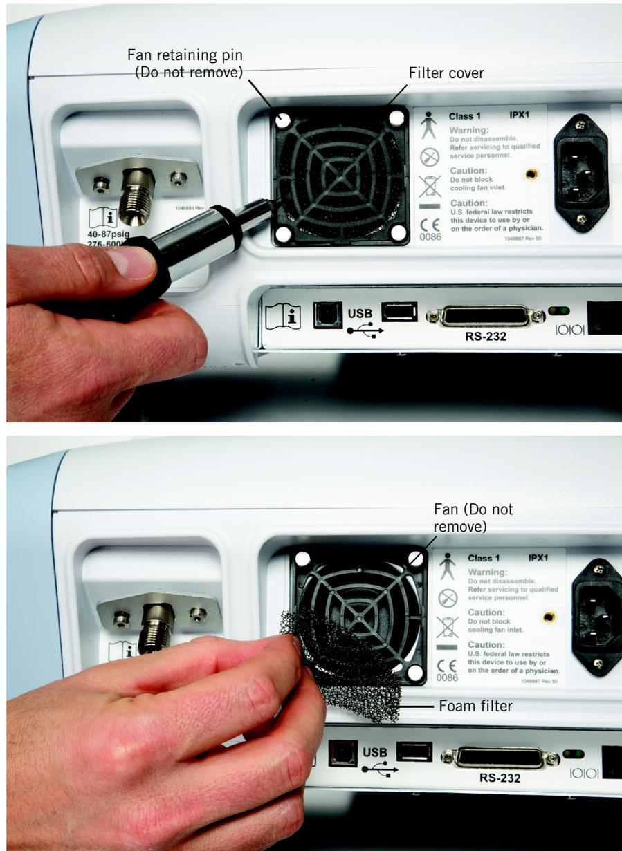
Figure 10-2: Replacing the cooling fan filter
