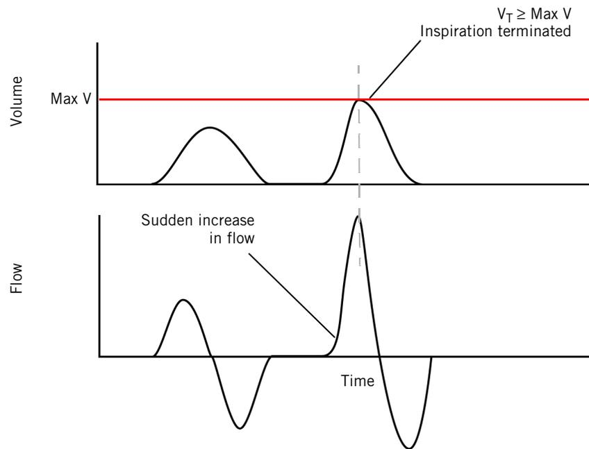
Figure 6-1: PPV waveform – Max V limit
