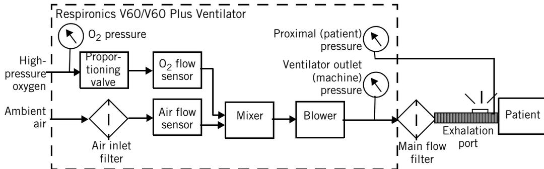
Figure 4-1: Respironics V60/V60 Plus Ventilator gas delivery system
