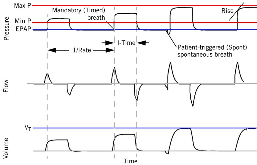
Figure 4-13: AVAPS waveforms
