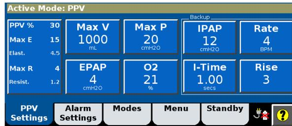
Figure 4-14: PPV controls
