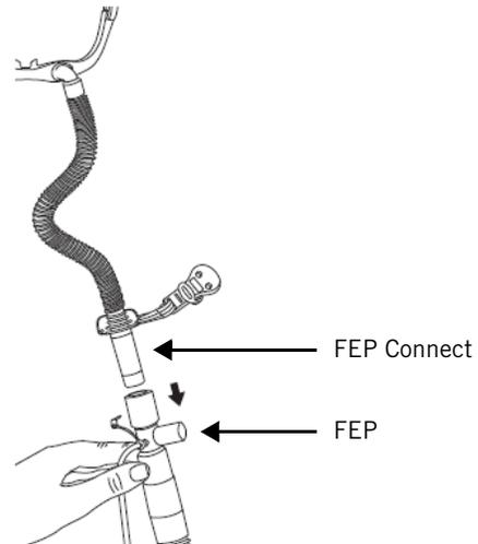
Figure 7-1: High flow nasal cannula using the FEP Connect
