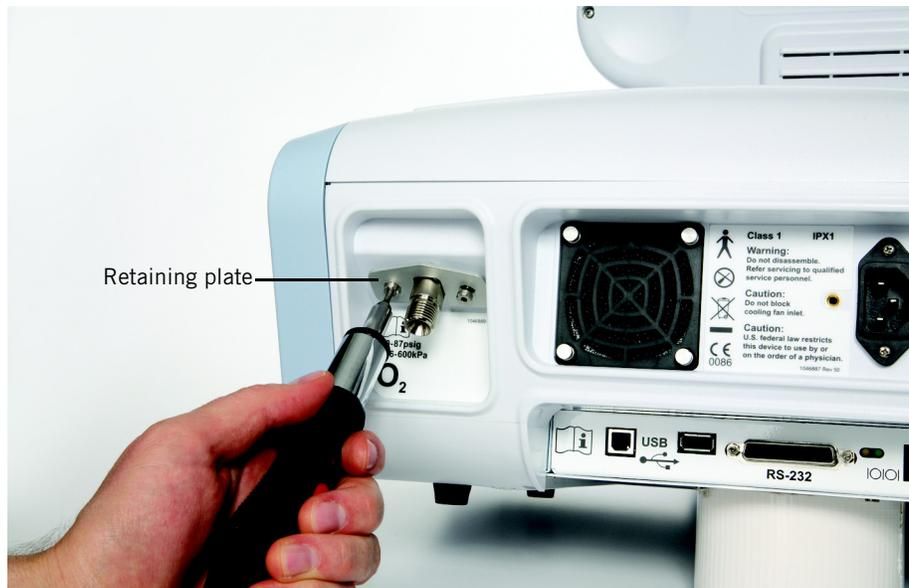
Figure A-3: Installing the oxygen inlet connector
