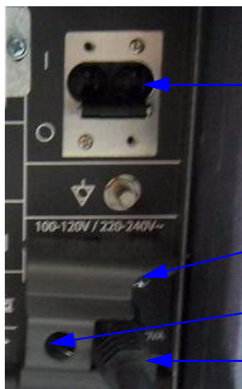
Figure 4-1 Circuit Breaker, pull-out protection and main power cable at rear of system
