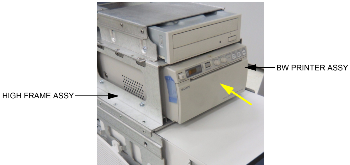
Figure 8-186 Insert BW PRINTER ASSY to HIGH FRAME ASSY
