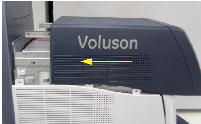
Figure 8-229 Place MID CABINET on MID FRAME and Moving toward BACKBONE
