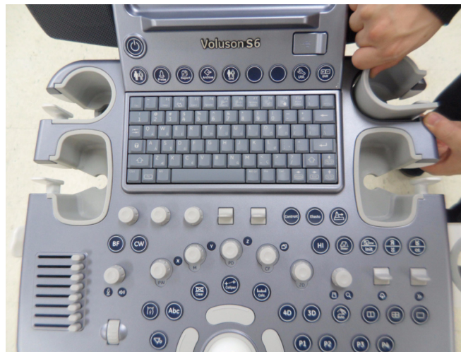
Figure 8-74 Removing the 4 PROBE HOLDERS
