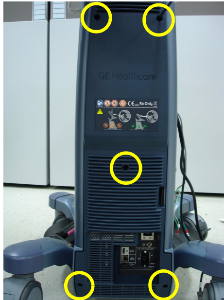
Figure 8-178 Unscrew 5 screws and remove REAR COVER POLARIS ASSY
