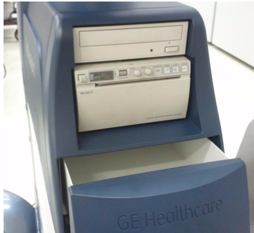
Figure 8-231 DRAWER Assembly for HIGH CABINET Option
