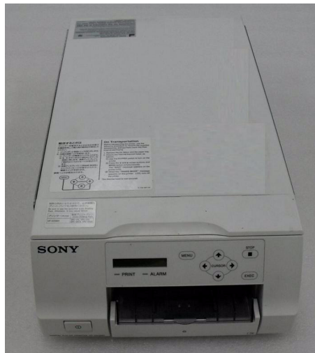
Figure 8-189 Fix COLOR PRINTER to COLOR PRINTER BRKT POLARIS with 6 screws (2306562, FH M3X6)
