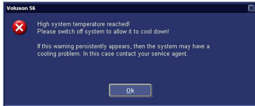
Figure 7-43 A second high system temperature message
