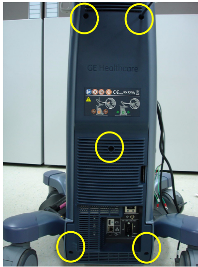
Figure 8-52 Unscrewing 5 screws and Remove REAR COVER ASSY
