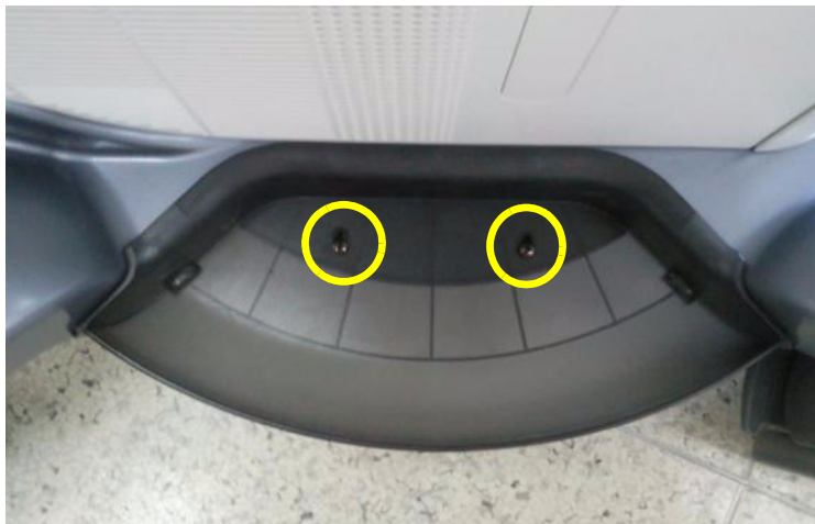
Figure 8-113 Unscrewing 2 screws and remove SIDE TRAY ASSY
