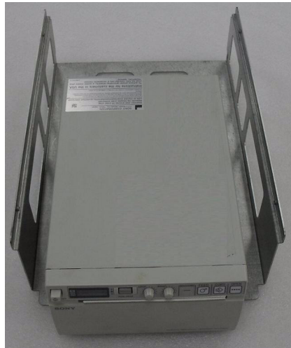
Figure 8-175 Fix BW PRINTER to COLOR PRINTER BRKT POLARIS with 4 screws (2306562, FH M3X6)
