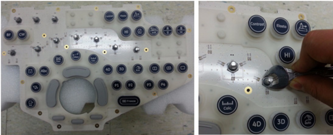
Figure 8-85 Unscrewing the nut of encoder and replace the encoder
