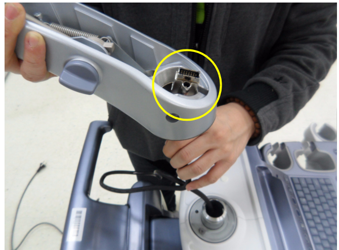
Figure 8-34 Removing the MONITOR STAND ARM
