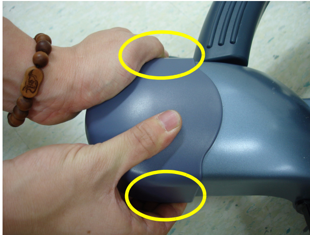
Figure 8-103 Removeing the CASTER CAP
