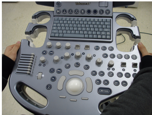
Figure 8-75 Unscrewing 9 screws and lifting up the MAIN OPIO
