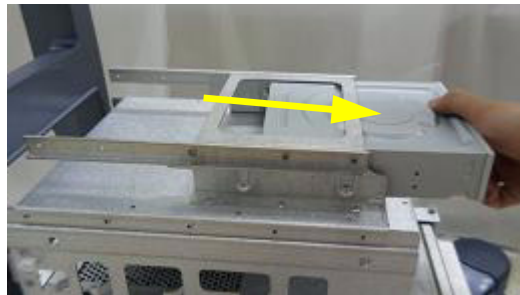
Figure 8-207 Remove DVD from MID FRAME ASSY
