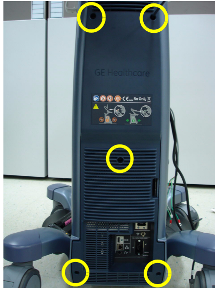
Figure 8-115 Unscrewing 5 screws and remove REAR COVER ASSY
