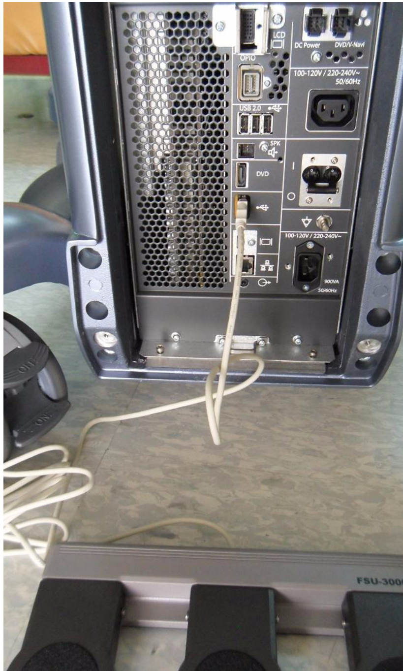
Figure 3-10 Connection Scheme - Footswitch
