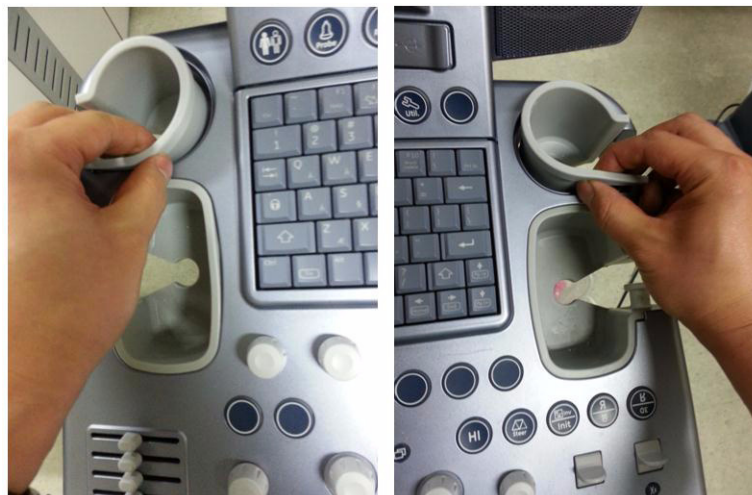
Figure 8-80 Removing 4 probe holders
