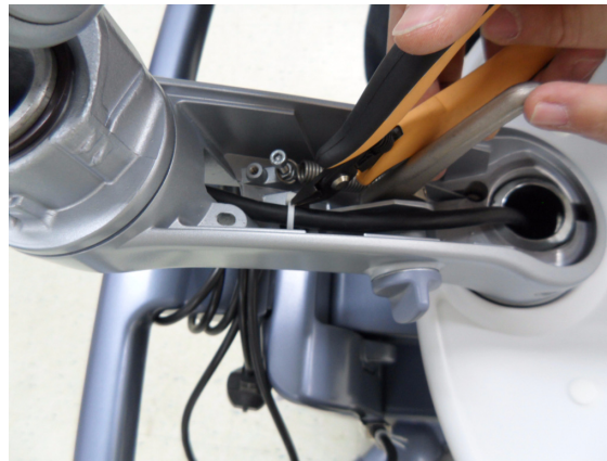
Figure 8-31 Removing Cable Tie
