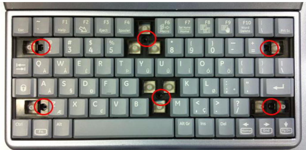
Figure 8-163 Tighten the 6 screws
