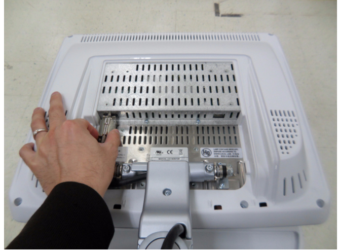
Figure 8-24 Disconnecting MAIN PANEL LONG CABLE
