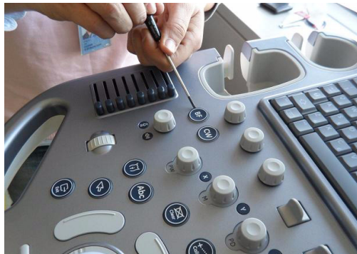
Figure 8-173 Push against the circle cap and lift it
