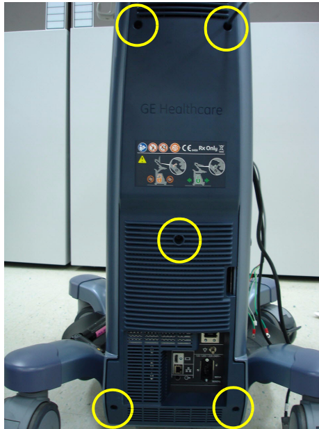
Figure 8-209 Unscrew 5 screws and remove REAR COVER POLARIS ASSY
