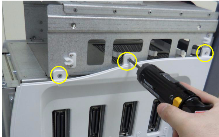
Figure 8-201 Unscrew 3 screws to remove SIDE COVER R ASSY
