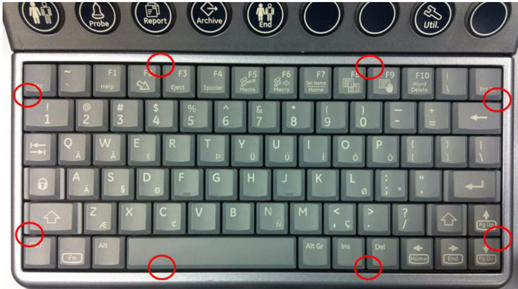
Figure 8-162 Push the AN key Top Assy
