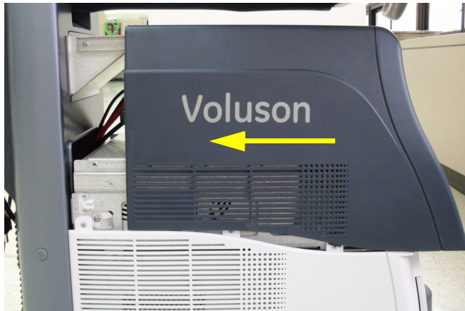
Figure 8-188 Assemble HIGH CABINET ASSY
