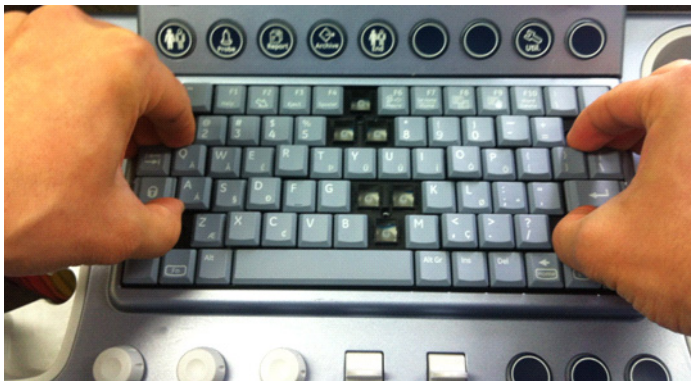
Figure 8-161 Pull out AN Key Top Assy
