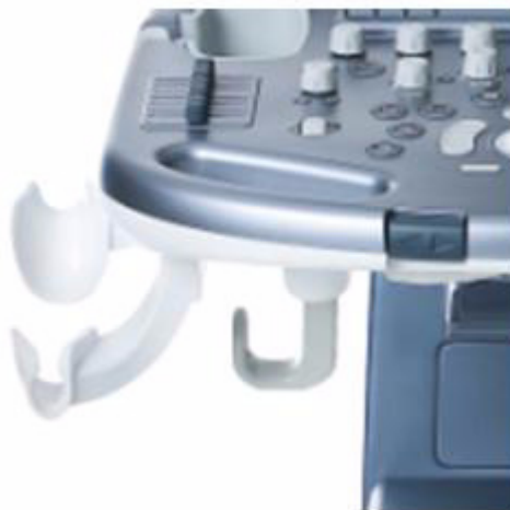
Figure 8-233 HORIZONTAL TV PROBE HOLDER is installed on Left Side only
