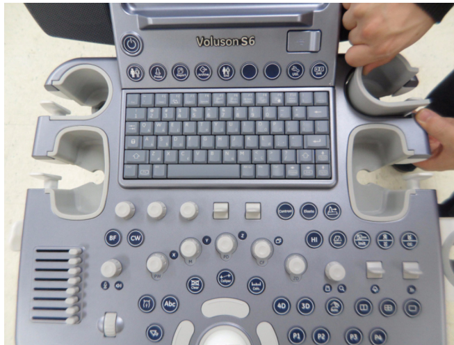
Figure 8-36 Removing the 4 PROBE HOLDERS
