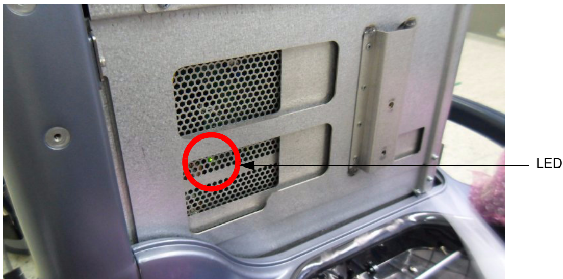
Figure 7-6 Check green LED inside CPS
