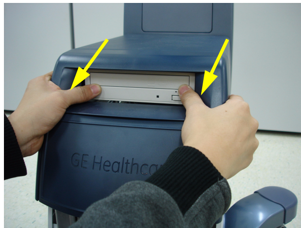
Figure 8-150 Removing FRONT PLASTIC COVER
