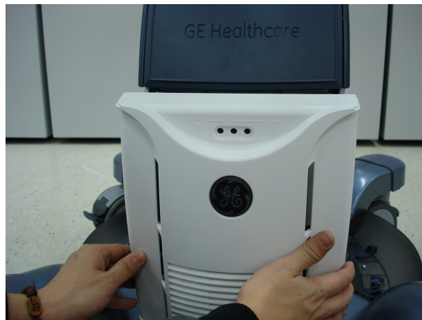
Figure 8-64 Removing the FRONT COVER ASSY
