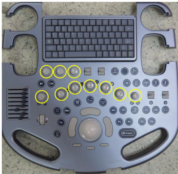
Figure 8-91 Pulling 10 encoder key caps out
