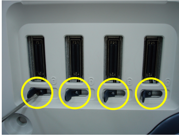
Figure 8-60 Removing the 4 RS KNOBS
