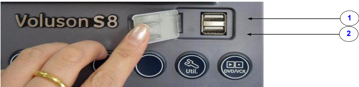
Figure 3-62 External I/O Connectors - on TOP OPIO
