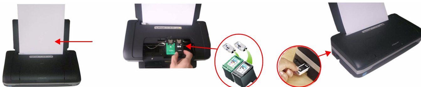
Figure 3-30 Connection of Bluetooth Printer Adapter (HP Officejet H470)
