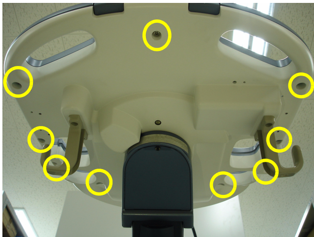
Figure 8-75 Unscrewing 9 screws and lifting up the MAIN OPIO
