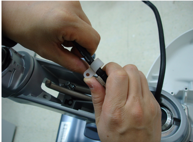
Figure 8-43 Removing the CABLE CLAMP
