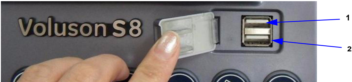
Figure 5-16 External I/O Connectors - on the TOP OPIO
