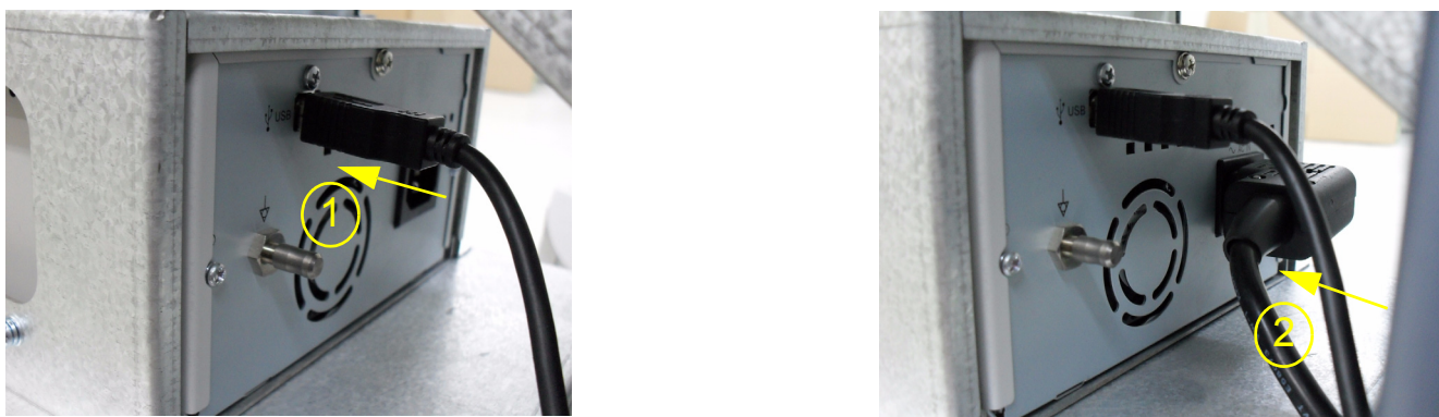
Figure 8-180 Connect BW PRINTER CABLE
