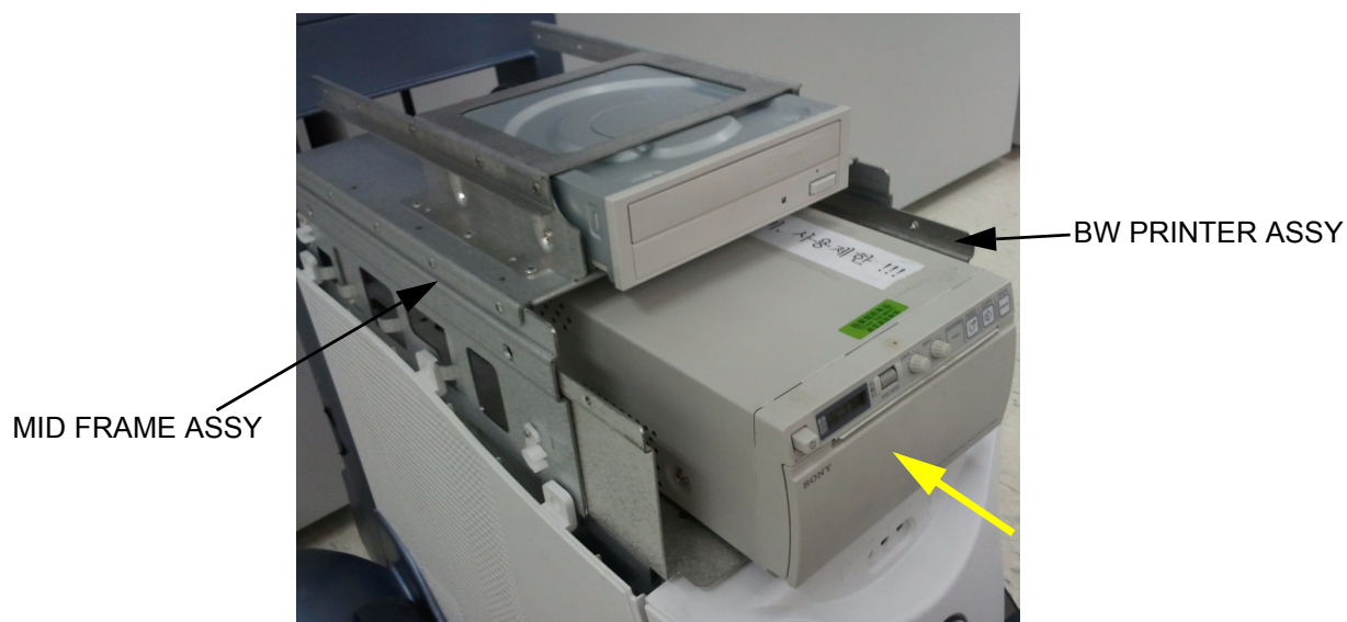
Figure 8-176 Insert BW PRINTER ASSY to MID FRAME ASSY
