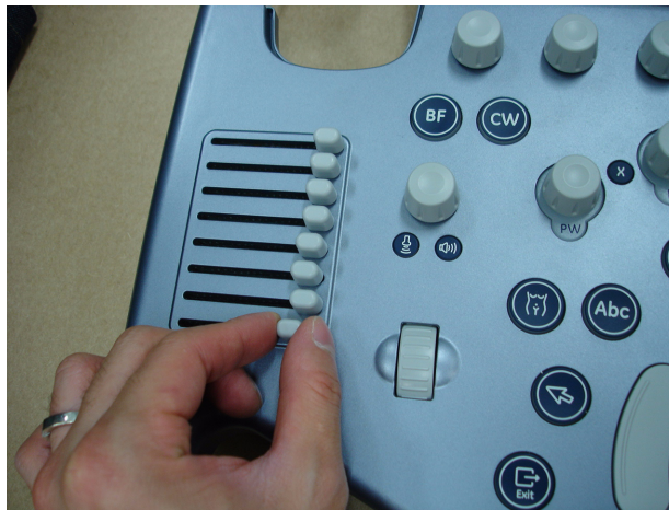
Figure 8-96 Removing 8 TGC KNOBS
