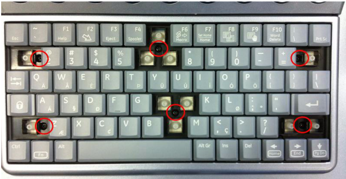
Figure 8-160 Loosen the 6 screws
