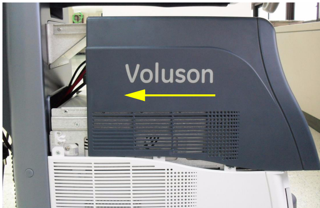
Figure 8-197 Assemble HIGH CABINET ASSY
