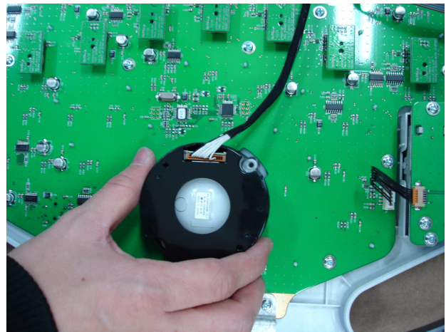
Figure 8-78 Unscrewing 2 screws and pulling out the TRACKBALL
