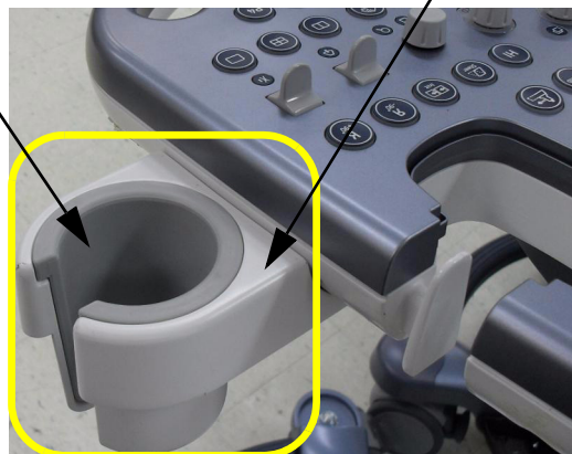
Figure 8-235 Insert TV PROBE HOLDER RUBBER to PROBE HOLDER BASE
