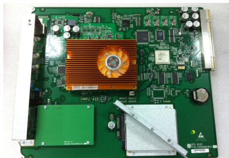
Figure 8-129 FAN power cable connection on the RFS, 5364098-2 or higher
