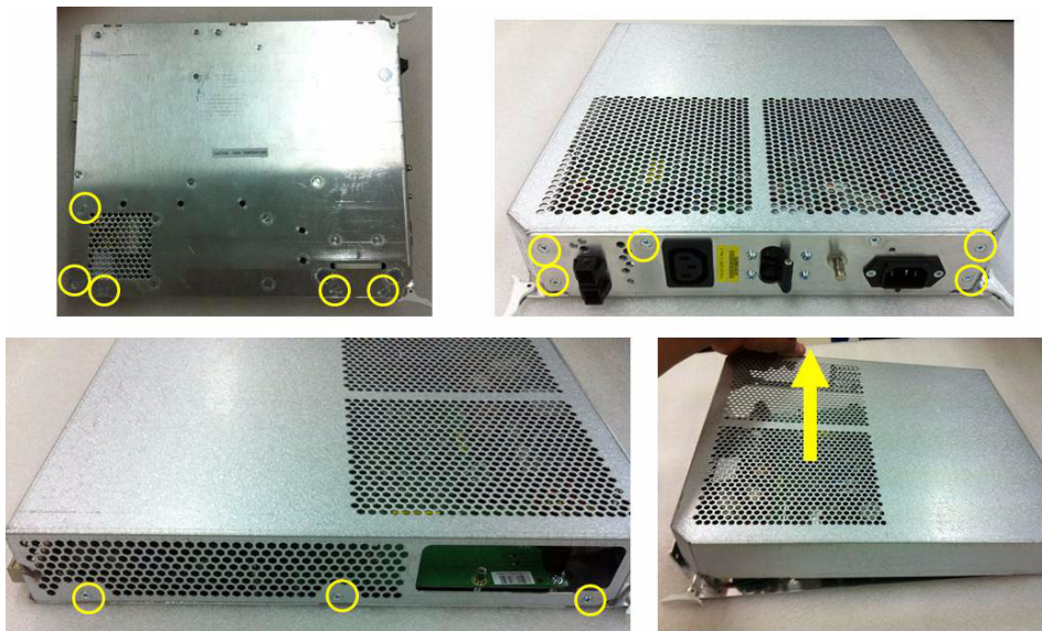
Figure 8-237 Remove CPS2 with Battery cover
