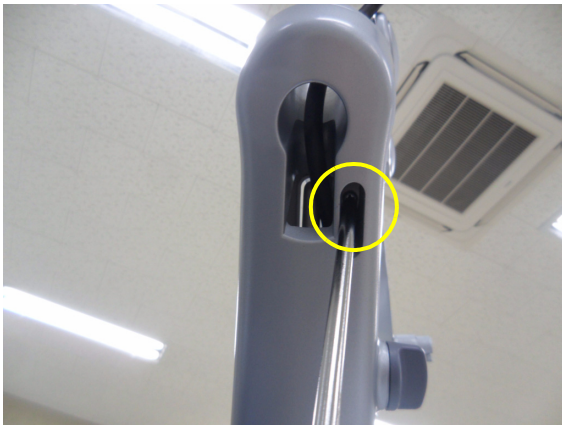
Figure 8-30 Unscrewing 1 screw and removing 1ST ARM COVER
