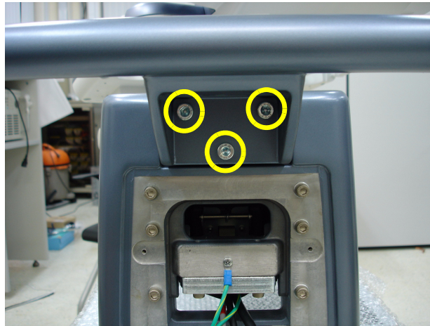
Figure 8-116 Unscrewing 3 screws and remove REAR HANDLE
