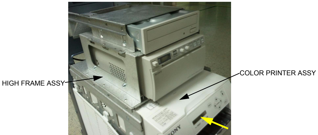
Figure 8-195 Insert COLOR PRINTER ASSY to HIGH FRAME ASSY
