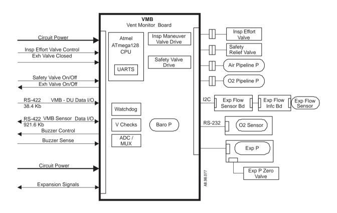
For further details, refer to Figure 11-8, "VMB block diagram" in Section 11.
