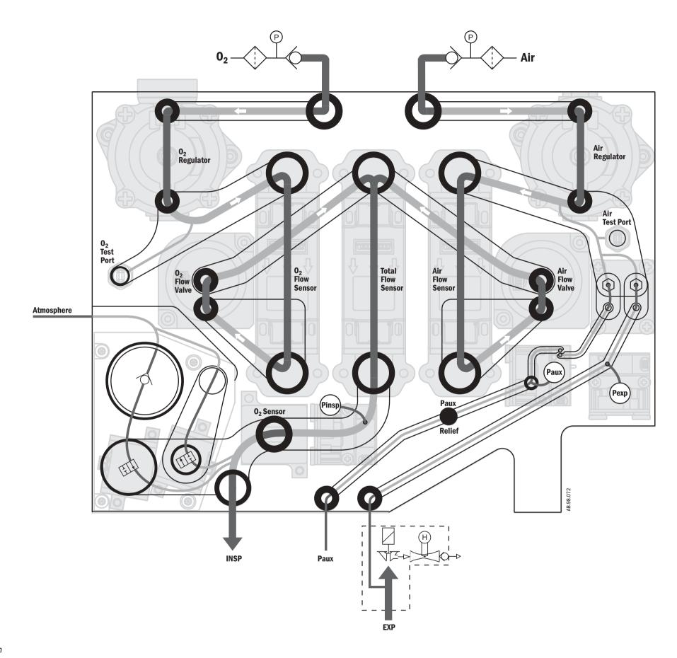
Figure 11-2 • Vent Engine manifold flow diagram
