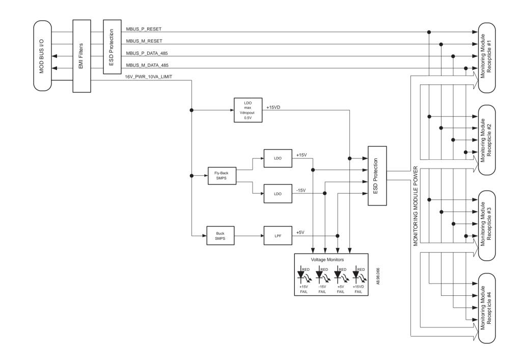
Figure 11-10 • Monitoring Module Rack block diagram
