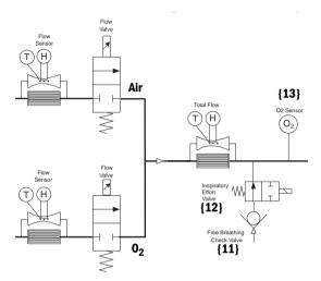
Next in the flow path is the  $O_2$  sensor {13}. The sensor is used to monitor the  $O_2$  concentration produced by the combined  $O_2$  and Air flows.
