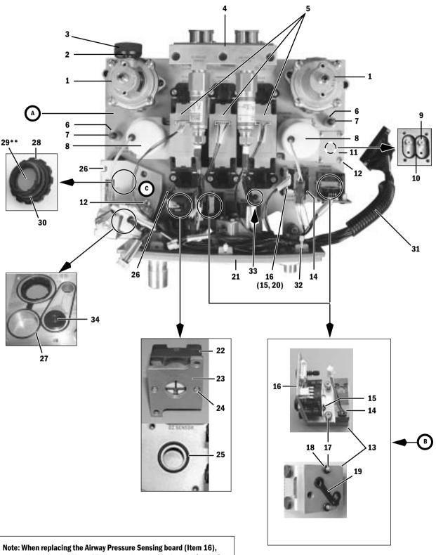
Note: When replacing the Airway Pressure Sensing board (Item 16), ensure that the o-ring (Item 15) is properly seated in the manifold before mounting the board in place.
