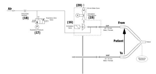
Immediately upstream of the exhalation valve is a tap for the expiratory pressure transducer {17} and its associated zeroing valve. The expiratory pressure tap is continuously purged with 35 ml/min of air to ensure that exhaled condensate does not occlude the tap. The air flow is established from the regulated Air supply using a fixed orifice (pneumatic resistor) {18}.
