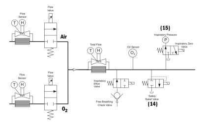
The inspiratory airway pressure transducer {15}, along with its associated zeroing valve, is located just prior to the inspiratory outlet port. This transducer has a range of -20 to  $120 \text{ cm H}_20$  and serves as one of three airway pressure measuring devices in the EV.
