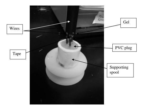
10.. Slide the heat shrink on the end of each wire. Solder the wires to the conductors embedded in the new connector plug in the appropriate positions as determined in step 7. Shrink the heat shrink tubing, using the BTA skill *Electrical-Connections-HeatShrinkTubing*.
