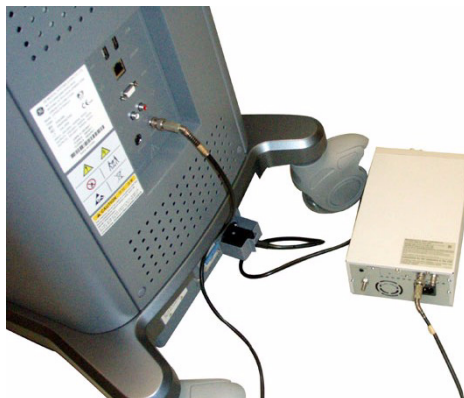
Figure 3-11 Connect B/W Printer (Sony UP-897MD) to the system
