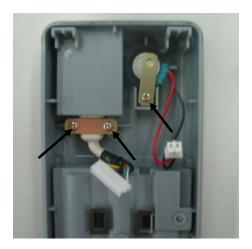
2. Thrust the end of the SpO<sub>2</sub> communication cable socket and push it out.
