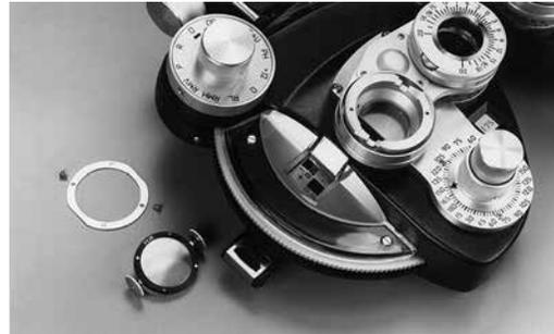
Figure MM-1 Cross Cylinder Lens Assembly
