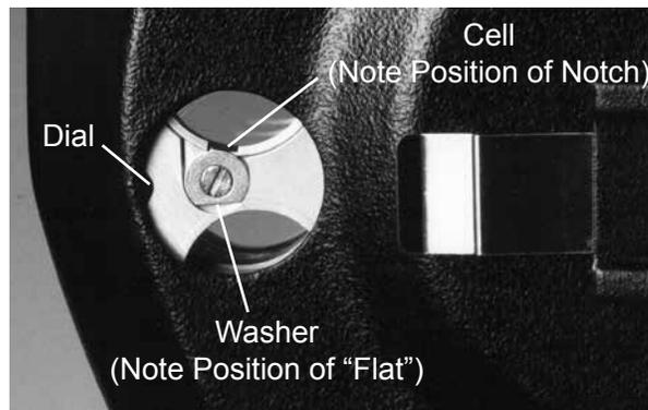
Figure MM-5 Auxiliary Dial - Old Style
