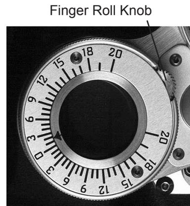
Figure IU-7 Rotary Prism Unit
