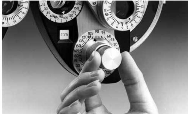
Figure TM-5 Turning Cylinder Power Knob
