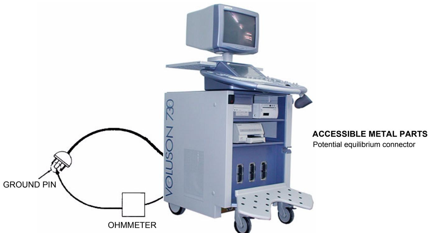
**Figure 10-2 Ground Continuity Test**
