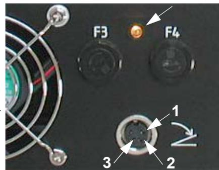
Figure 7-2 Diagnostic LED's and corresponding voltage check points
