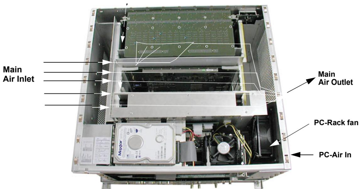
Figure 5-34 Air Flow Control
