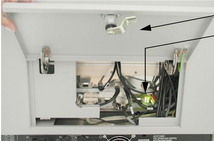
Open the locking, flap the service lid on the back of the Voluson® 730Expert upwards, and check the status of the Diagnostic LED's.
