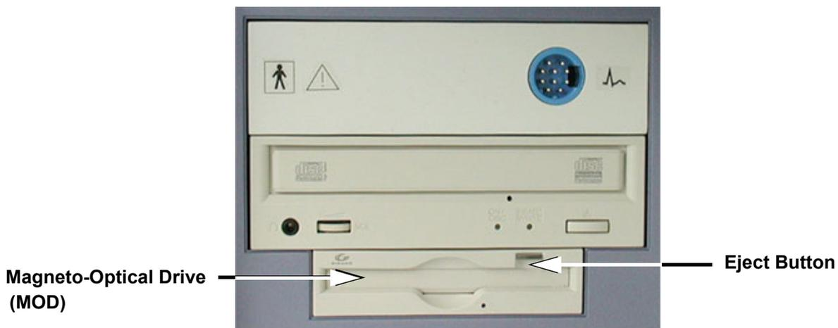
Figure 4-16 Magneto-Optical Drive
