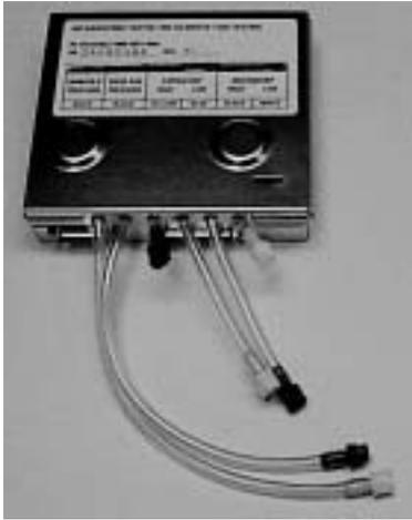
A Sensor Interface Board (SIB) serves as the interface between the ventilator CPU board and the breathing circuit sensors.
