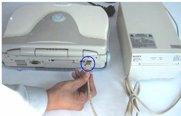
**Figure 3-15 Connect B/W printer to the system**
