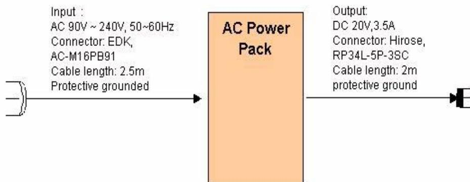
**Figure 5-71 AC Power Distribution Block Diagram**
