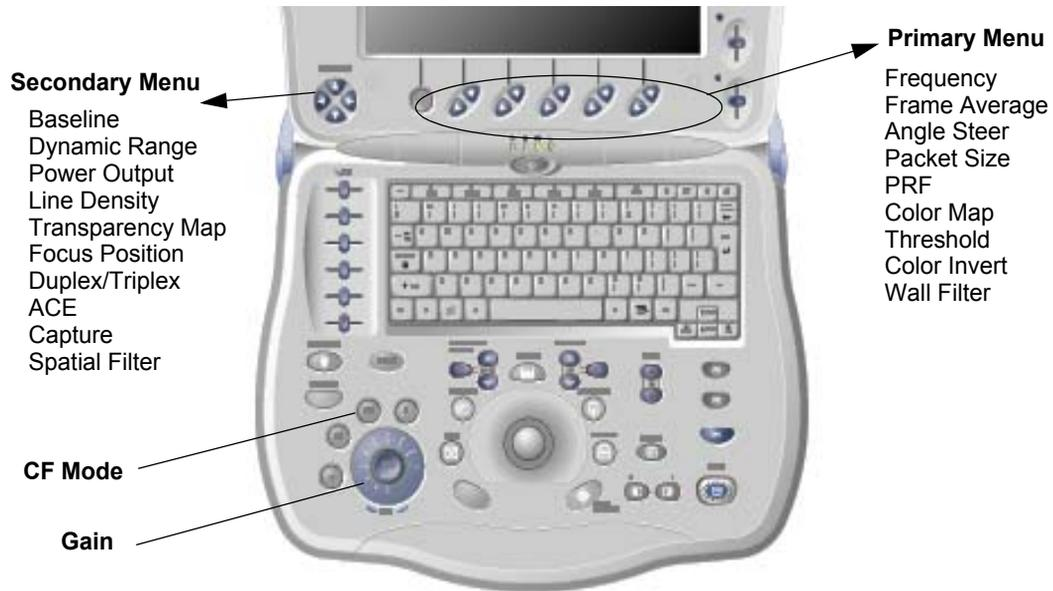
Figure 4-49 Controls available in Color Flow Mode
