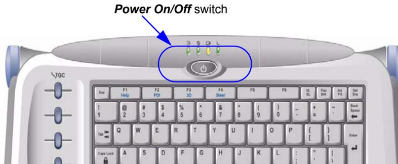
Figure 4-37 Power On/Off Switch
