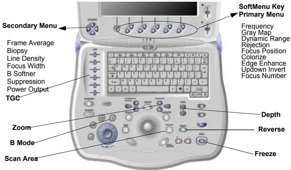
Figure 4-45 Controls available in B Mode
