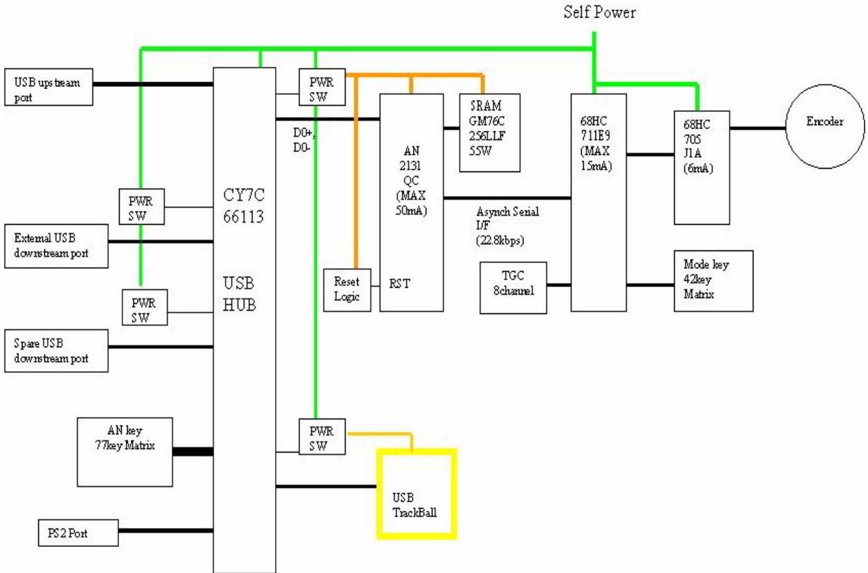
Figure 5-70 Keyboard Block Diagram
