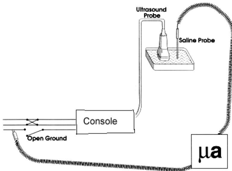
Figure 10-4 No Meter Probe Adapter Procedure
