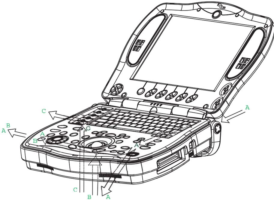
**Figure 5-74 Air Flow Inside the Scanner**
