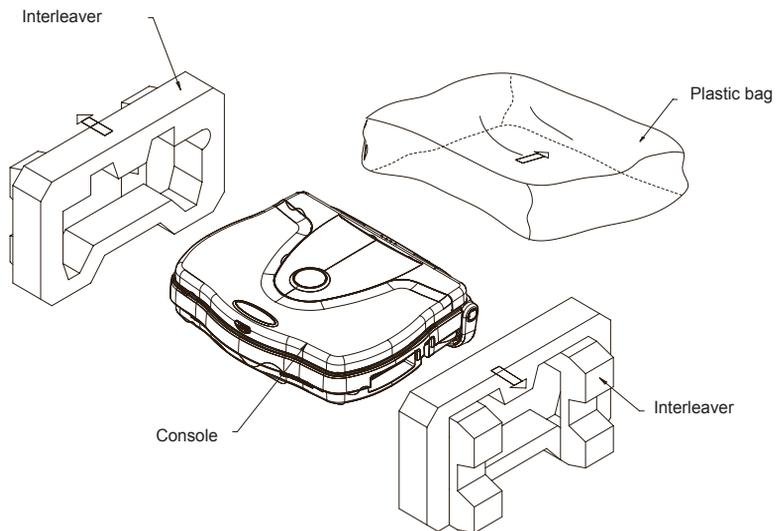
**Figure 3-7 Removing interleavers and plastic bag**
