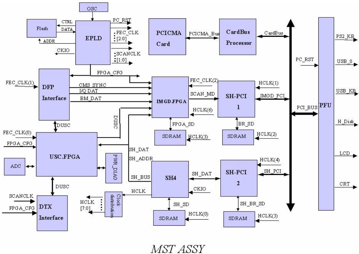
Figure 5-66 MST Block Diagram
