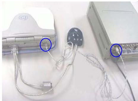
**Figure 3-21 Video Adapter and VCR Connection**
