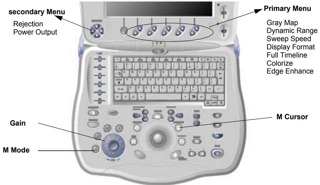
Figure 4-47 Controls available in M Mode
