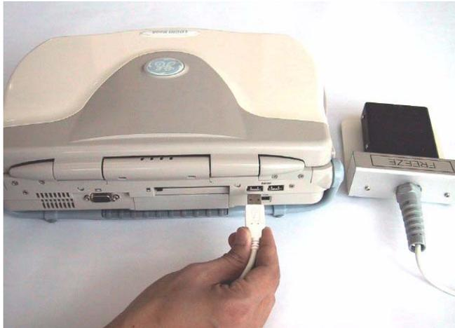
**Figure 3-18 Connect Foot Switch to the system**
