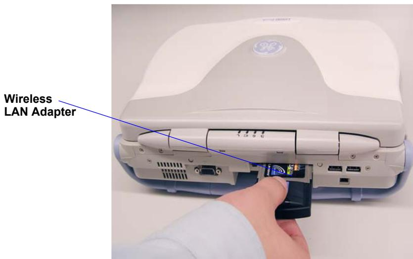
**Figure 3-19 Connect Wireless LAN Adapter to the system**
