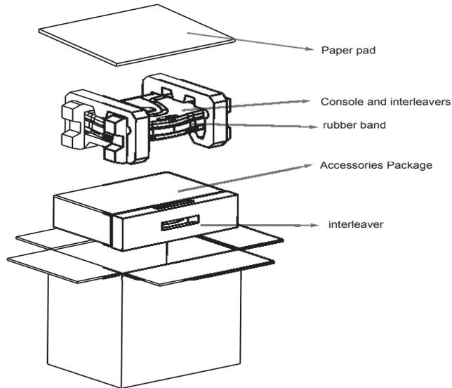
Figure 3-6 Unpacking the equipment
