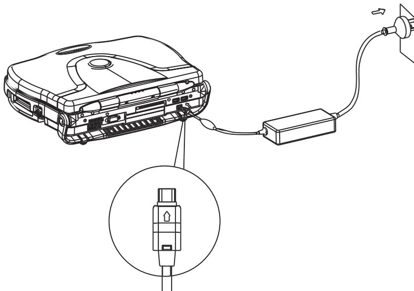
Figure 3-9 connect AC adapter
