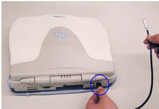
**Figure 3-20 USB Lamp connection**
