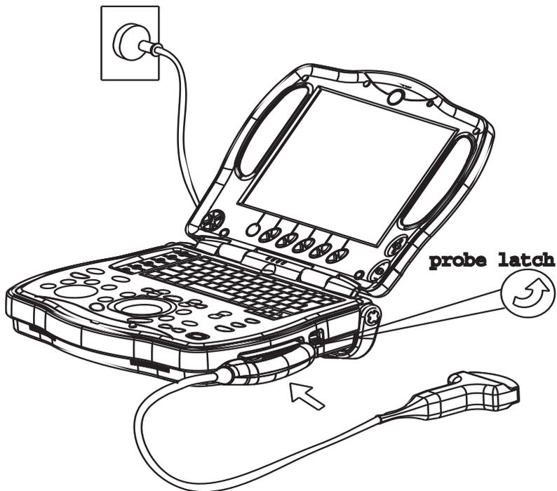
**Figure 3-12 Connect the probe**
