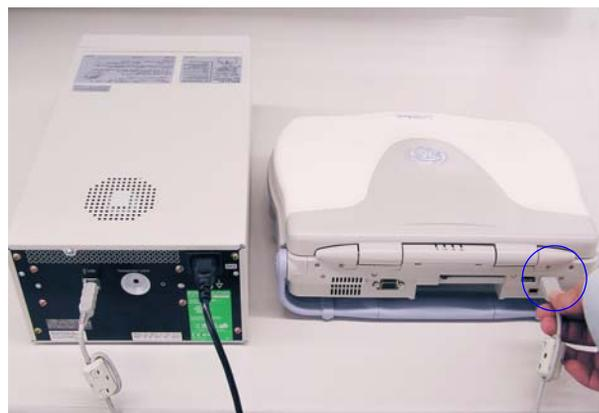
**Figure 3-16 Connect digital color printer to the system**
