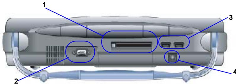
**Figure 3-14 Rear Connector Panel**
