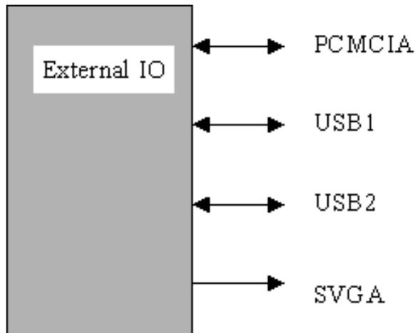
**Figure 5-64 External I/O module overview**
