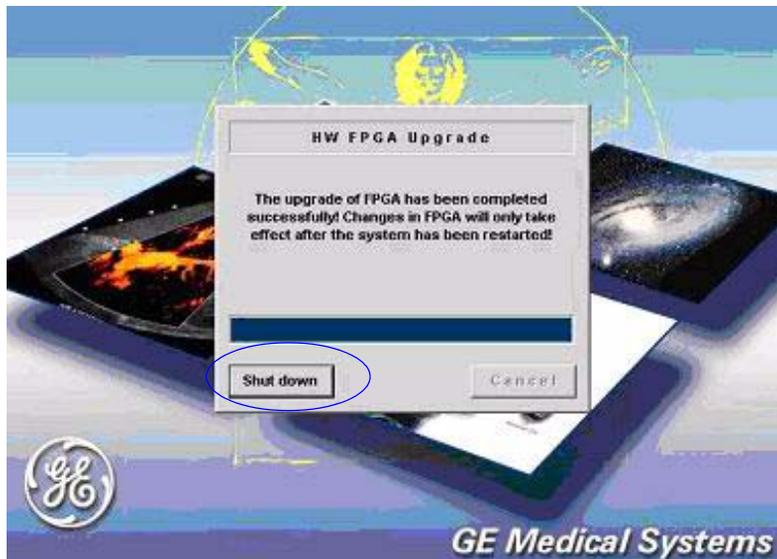
Figure 3-32 FPGA Upgrade
