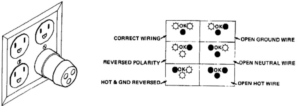
Figure 10-1 Typical Alternate Outlet Tester
