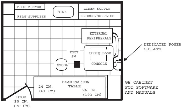
An 8 by 10 foot Minimal Floor Plan
