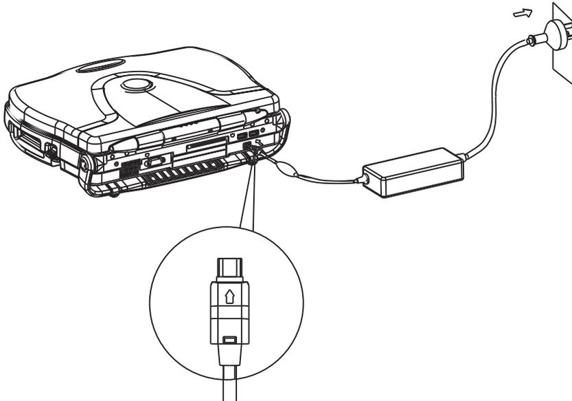
Figure 4-36 connect AC adapter
