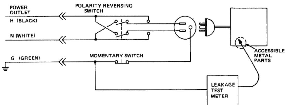
**Figure 10-2 Set Up for Chassis Source Leakage Current, IEC 601-1 Clause 19 - Continuous Leakage Currents and Patient, Auxiliary Currents**
