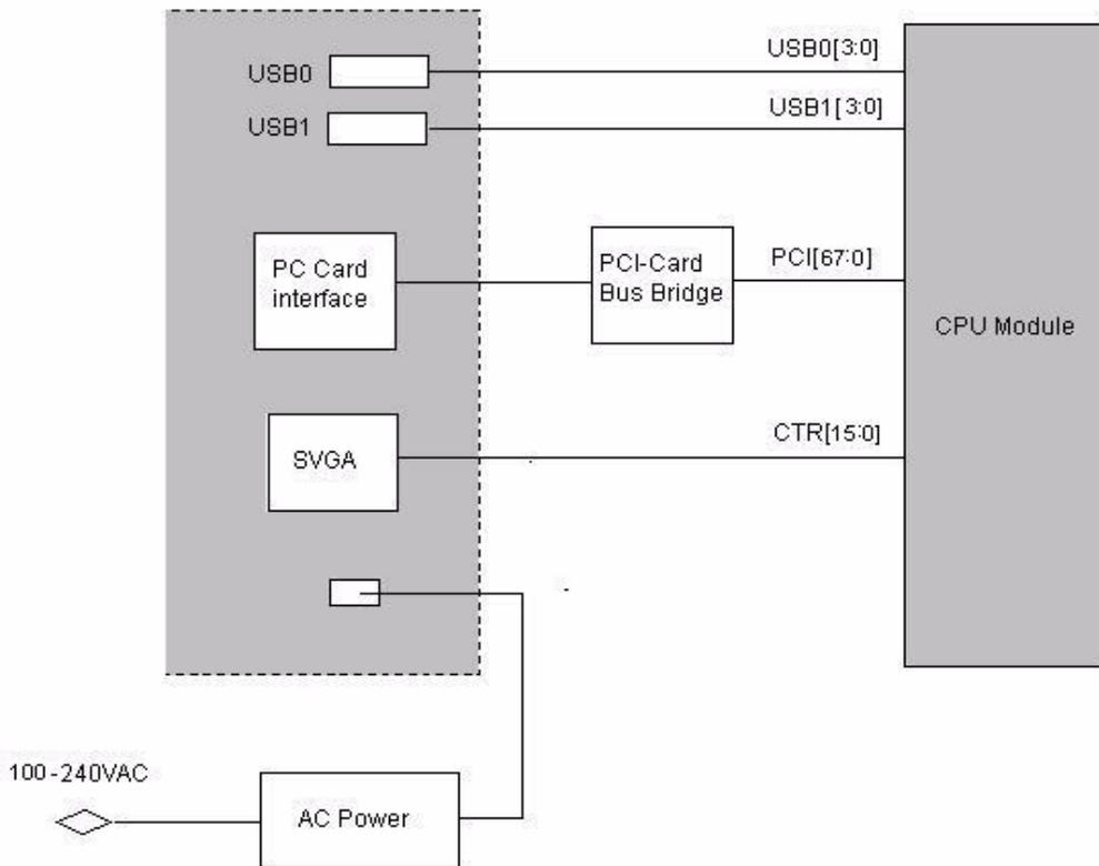
Figure 5-73 Rear Panel Block Diagram
