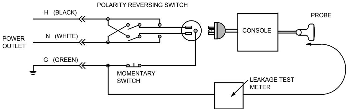
**Figure 10-3 Set Up for Probe Leakage Current**
