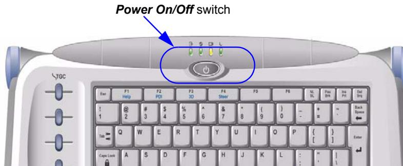
Figure 3-10 Power On/Off Switch
