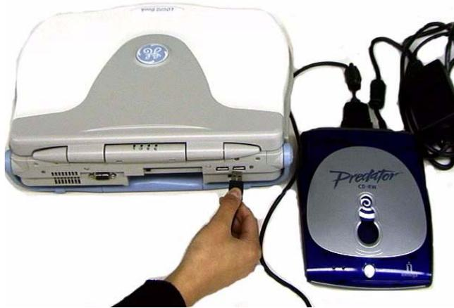
**Figure 3-17 Connect CD-RW to the system**
