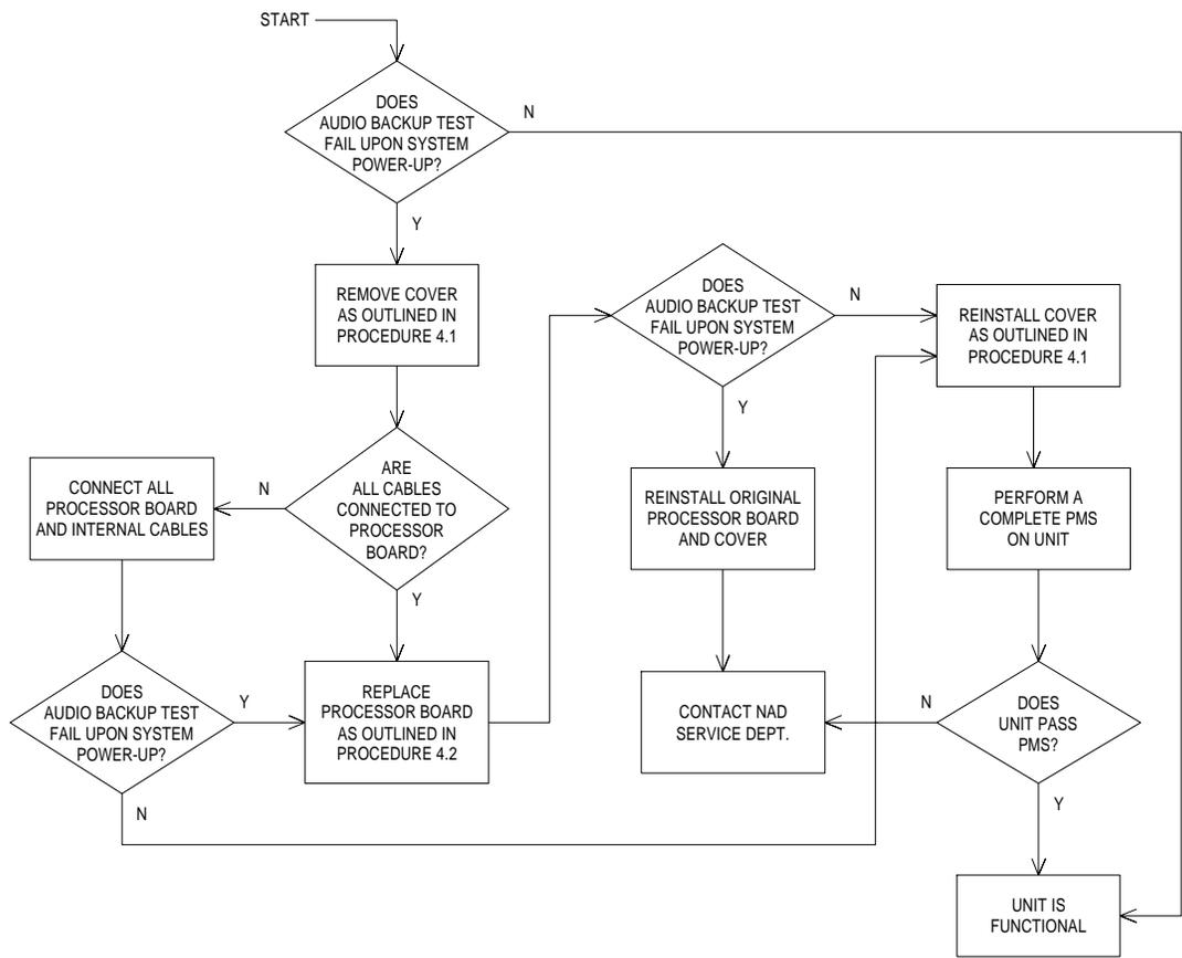
GUIDE 8: Audio Test - SpO<sub>2</sub> fails upon power-up
