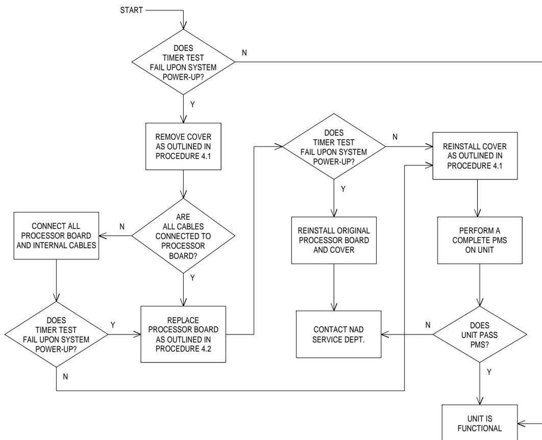
GUIDE 6: Audio Test - Primary fails upon system power-up
