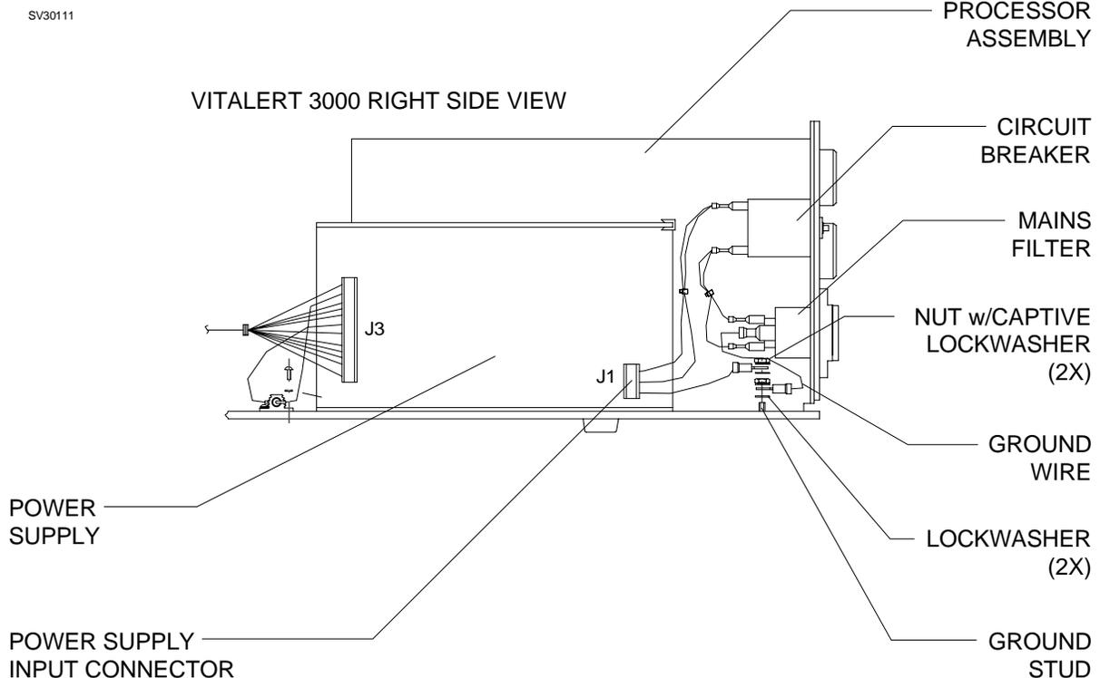
**Figure 4-2A: REPLACEMENT OF PROCESSOR ASSEMBLY (continued)**
