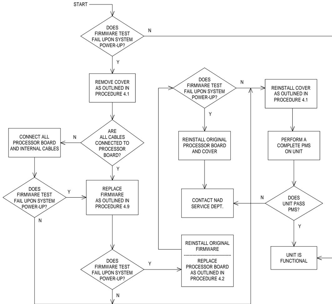
**GUIDE 3: Video Test fails upon system power-up**
