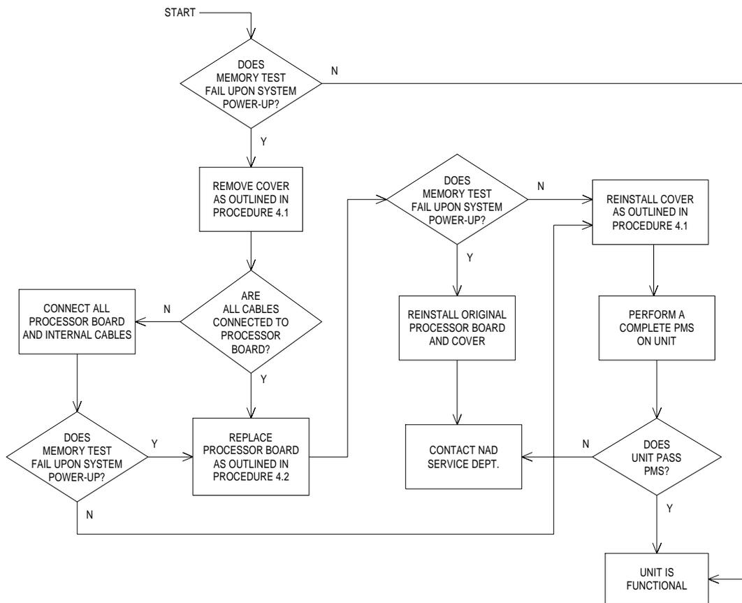
**GUIDE 5: Timer Test fails upon system power up**
