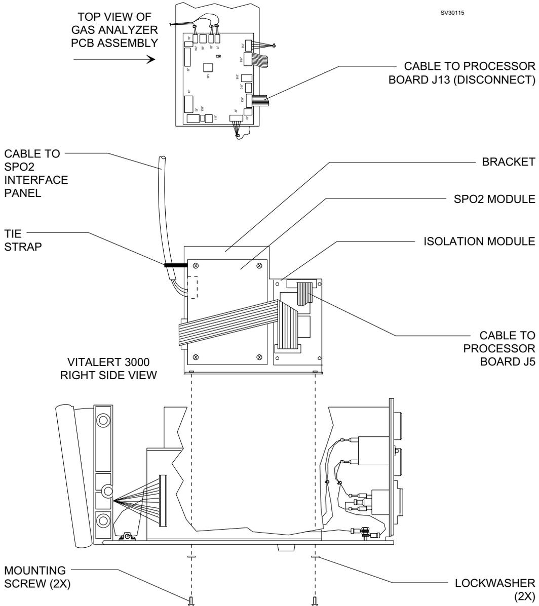
Figure 4-5: REPLACEMENT OF THE SpO<sub>2</sub> ASSEMBLY
