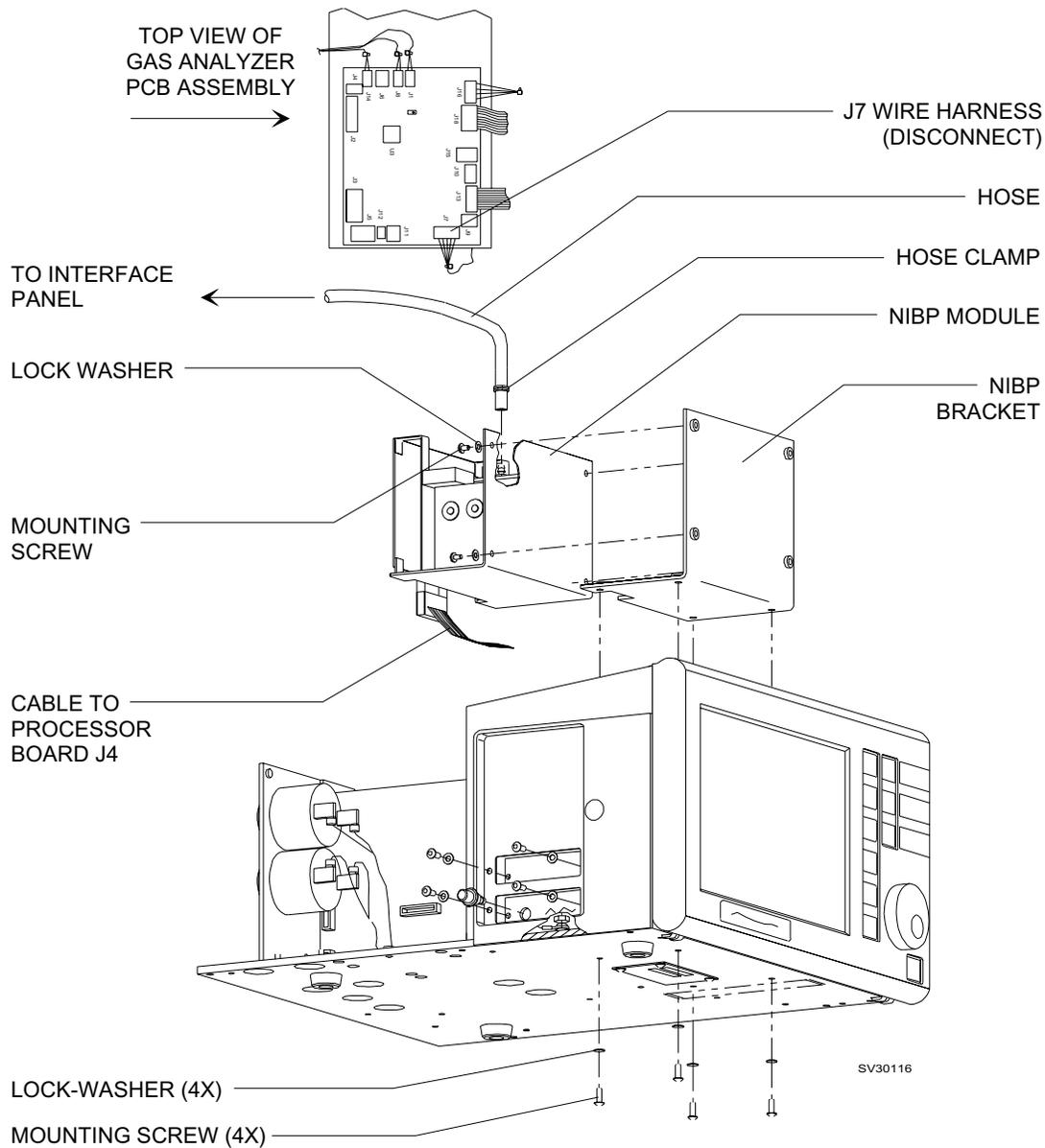
Figure 4-6: REPLACEMENT OF THE NIBP ASSEMBLY
