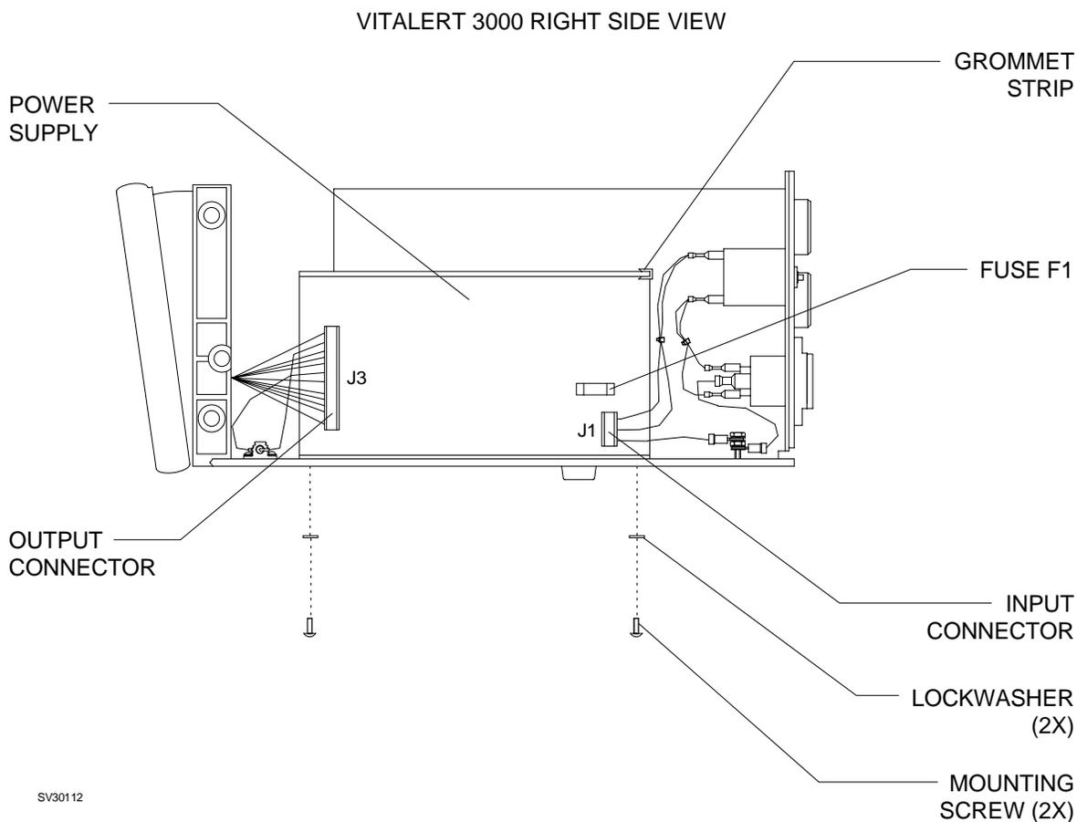
**Figure 4-3: REPLACEMENT OF POWER SUPPLY**
