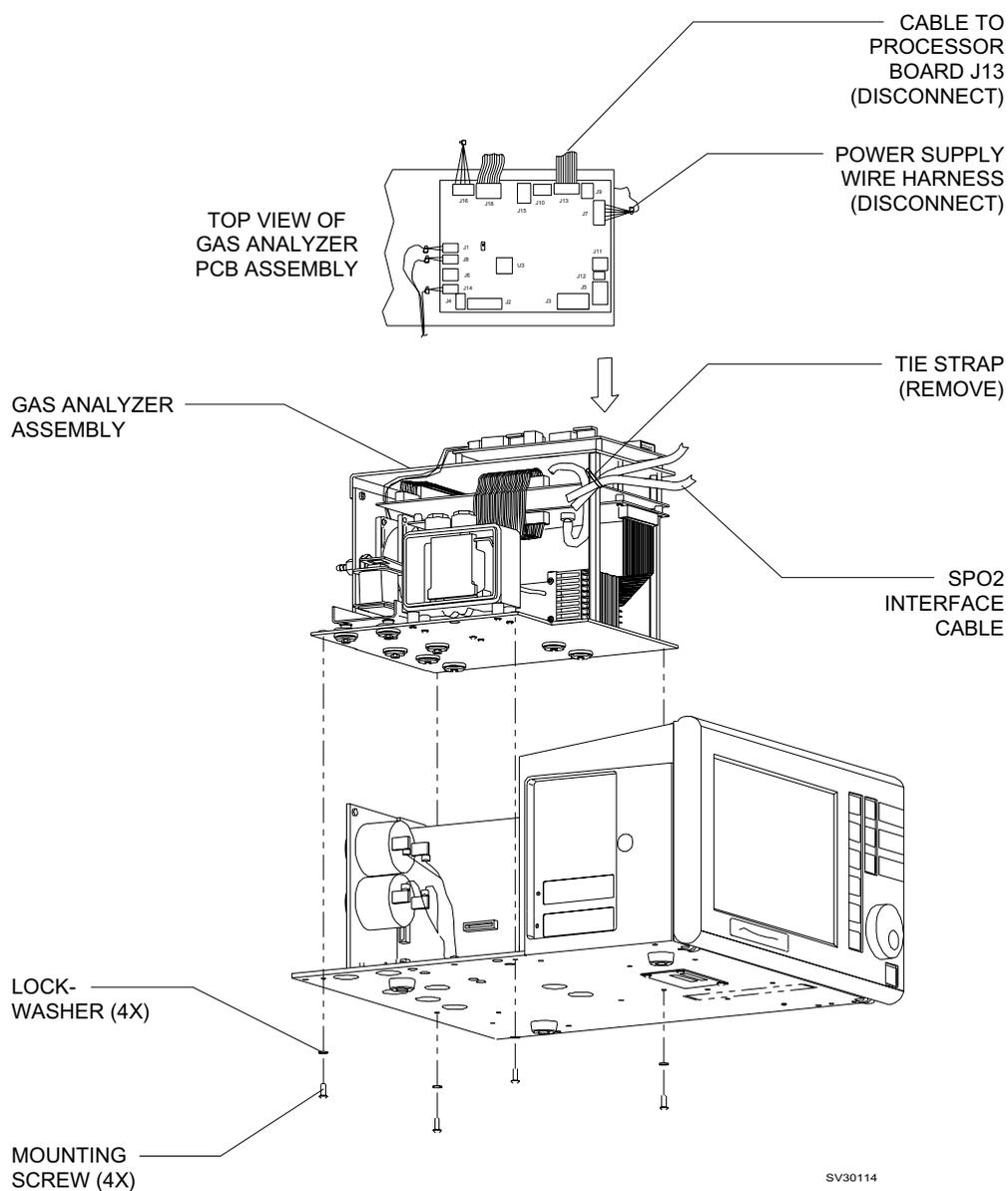
Figure 4-7: REPLACEMENT OF THE GAS ANALYZER ASSEMBLY
