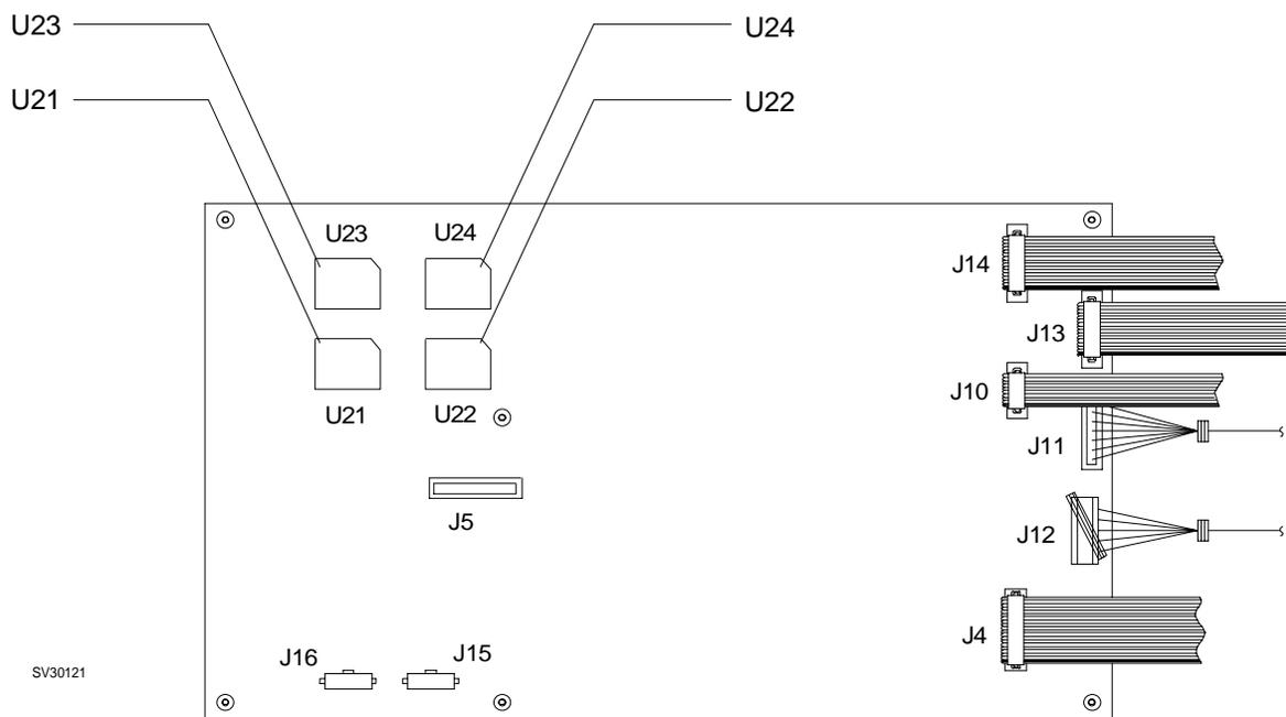
**Figure 4-9: PROCESSOR BOARD FIRMWARE LOCATIONS**
