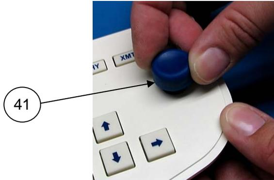
Apply the Keyboard Bezel Assembly to the Top Housing (part of the core BOM) as shown. Ensure the Bezel is centered in the opening.
