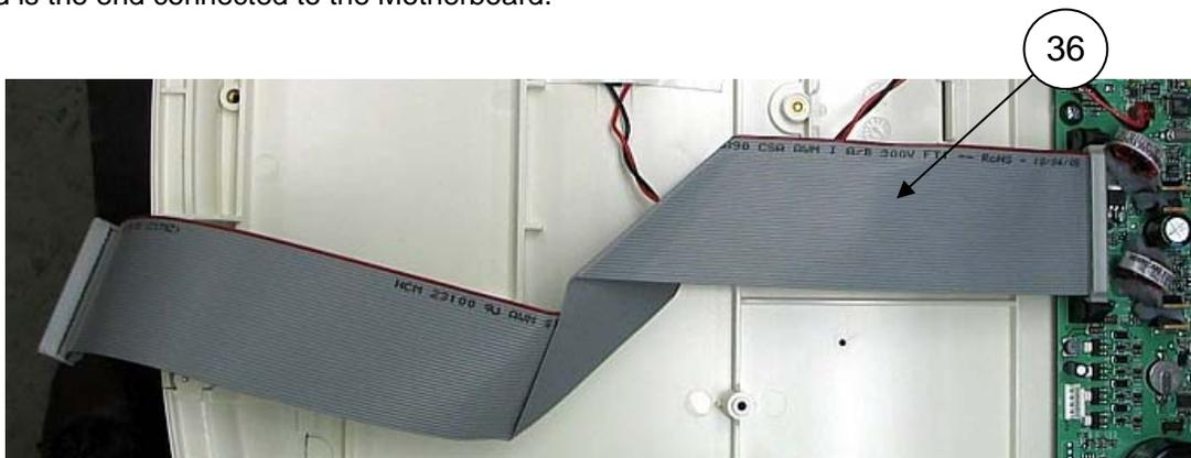
Install the cable retention clip (Item 26) inside the lower housing along the right side as shown. This will be used for routing the writer cables later in the assembly.
