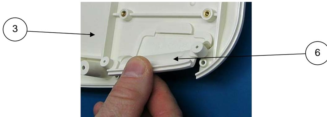
Flip the Lower Housing over and secure the Front Closure Plate to the Lower Housing using 2 screws (Item 30). Use a T9 bit. Torque Spec: Hand Tighten Only
