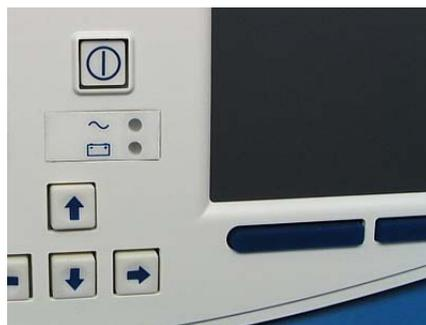
Apply the Keyboard Bezel Assembly to the Top Housing as shown. Ensure the bezel is centered in the opening.
