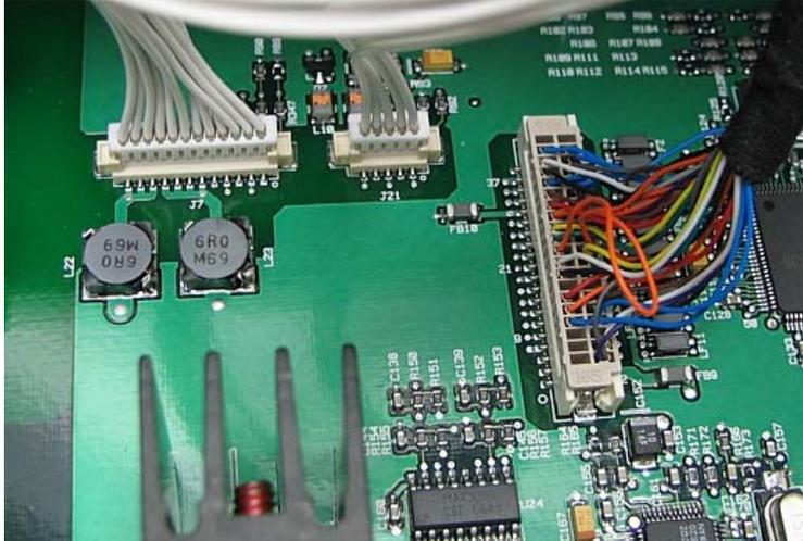
Tie-wrap (Item 25) the LCD display cables as shown to prevent them from getting pinched later in the hinge and rear cover housings. Cut the excess length from the tie-wrap.
