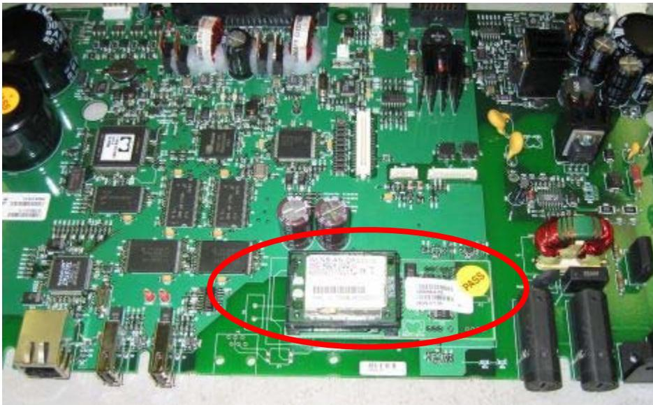
Figure 5-1 above shows the ELI 350 motherboard with the Wireless LAN option installed.
