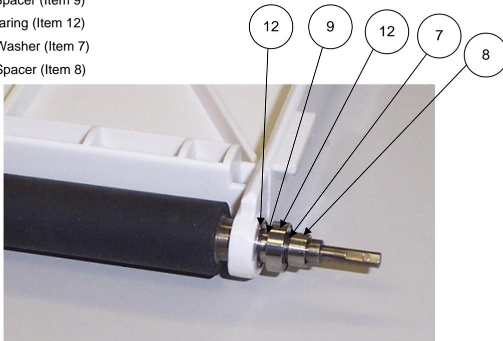
Lock the previous items in place with an E-Ring (Item 10) as shown. Make sure E-Ring snaps completely into the slot on the shaft.
