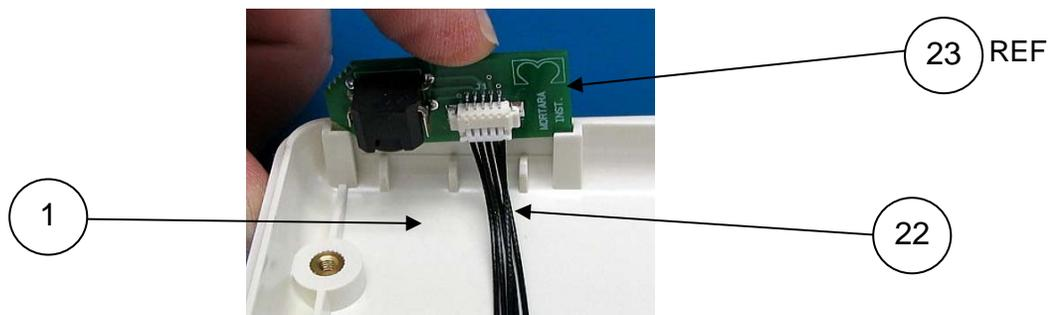
Route the tilt switch cable as shown using the rear housing as a guide. Retain the cable to the rear housing with tape (Item 29) 2 Plcs typical.
