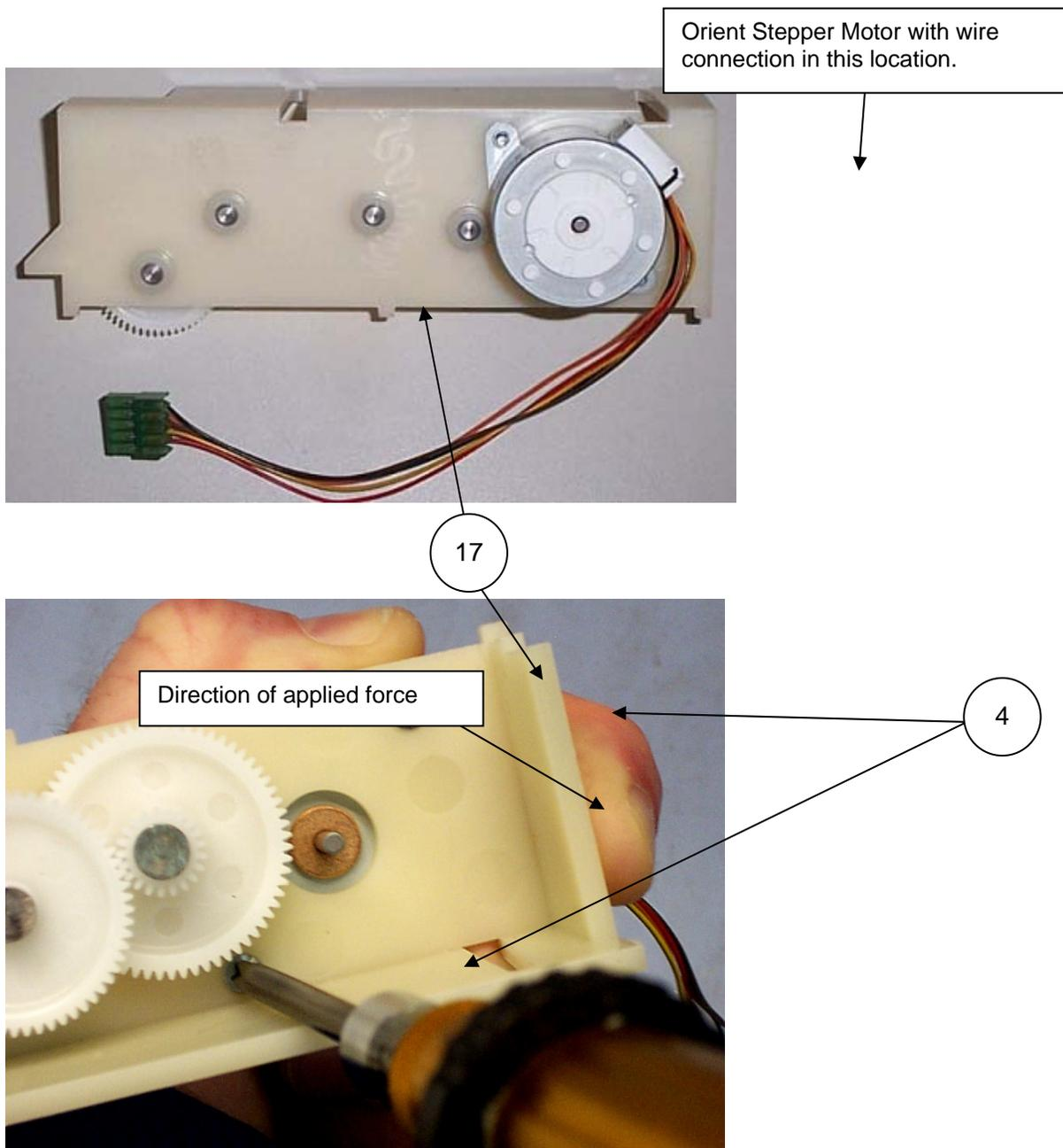
Install Vibra-Tite (Item 31) prepared Set Screw (Item 6) partially into Single Gear (Item 22). Slide Single Gear onto the shaft of the Stepper Motor (Item 13). Align the stepper motor gear flush with the edge of the large gear with which it meshes. Tighten Set Screw to secure Single Gear to Stepper Motor. Using your thumb, rotate the large gear to ensure smooth operation of the gear train.
