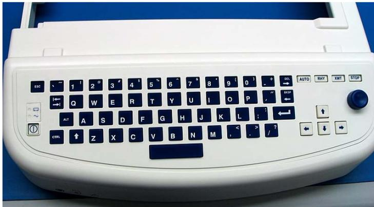
Flip the assembly over and secure the keyboard bezel to the top cover with 6 screws (Item 20).
