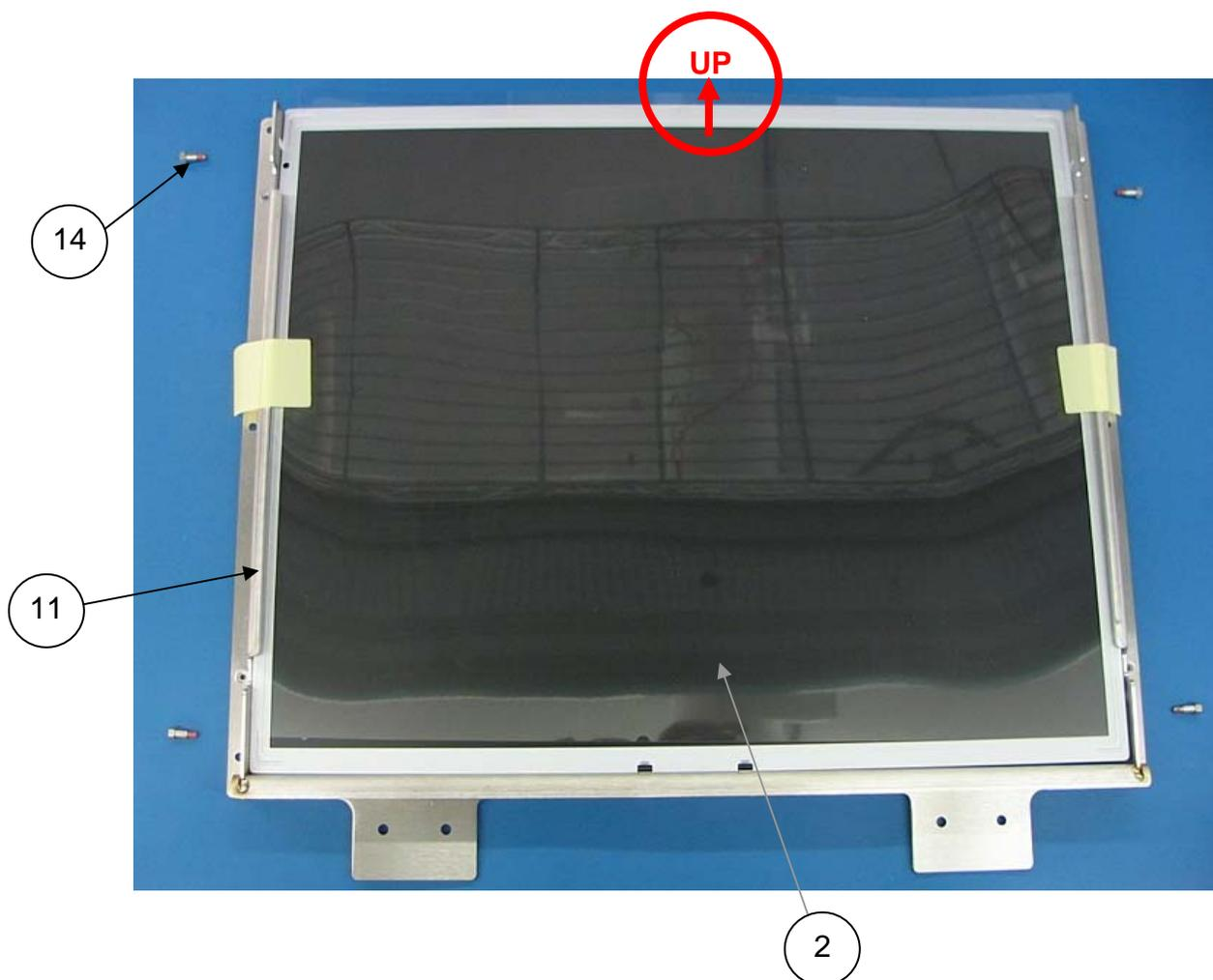
Flip the assembly over to mark the cable routings and backlight PCB location. Use caution not to damage the front of the LCD.
