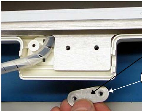
Note: Flat side of load plate must be up towards the rear housing.
