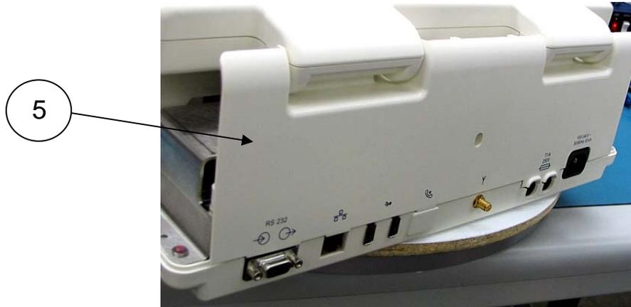
Close the LCD display in order to insert the Rear Housing to the Lower Housing. Mount the Rear Housing to the base assembly using 3 screws (Item 21)
