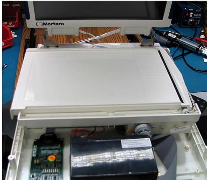
Connect the writer cue sensor to J15 and the stepper motor to J18 on the motherboard.
