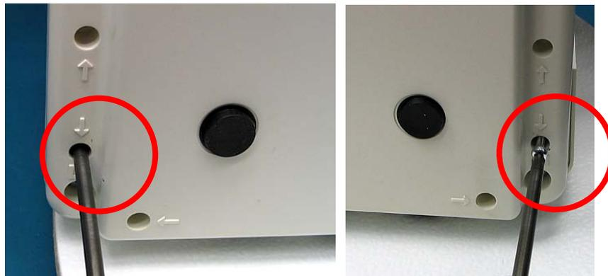
SNAP the Hinge Cover Housing to the Rear Housing. Ensure the LCD Monitor cables are not pinched between the housings.
