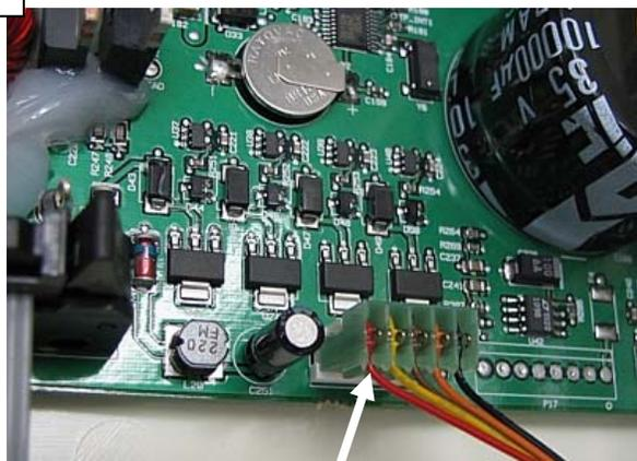
Connect the writer print head cables to the motherboard (longer cable to J13; shorter cable to J10).
