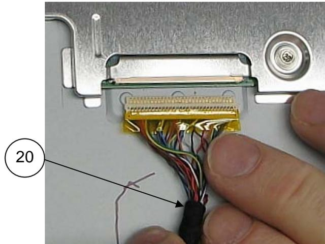
Route the cable as shown using the markings created on the LCD. Retain the cable to the LCD with a piece of tape (Item 29)
