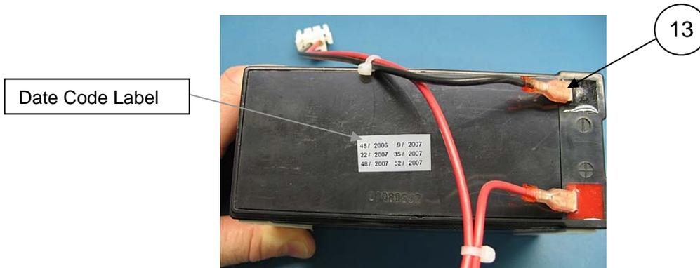
Remove paper backing from double sided tape and install battery into the lower housing as shown. Note the orientation of the battery terminals to the fuse holder.
