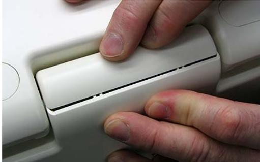
Assemble the applicable (Click Knob or Touch Pad) Top Cover Assembly as shown.
