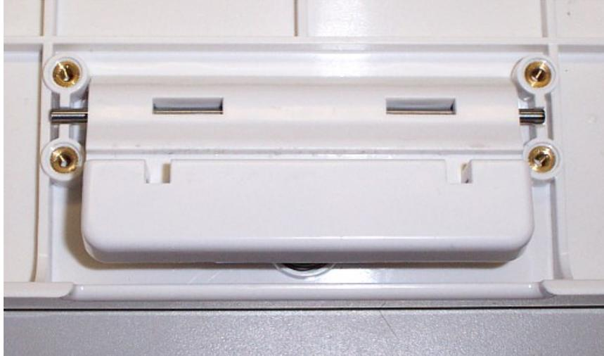
Place a Pivot Bar Restraining Plate (Item 26) over each end on the Pivot Bar and secure with four Screws (Item 4) as shown. Make sure Latch Release moves freely. Close and open the Paper Cover and verify it latches and releases properly. Leave Paper Cover open.
