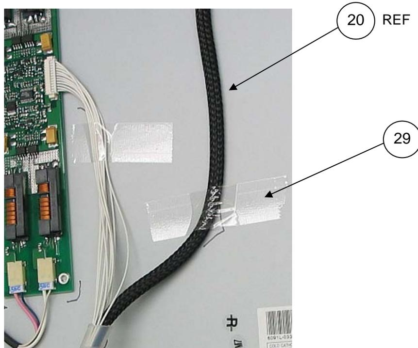
Cut a piece of 3/8" spiral wrap (Item 32) 4 inches long. Capture both the LCD Backlight cable and LCD Signal Cable within the spiral wrap as shown.
