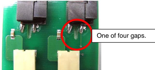
Remove the backing from the double sided tape and mount the Backlight Inverter Module PCB to the LCD centering within markings
