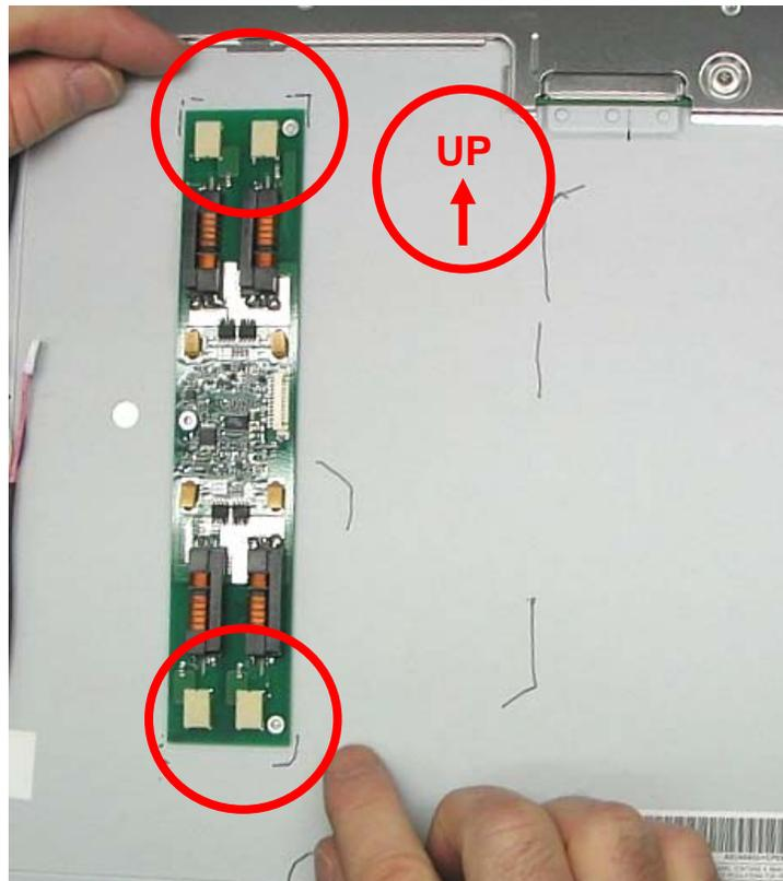
Plug the Inverted cable connectors from the LCD to the Backlight Inverter Module PCB as shown (4 Plcs).
