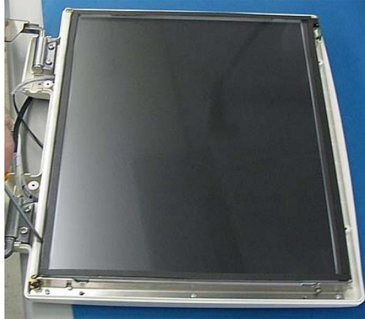
Assemble Front Bezel (Item 3) to the Rear Housing (REF: Item 1) using screws (Items 27, 4 Plcs). Ensure cables are not pinched between the front and rear housings.
