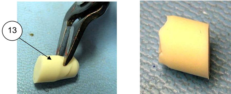
Insert the Elastomeric Plugs in the top two (2) screw hole of the rear housing. Ensure the plugs are flush to the housing. Note: the beveled side of the plug must match the bevel of the rear housing.
