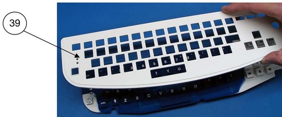
Apply the Battery / Power Label (Item 40) to the Keyboard Bezel.
