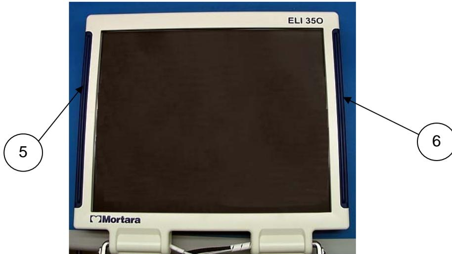
Apply Tilt Switch Label (Item 15) to top of the finished display
