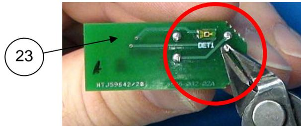
Connect the Tilt Switch cable (Item 22) to the Tilt Switch PCB Assembly (REF: Item 23) and insert the PCB into the display Rear Housing (Item 1) as shown.
