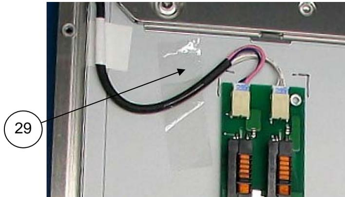
Insert the Backlight Inverter cable (Item 21) to the PCB Assembly. Route the cable as shown using the markings created on the LCD and retain the cable to the LCD with a piece of tape (Item 29)
