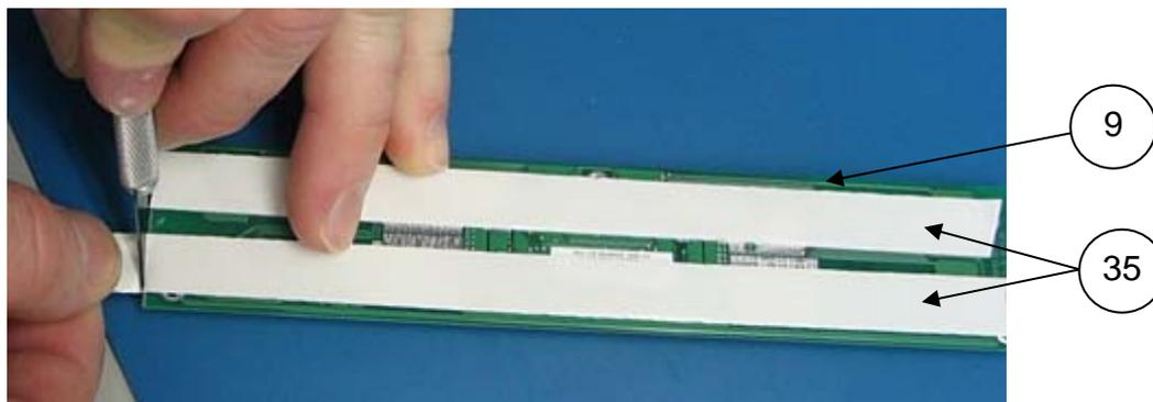
Ensure the tape covers each of the 4 High Voltage spark-gap holes located between the connectors and coils. (Top side view)
