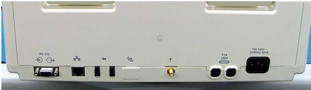
Antenna shown here connected for test purpose only. Disconnect the antenna to ship along with the unit.
