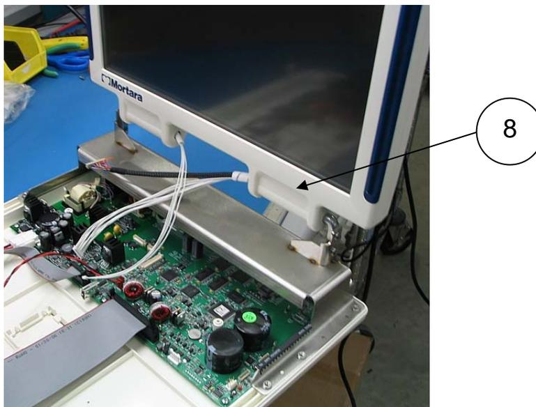
Secure the LCD Display assembly (Item 8, Ref) to the Lower Housing using 4 screws with Vibra-Tite (Item 31) in the locations marked with the display mount symbol.
