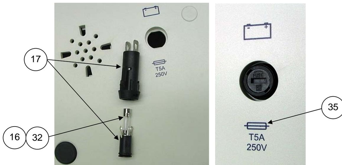
**IMPORTANT** – The battery fuse on the ELI 350 unit is dependent upon the item number of the unit's motherboard. Units manufactured with the older motherboard (Item #26025-076-51) use a 5A fuse; and those manufactured with the newer motherboard (Item # 26025-076-52) use an 8A fuse. Fuse labeling shown above is for the 5A fuse application; fuse rating labels (Item # 35) are available to properly label the unit chassis if a fuse rating change is required, due to a motherboard service replacement.
