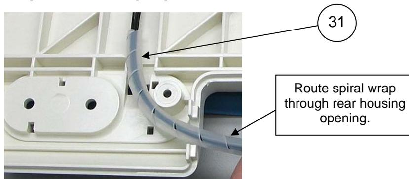
Flip LCD electronic assembly over and place into the back housing as shown
