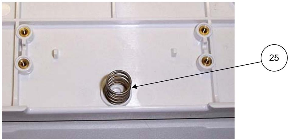
Place Latch Release with Pivot Bar installed onto Compression Spring as shown. Make sure Compression Spring sets in the spring capture area provided on Latch Release.
