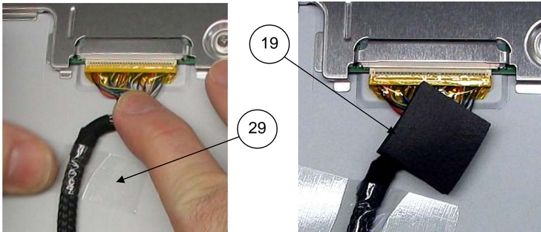
Apply LCD support block foam (Item 19) to retain signal cable top to the LCD.
