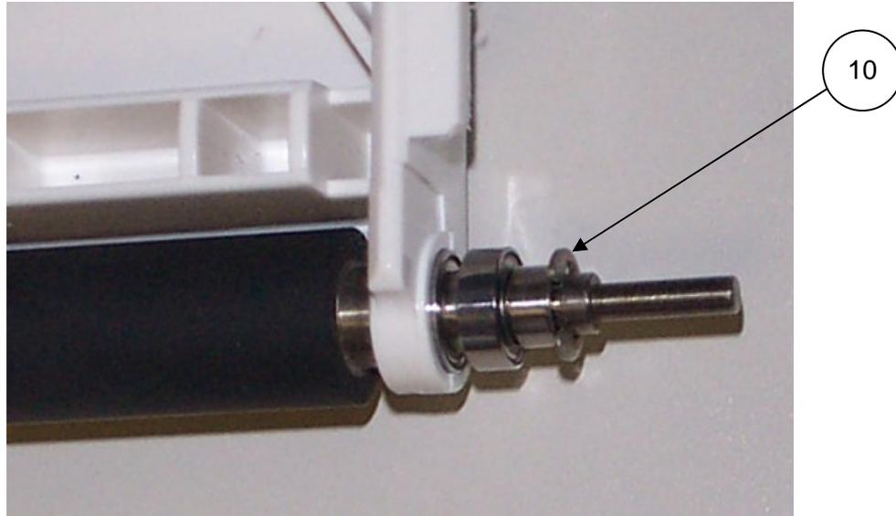
Slide the following items onto the shorter side of the Platen in the order listed. The first Ball Bearing should slide into the open loop on Paper Cover.
