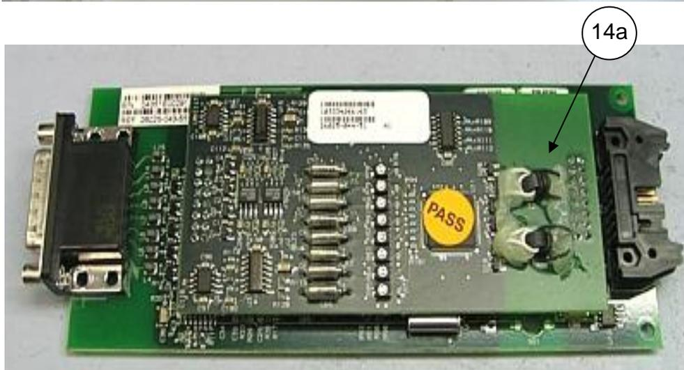
If the 10K+ AUXILIARY PCB ASSY (Item 14a) is needed for the 15 lead option, install the 10K+ AUXILIARY PCB ASSY onto Front End PCB (Item 14) prior to installation of Front End PCB (Item 14) Assy.
