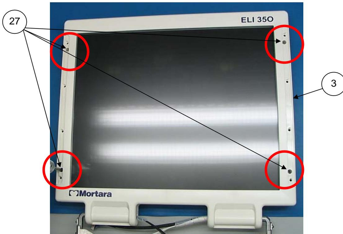
Flip the assembly over and fasten the Rear Housing to the Front Bezel using screws (Items 27, 4 Plcs).
