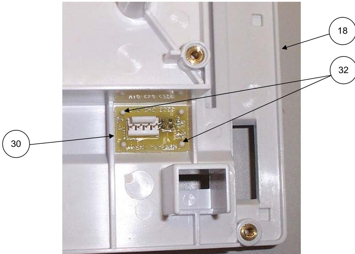
Connect Cue Sensor Cable (Item 29) to Cue Sensor PCB as shown.
