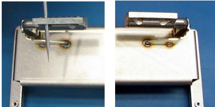
Apply Vibra-Tite (Item 30) to 4 Screws (Item 36). Mount hinge assembly to LCD Back Housing Assembly using Hinge Load Plate (Item 12, 2 Plcs) and Screws (Item 36, 4 Plcs). Torque 18 in-lbs.
