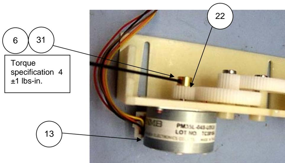
Prepare three Screws (Item 5) by brushing Vibra-Tite (Item 31) onto the threads as shown. Allow to dry for a minimum of 10 minutes. Note: This step may be done prior to assembling the unit so the Vibra-Tite has time to dry and the screws are ready to install. If the parts already have Vibra-Tite on the threads this step can be skipped.
