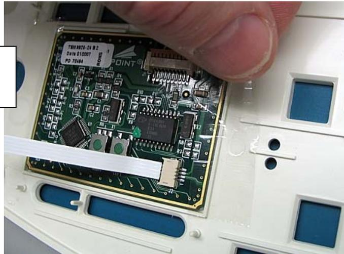
Feed the USB Cable and the flex circuit through the opening in the Keyboard PCB assembly. Pull up on J2 connector ears (on Keyboard PCB) to open connector. Insert the flex cable into the connector. Push the connector ears down as shown.
