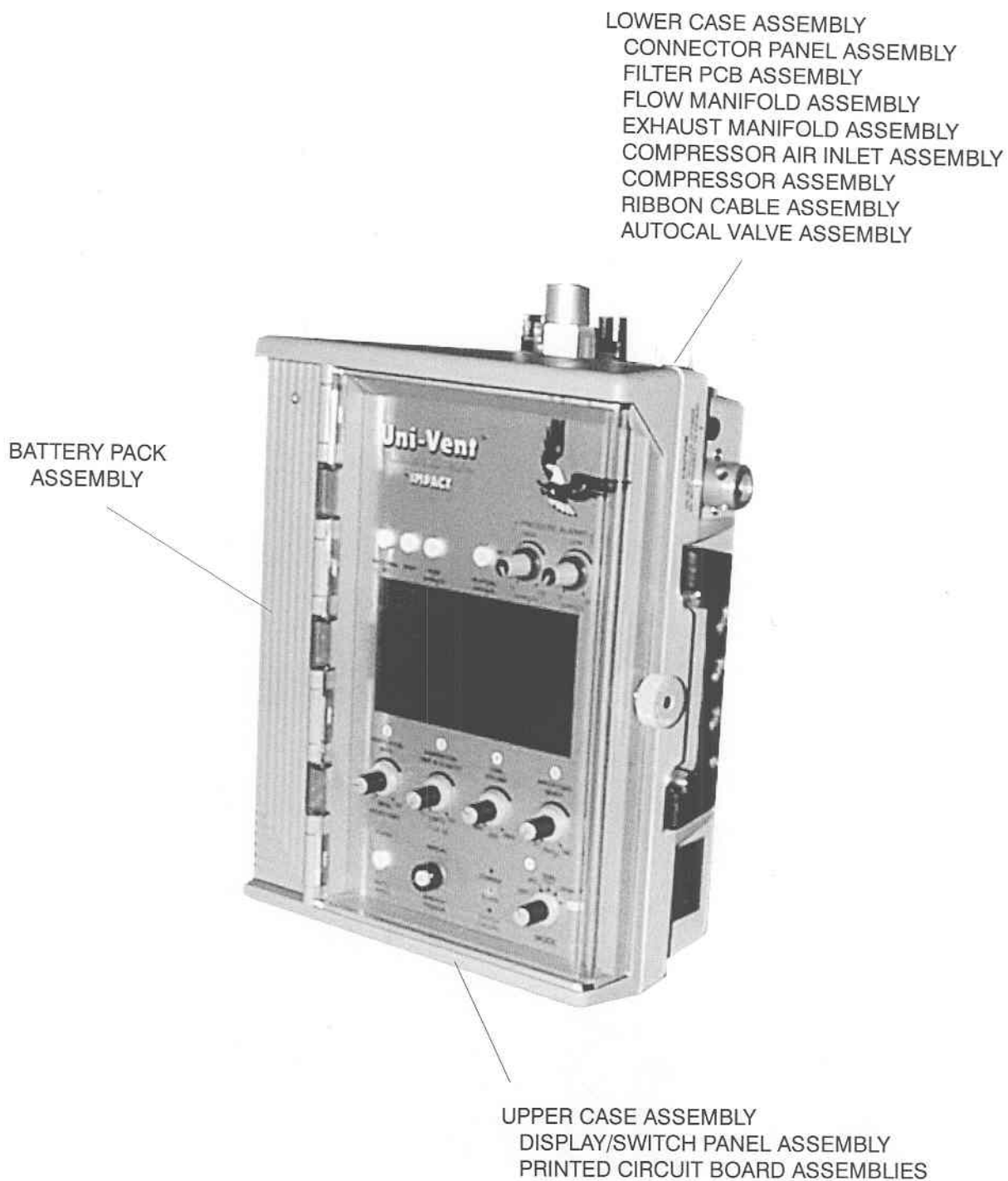
FIGURE 6, COMPOSITE ILLUSTRATION DEPICTING MAJOR SUB-ASSEMBLIES
