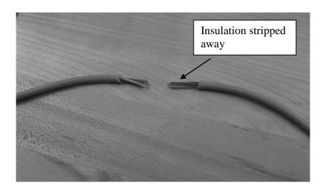
Pair the wires by color. Match the wires on one side of the cable to the corresponding wires on the other side. Twist each group of wires together tightly. Your cable may have a shiny jacket around the wire. The shiny jacket must also be connected between the two halves of the cable.
