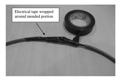
For broken wires with no visible damage:
