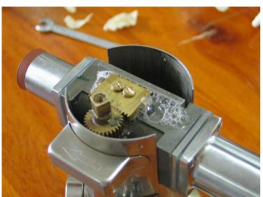
Finally the leak test. Block outlet connector and connect an air source and a pressure gauge to the inlet. (An old sphygmometer works very well) Pump air into the system until approximately 200 mmHg. Close the air way. The pressure will fall slowly. The time for falling until 190 mmHg should be at least 30 seconds. Do the test with pointer in 'OFF' and in '3.5' position.
