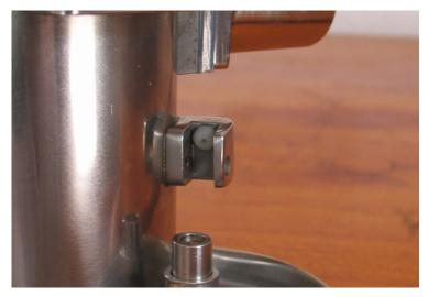
While assembling be sure that the lever covers the hole of the white plastic nozzle properly.
