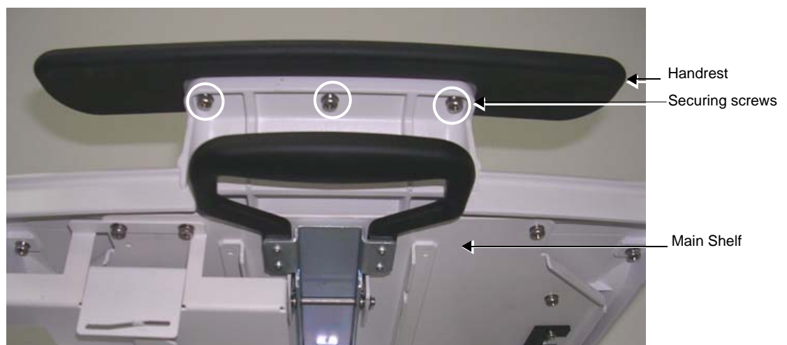
Figure 8-106 Handrest Secured to Main Shelf (viewed from below)
