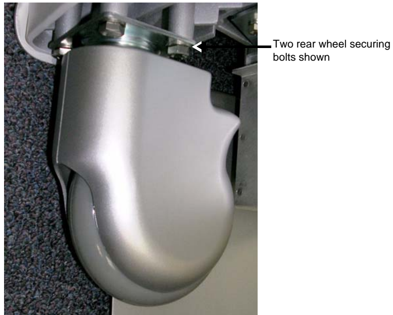
Figure 8-111 Rear Wheel Bolted to SafeLock Cart Chassis
