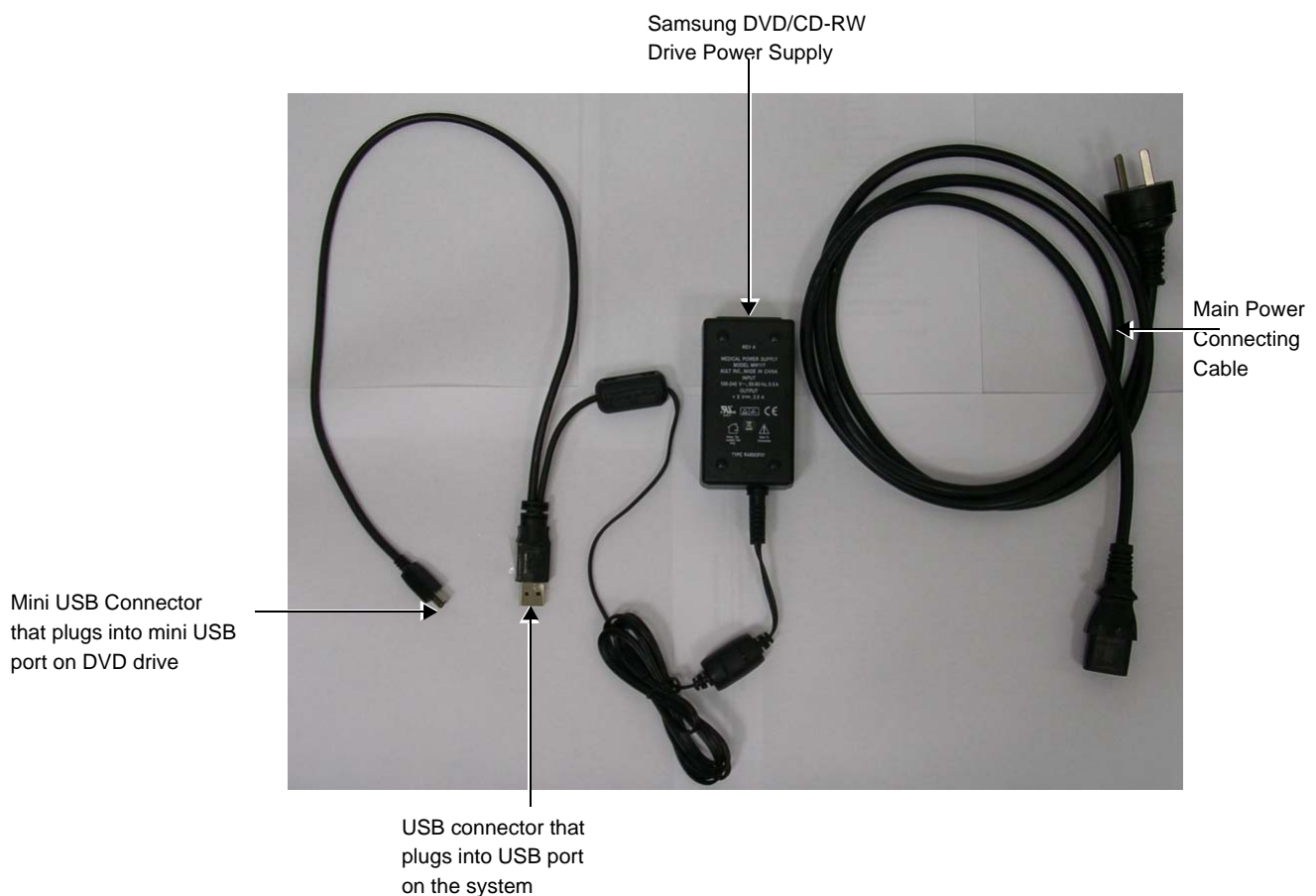
Figure 3-29 Vivid q N Power Supply with Two USB Connectors
