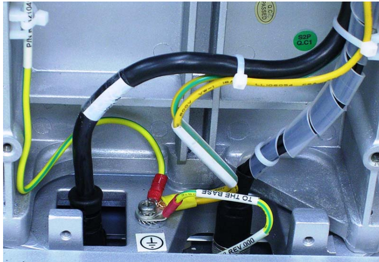
Figure 8-94 Peripheral AC Outlet and Ground Cable Connected
