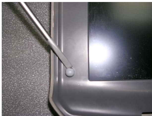
Figure 8-28 Removing the Screw Caps from the LCD Display Frame
