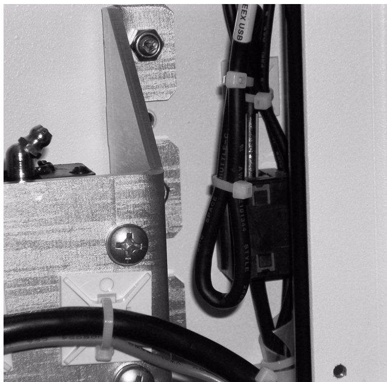
Figure 8-95 USB Power Cable Folded and Fastened with Tie-wraps
