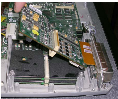
Figure 8-33 Removing the Probe and MUX Board from the Bottom Assembly
