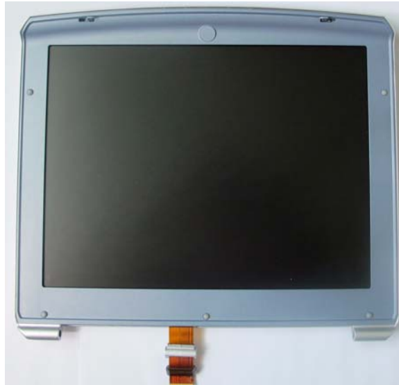
Figure 8-63 AUO LCD Display Assembled in Display Frame
