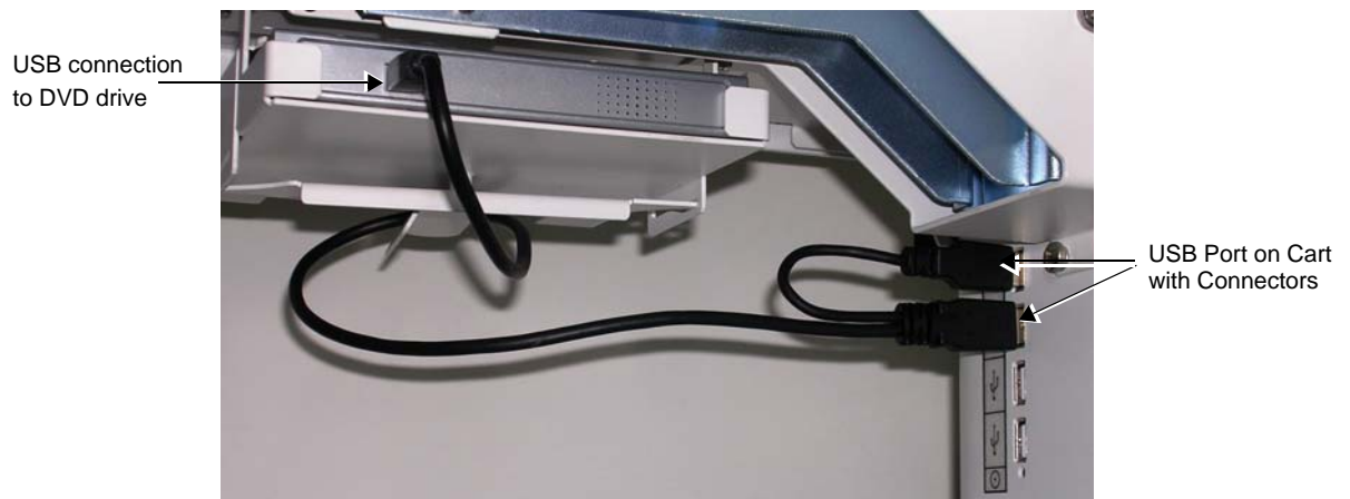
Figure 3-35 USB Cable Plugged Into the DVD/CD Drive and the Cart's USB Connectors
