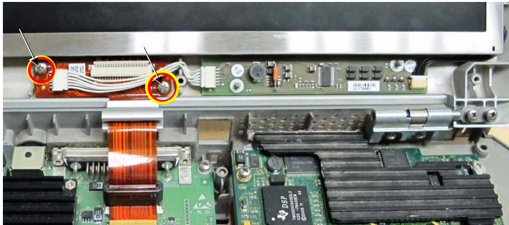
Figure 8-75 AUO LCD Display located in the Vivid q N Top Rear Cover
