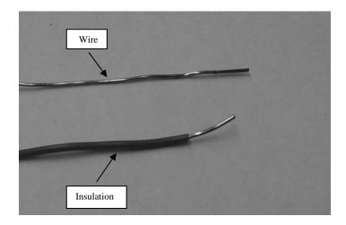
Many different non-conducting materials can be used as insulation. Plastic insulation can be used for most projects. Plastic insulation is low-cost. Plastic insulation is appropriate for dry environments. Plastic insulation can be used for color-coding.
