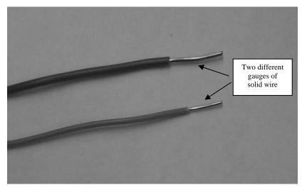
Wire is sized according to standard gauges. The two primary wire gauges are the American Wire Gauge (AWG) and the Metric Wire Gauge (MWG).
