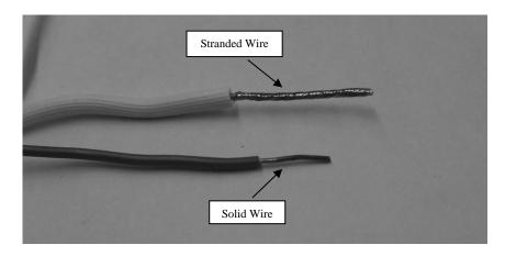
Solid wire conducts well. Solid wire is very stiff. Solid wire may break if it is forced to bend. Solid wire should always be used unless the wire must be able to bend or move easily.
