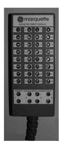
The equivalent to the Stimulus Inputs 1-4 on the Stimulator Input Cable are labeled on the CardioLab II Plus Amplifier as Stimulus Inputs A1, A2, B1 and B2.
