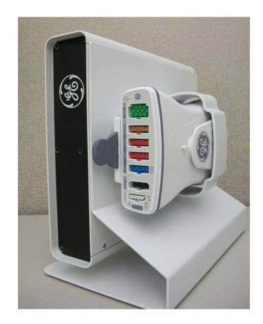
The PDM Base Station may also rest with its feet on the floor, connected to the PDM by a longer cable. In this setup, the PDM dock is attached to the pole/rail clamp, which clamps onto a bed rail or pole. The pole/rail clamp is attached and detached by adjusting the clamp knob. Ensure the knob is fully tightened when clamping to bed rails and poles.
