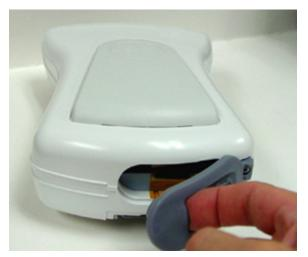
2. Pull the battery tray out of the PDM using the battery tray strap and remove the battery from the battery tray.
