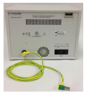
Connect the other end of the cable to the equipotential connector on the patient table. If the equipotential connector on the table is in use, use the equipotential junction box to allow for the connection of multiple cables to the table as shown below:
