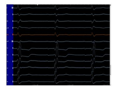
Typically, Power Line Frequency noise is the result of a difference in ECG lead wire impedance (poor connection with the patient). For CardioLab systems, Power Line Frequency can induce noise on the CardioLab II Plus Amplifier.
