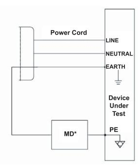
**NOTE:** The measuring device (MD) represents the safety analyzer.
