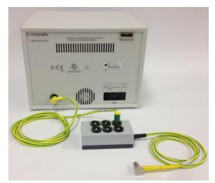
All of the patient connected equipment may be connected to the table using the junction box.
