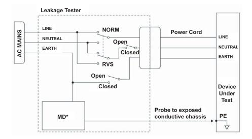
**NOTE:** The measuring device (MD) represents the network and voltage measuring instrument and its frequency characteristics per IEC 60601-1.
