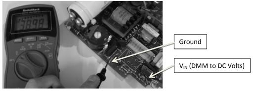
2. With the probes in the same positions as in step 1, set the DMM to read AC and take the following reading.
