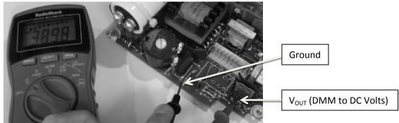
4. With the probes in the same positions as in step 3, set the DMM to read AC and take the following reading.
