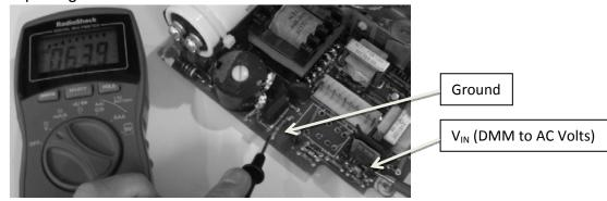
3. Now place one probe from the DMM on the output pin of the linear voltage regulator. You may need to consult the data sheet to determine the output pin. The other probe should remain on the electrical ground.
