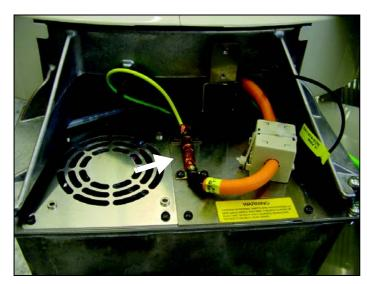
Shield on the tube assembly
