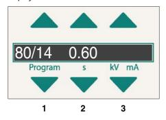
The single-line display of the Control Pad shows the exposure parameters.
