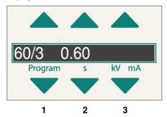
The single-line display of the Control Pad shows the exposure parameters.
