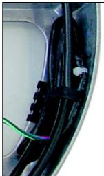
Lay cable in a single loop and fasten it with a cable tie.
