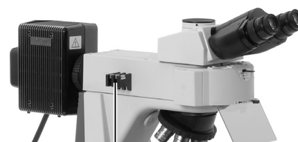
ND filter attach/detach lever
