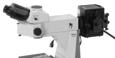
Mercury lamp house fitted in place
