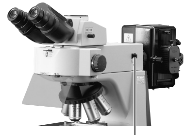
Fully open the field diaphragm.
