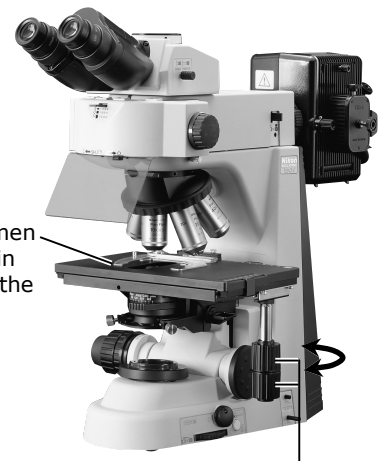
Move the portion to be viewed into the optical path using the XY stage knobs.
