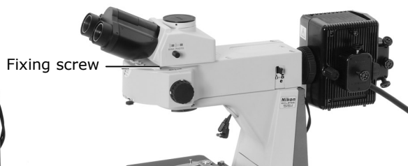
Trinocular eyepiece tube mounted on the fluorescent unit
