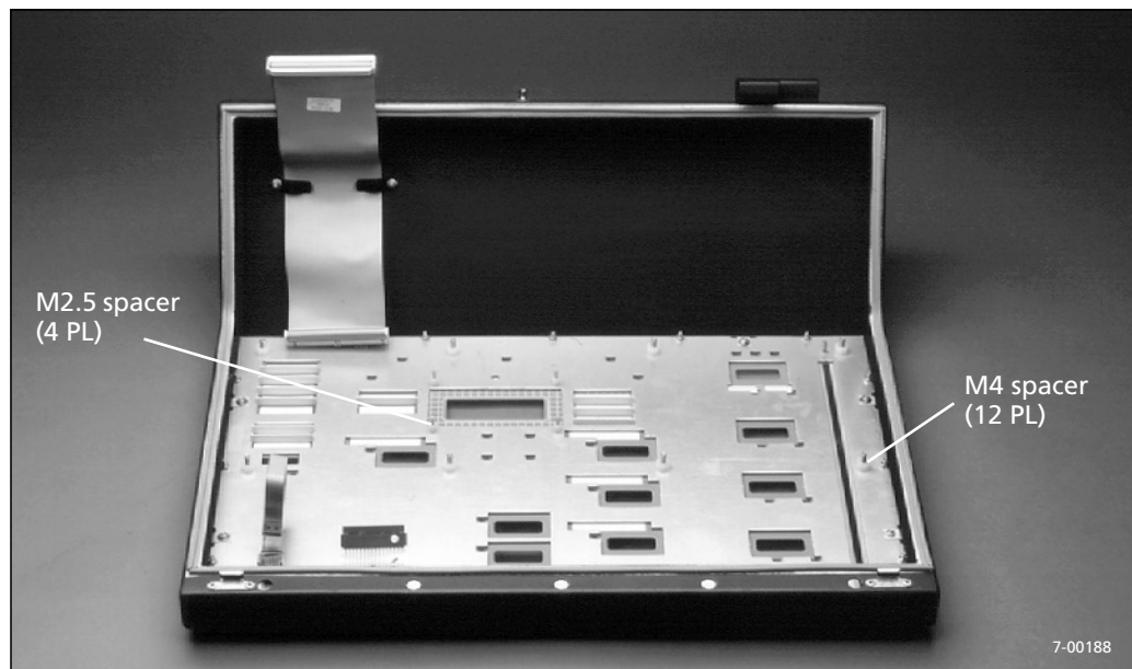
Figure 8-14. Spacers on keyboard assembly
