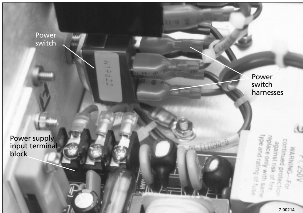
Figure 8-55. Power supply input terminal connections
