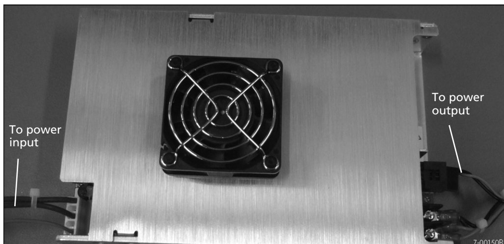
Figure 2-29. Power supply with harnesses
