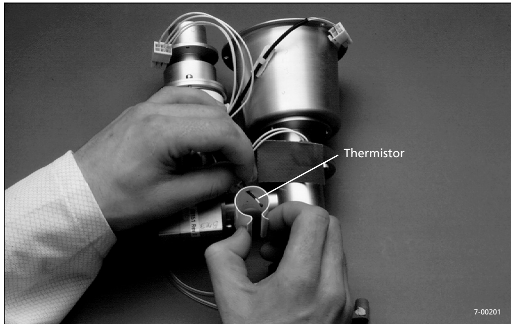
Figure 8-37. Threading thermistor through flow sensor heater clip
