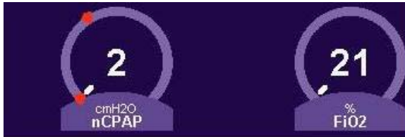
Figure 6: nCPAP Primary Controls and Alarm Threshold Indicators
