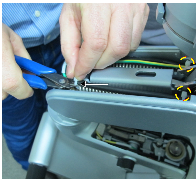
Figure 8-101 Cutting Tie-wraps on the Articulated Arm
