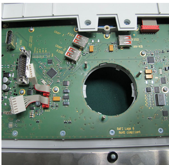
Figure 8-94 Trackball Board and Housing Removed
