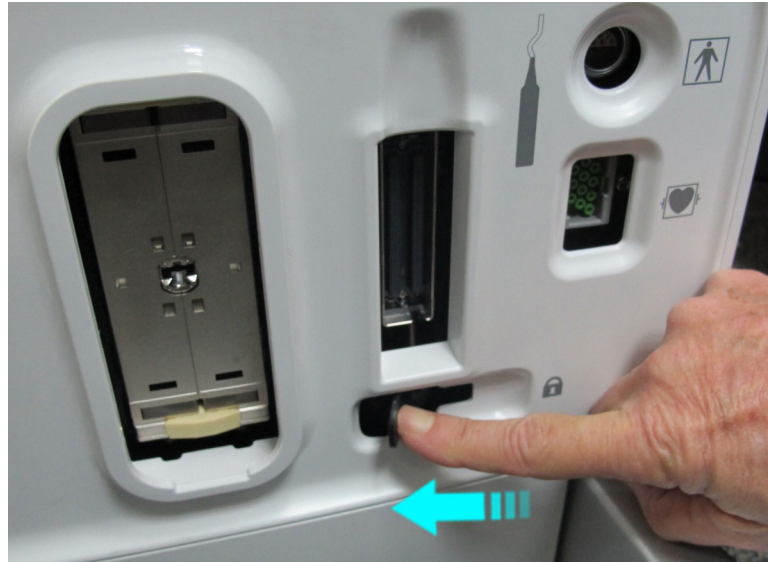
Figure 8-11 RS Probe Connector Lock - OPEN
