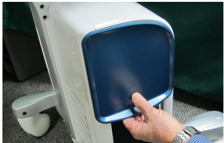
Figure 8-8 Removing the Blank Cover
