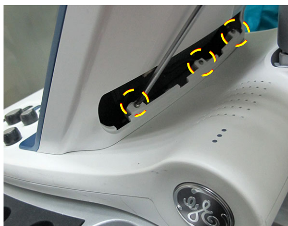
Figure 8-65 Removing the Rear Cover (Base) Securing Screws
