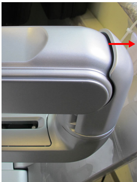
Figure 8-222 Removing Vertical Articulated Arm Service Cover
