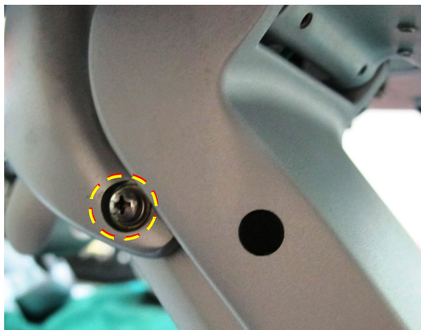
Figure 8-106 Lower Arm Securing Screws
