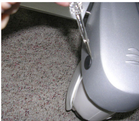
Figure 8-277 Removing the Screw Cap
