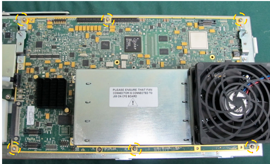
Figure 8-166 CFE Board showing 6 Retaining Screws
