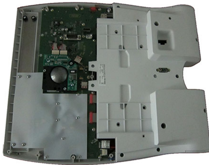
Figure 8-88 Operator Panel Keyboard Assembly with AN Keyboard/Bottom Cover Removed
