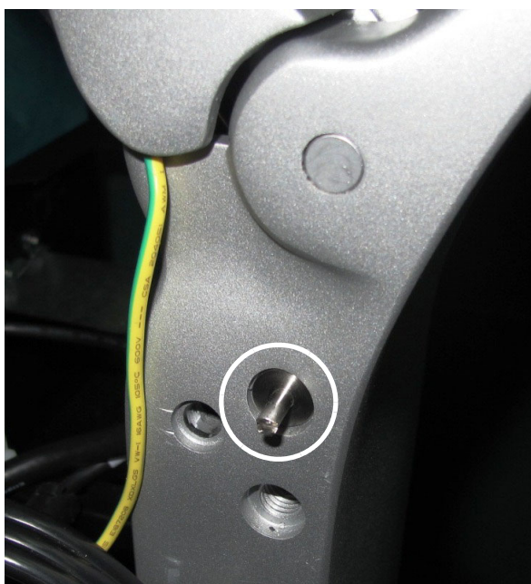
Figure 8-254 Shaft Covering Screws
