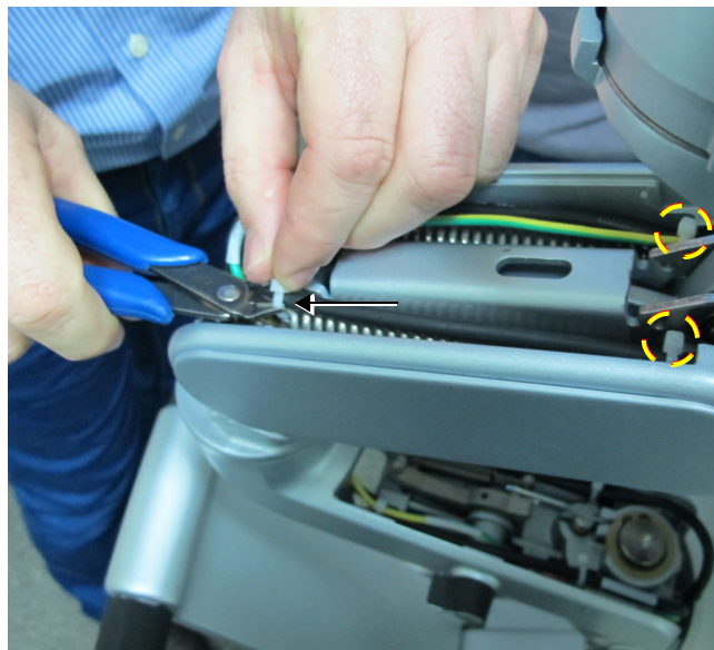
Figure 8-227 Cutting Tie-wraps on the Articulated Arm
