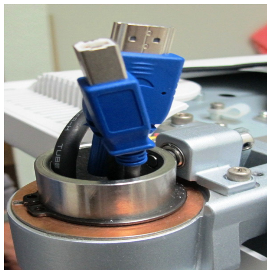
Figure 8-103 Monitor Cables Threaded Through Arm Aperture
