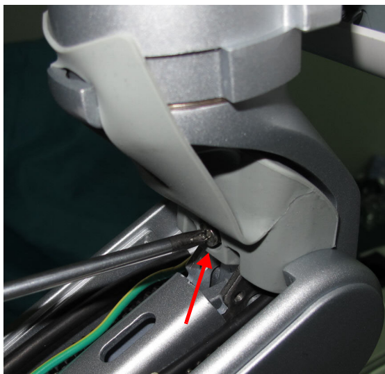
Figure 8-224 Removing the Protective Pad
