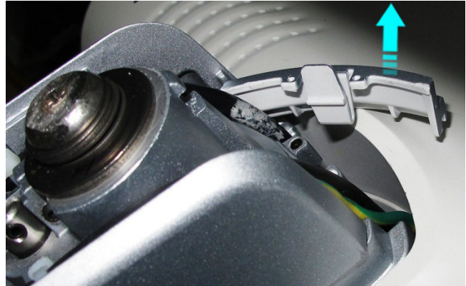
Figure 8-61 Removing the Monitor Arm Base Cover
