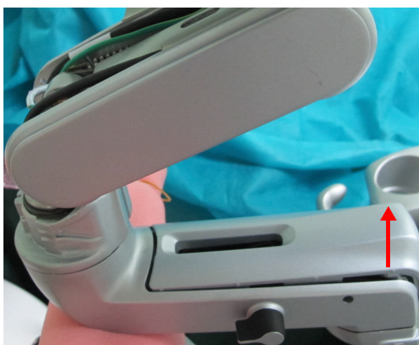
Figure 8-225 Removing Lower Horizontal Articulated Arm Cover
