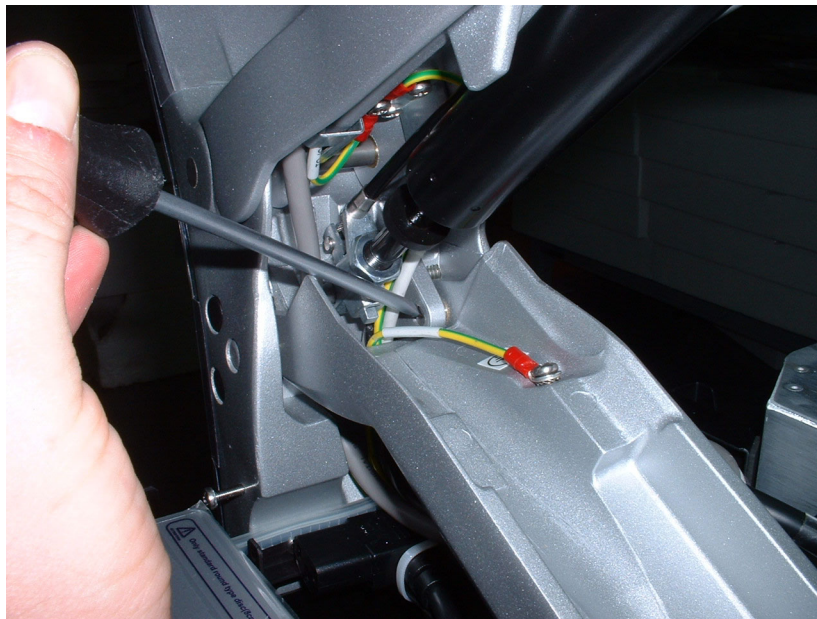
Figure 8-246 Removing Securing Pin and Disconnecting Ground Lead
