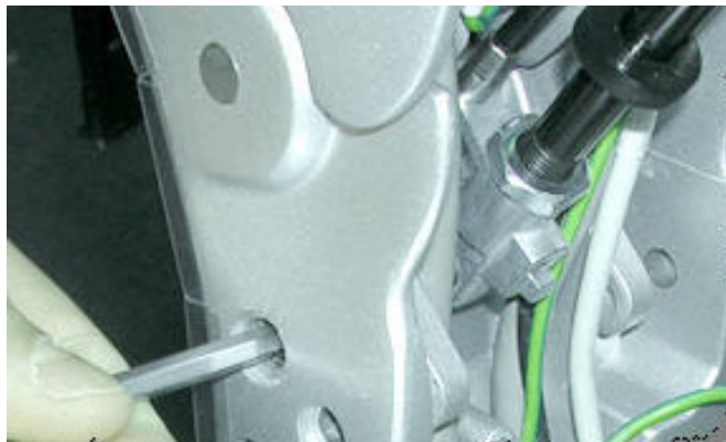
Figure 8-255 Releasing the Securing Screws on Either Side of the Support Arm
