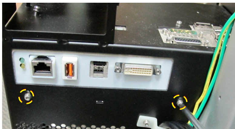
Figure 8-180 Removing the BIF Board Securing Screws Located at Rear of System
