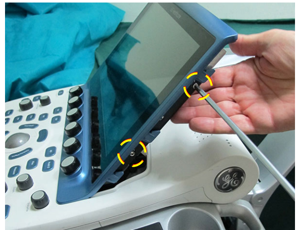
Figure 8-68 Removing the Touch Screen Securing Screws
