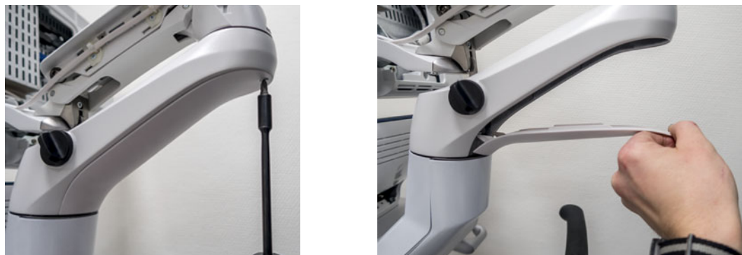
Figure 8-213 Remove the Lower Service Cover
