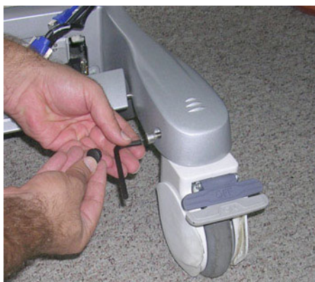
Figure 8-278 Removing the Securing Screw
