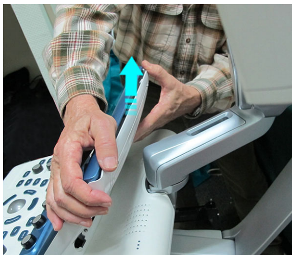
Figure 8-67 Removing the Touch Screen Rear Cover
