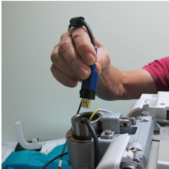
Figure 8-120 Feeding Cables through Top Aperture
