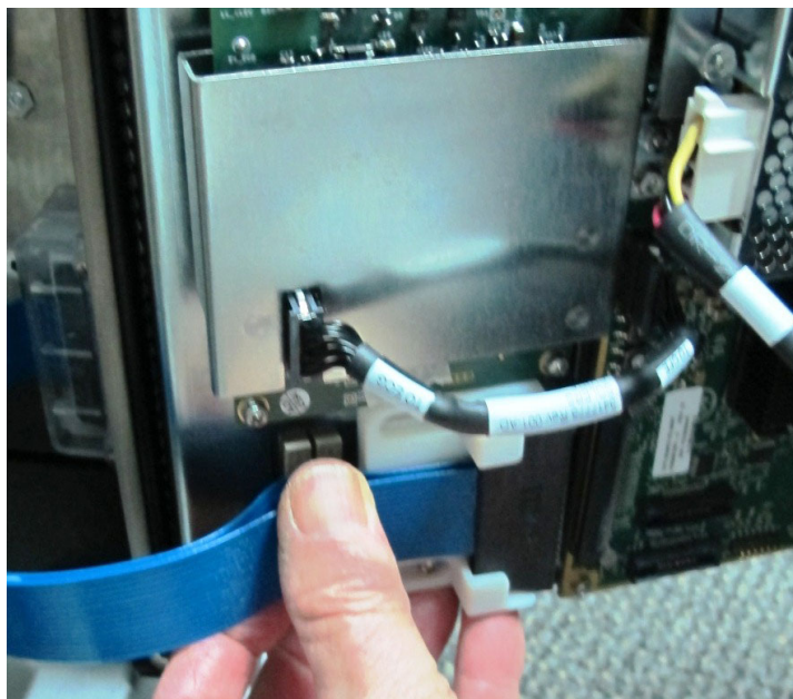
Figure 8-138 Releasing the HDR flat cable from the CFE
