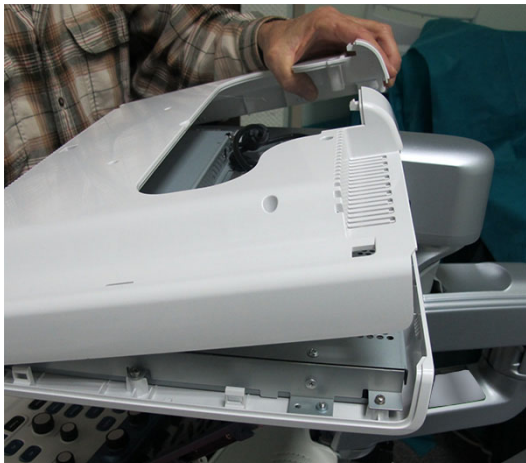
Figure 8-42 Removing the Monitor Rear Cover
