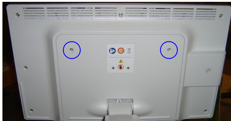
Figure 8-32 Monitor Rear Cover's fixing screws
