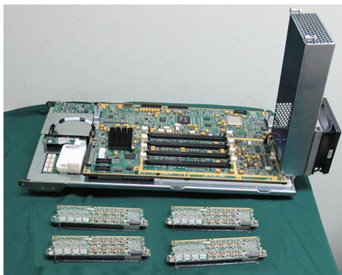
Figure 8-186 All TRX32 Boards Removed
