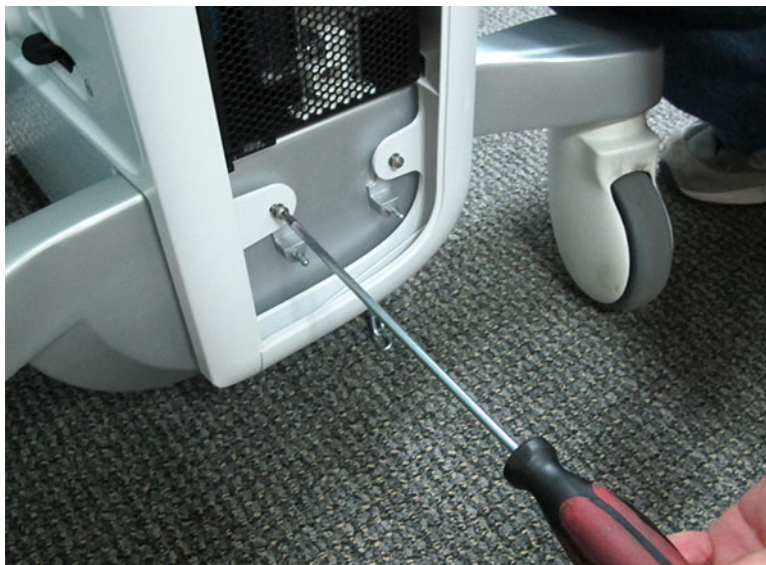
Figure 8-13 Removing Screw from Front Cover Securing Tab
