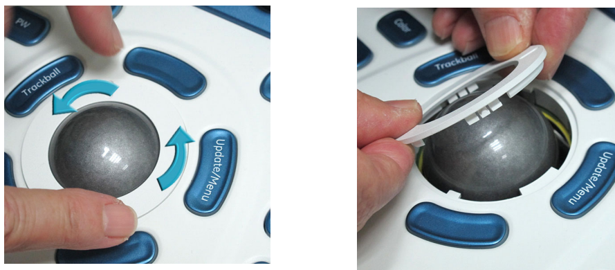
Figure 4-11 Removing Top Locking Plate and Rubber Dust Filter Ring
