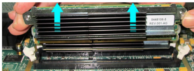
Figure 8-185 Removing a TRX32 Board
