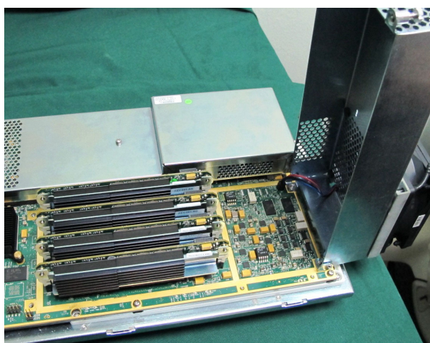
Figure 8-183 Opening the Metal Cover of the TRX32 Box
