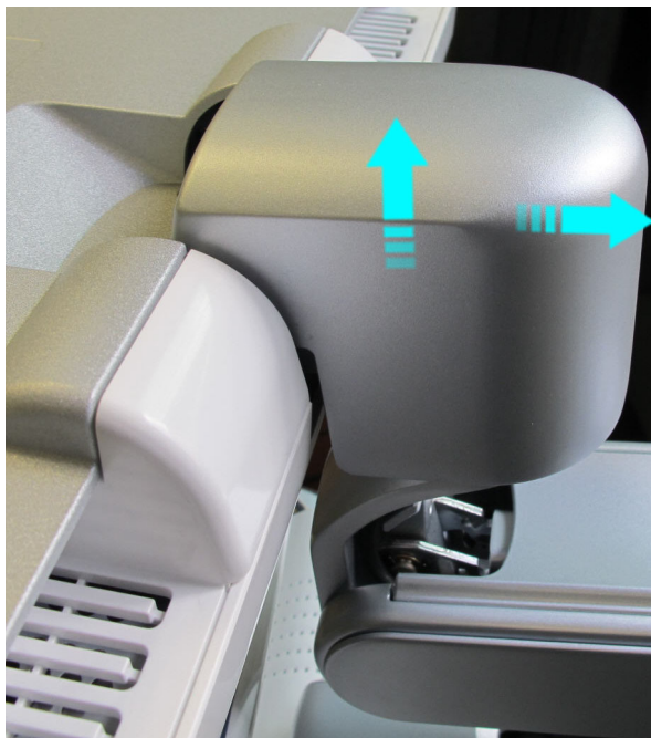
Figure 8-221 Removing Upper Articulated Arm Cover
