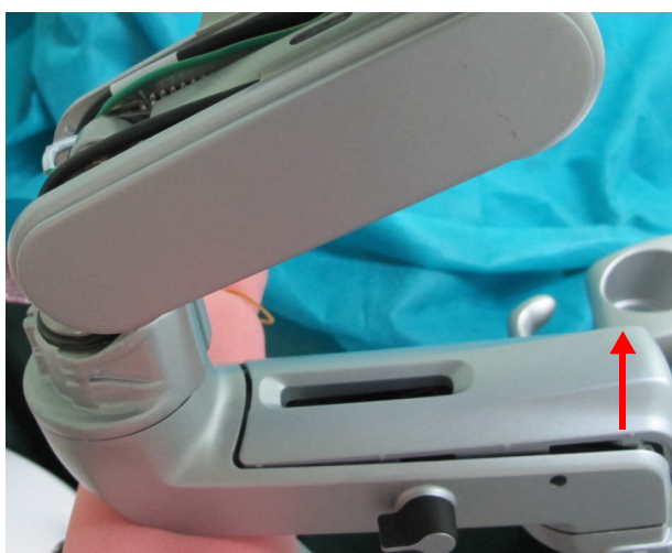
Figure 8-60 Removing Lower Horizontal Articulated Arm Cover
