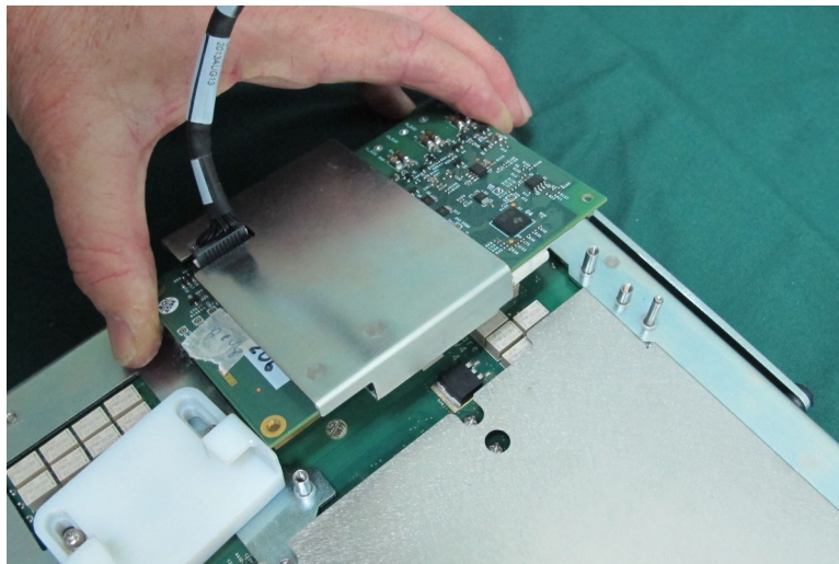
Figure 8-161 Removing the ECG Respiratory Module Assembly
