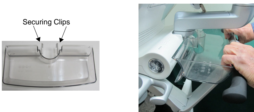
Figure 8-24 Removing the OPIO Basket
