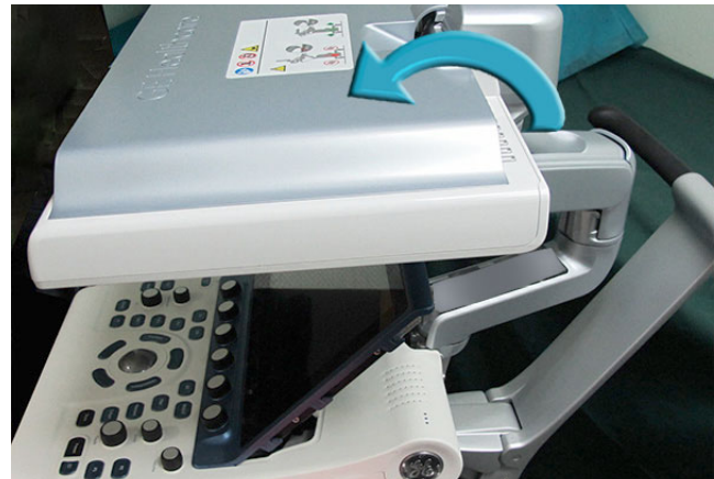
Figure 8-34 Folding Monitor Face-Down
