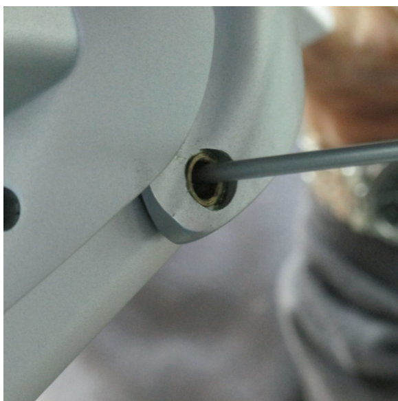
Figure 8-107 Remove Securing Pin
