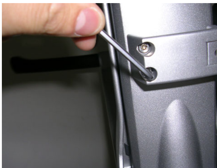
Figure 8-271 Removing the Cable Holder Bracket from the Support Arm
