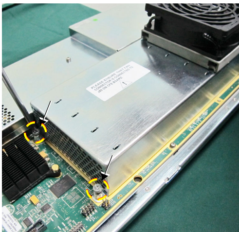
Figure 8-168 Opening the Metal Cover of the TRX32 Box
