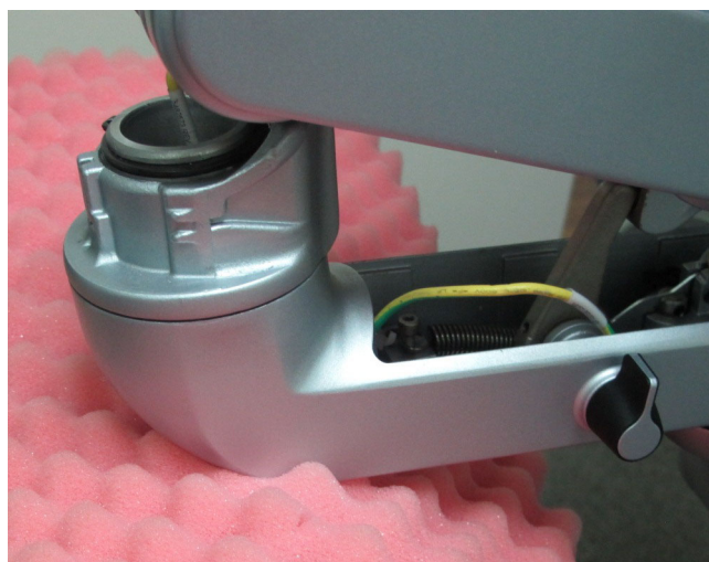
Figure 8-105 Protective Sponge Between Articulated Arm and System Handle
