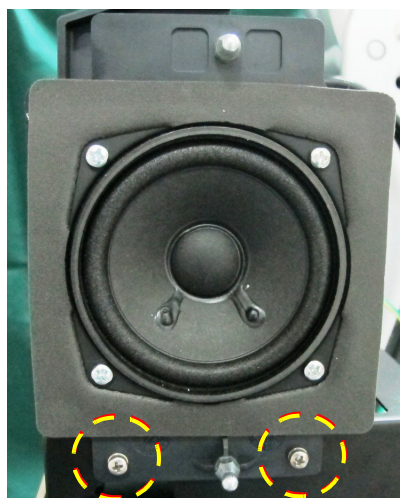
Figure 8-193 Loosening the Securing Screws
