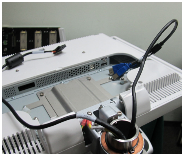
Figure 8-103 Monitor Cables Threaded Through Arm Aperture
