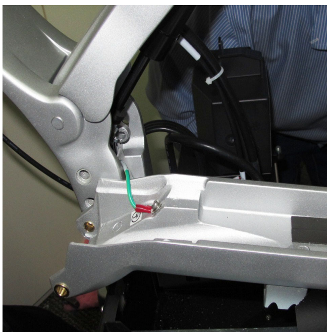
Figure 8-111 Lower Arm Cover Removed from System
