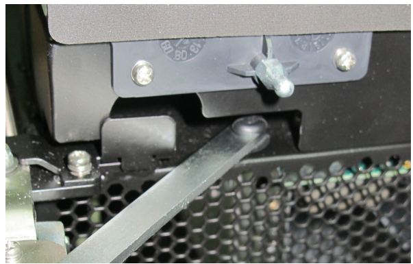
Figure 8-135 Securing the Cage Door with the Securing Arm
