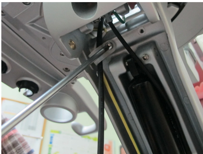
Figure 8-114 Cable Holder on Upper Section of Lower Arm Cover
