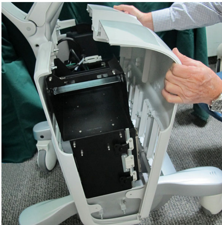
Figure 8-14 Removing the Front Cover
