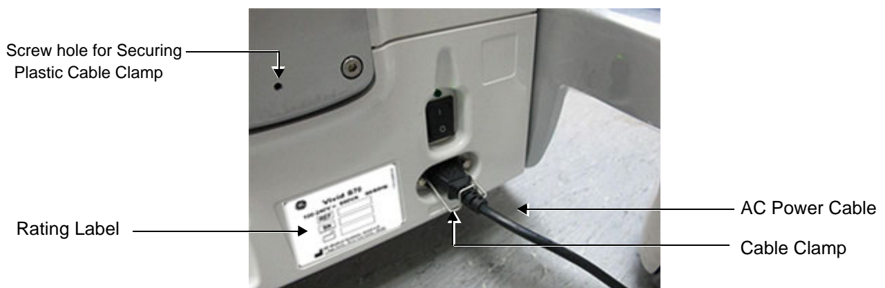
Figure 4-2 AC Power Cable Connected - Rear Panel
