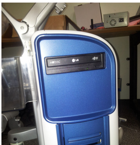
Figure 8-6 Removing the DVD Cover
