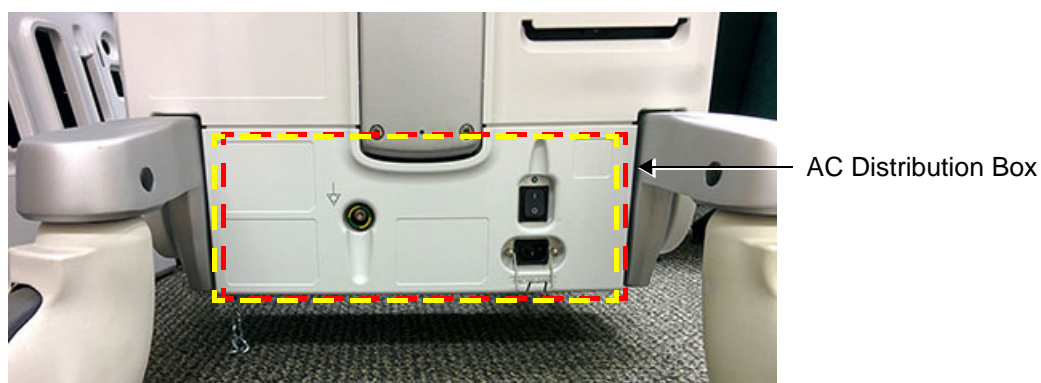
Figure 8-197 AC Distribution Box Located at Rear of System
