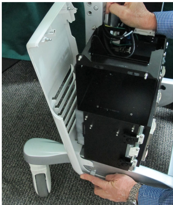
Figure 8-19 Removing the Right Rear Cover
