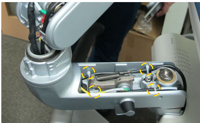
Figure 8-228 Four Tie-wraps on Lower Articulated Arm
