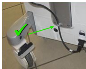
Figure 8-275 AC Power Cable Connected and Routed
