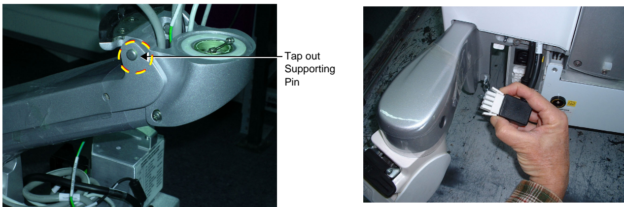
Figure 8-252 Removing the Joint Assembly
