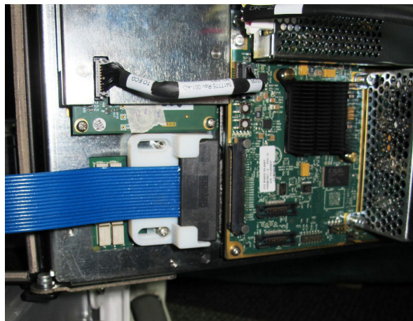
Figure 8-137 Releasing the Retaining Bracket on the CFE
