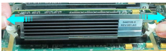
Figure 8-170 Removing a TRX32 Board
