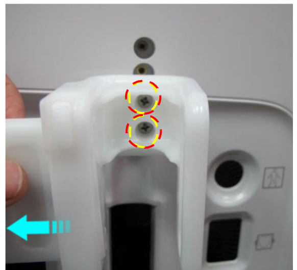
Figure 8-12 Removing the RS Cable Assembly - Front Part
