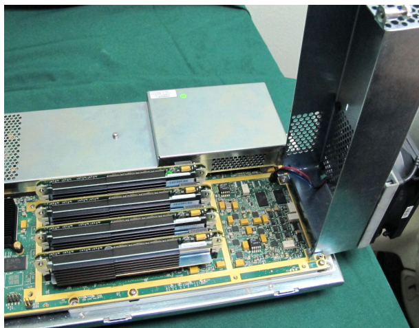
Figure 8-168 Opening the Metal Cover of the TRX32 Box
