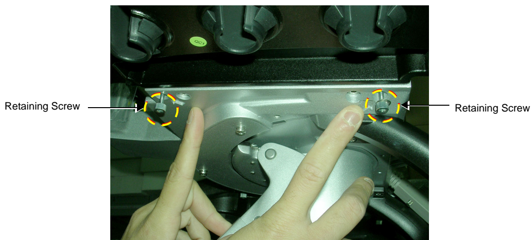
Figure 8-270 Probe Shelf - Viewed from Below indicating Retaining Screws
