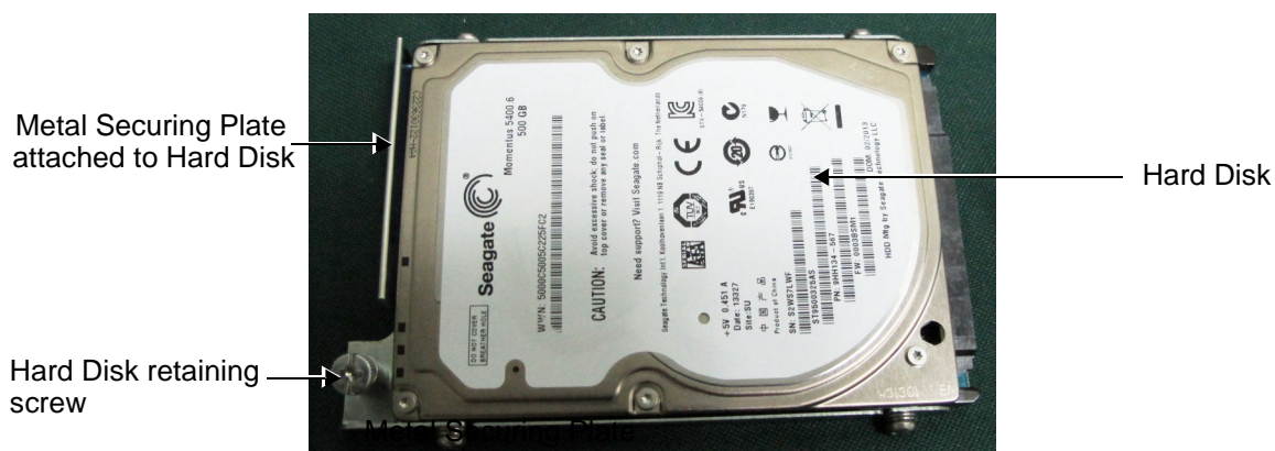
Figure 8-144 Hard Disk with Metal Securing Plate Attached
