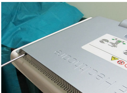
Figure 8-35 Removing Screws from Top of Service Cover
