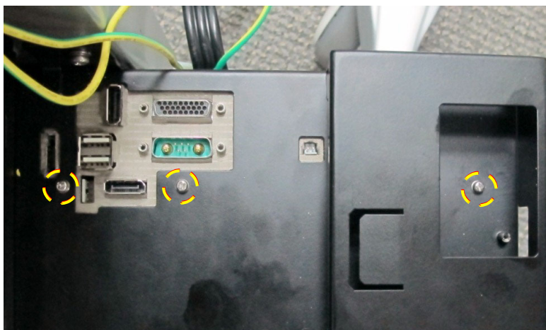
Figure 8-181 BIF Board Securing Screws Located on Top of Cabinet
