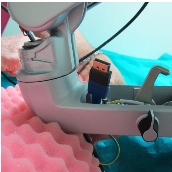
Figure 8-121 Feeding Cables through OPIO Aperture
