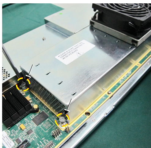
Figure 8-183 Opening the Metal Cover of the TRX32 Box
