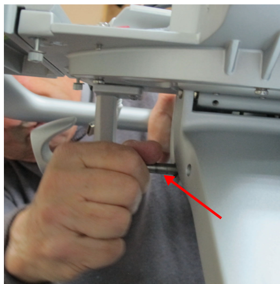
Figure 8-107 Remove Securing Pin
