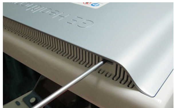
Figure 8-35 Removing Screws from Top of Service Cover
