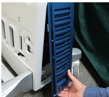
Figure 8-3 Removing the Air Inlet (Left Side) Cover
