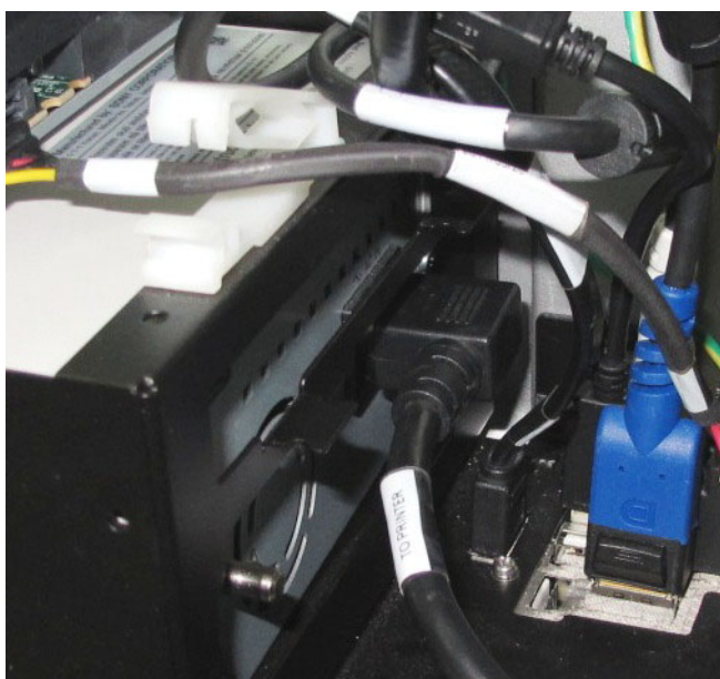
Figure 8-129 Peripheral Power Output Cable (Printer-to-AC Box)
