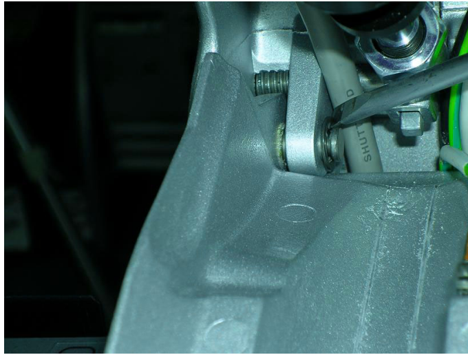
Figure 8-245 Removing Left Securing Clip from Securing Pin
