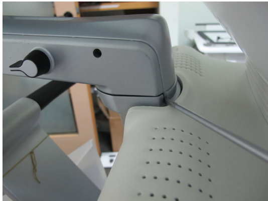
Figure 8-61 Removing the Monitor Arm Base Cover
