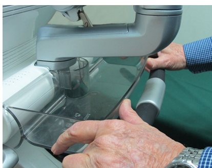
Figure 8-25 Installing the OPIO Basket
