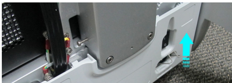
Figure 8-29 Removing the AC Distribution Box Cover
