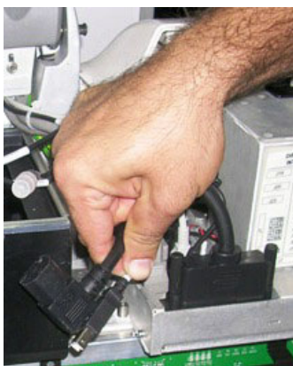
Figure 8-283 Cables Disconnected from Rear of Black and White Printer
