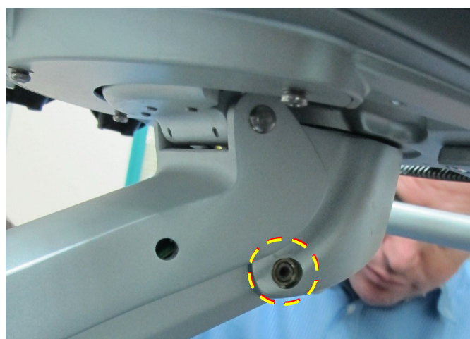
Figure 8-106 Lower Arm Securing Screws
