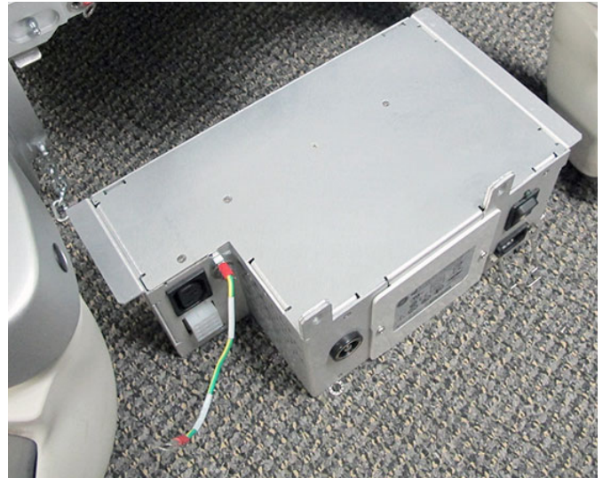
Figure 8-201 Removing the AC Distribution Box
