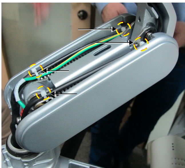
Figure 8-101 Cutting Tie-wraps on the Articulated Arm
