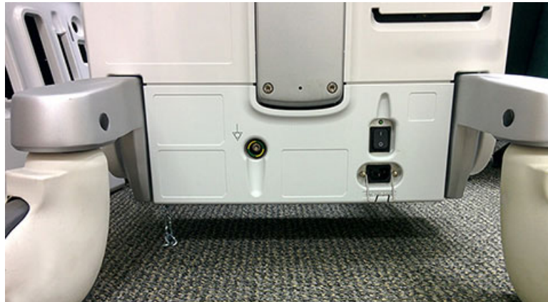
Figure 8-31 AC Distribution Box Cover Installed
