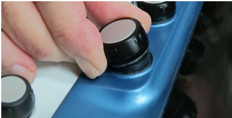
Figure 8-95 Removing a Rotary Knob
