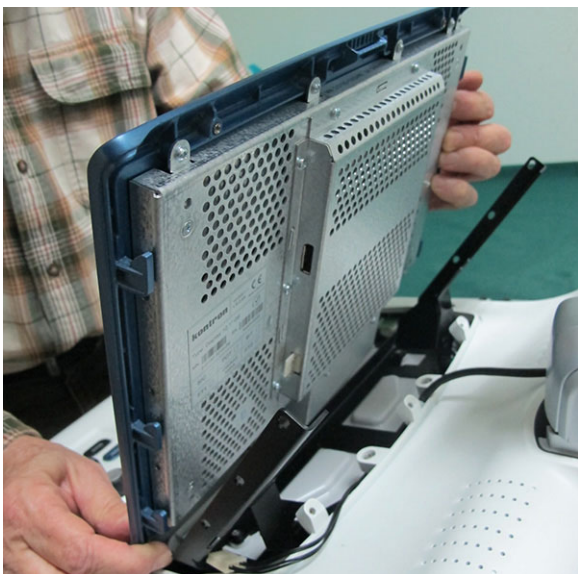
Figure 8-72 Removing the Touch Screen
