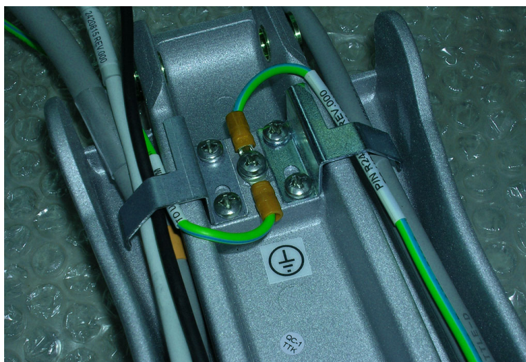
Figure 8-241 Positioning of Cable in Upper Arm
