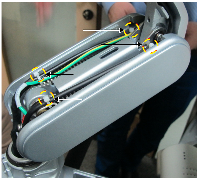
Figure 8-227 Cutting Tie-wraps on the Articulated Arm
