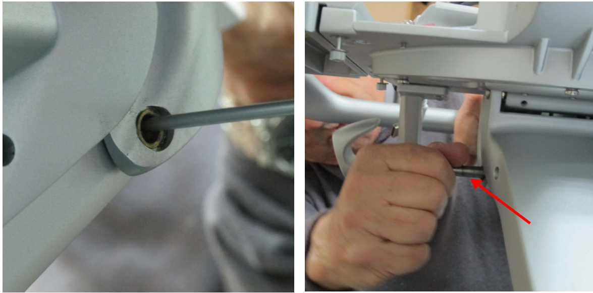
Figure 8-243 Remove Securing Pin
