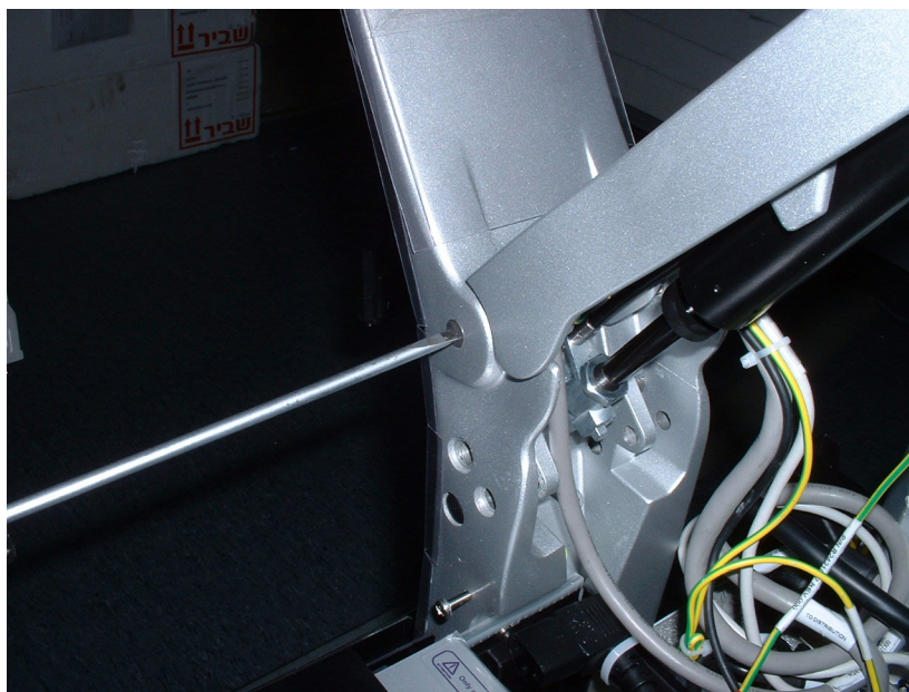
Figure 8-240 Tapping Out the Upper Arm Support Pin
