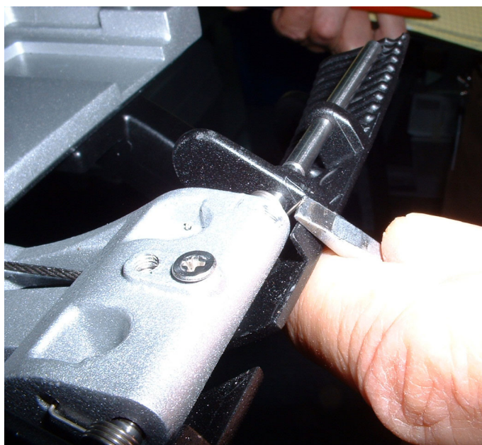
Figure 8-236 Releasing Spring that Presses on the Handle
