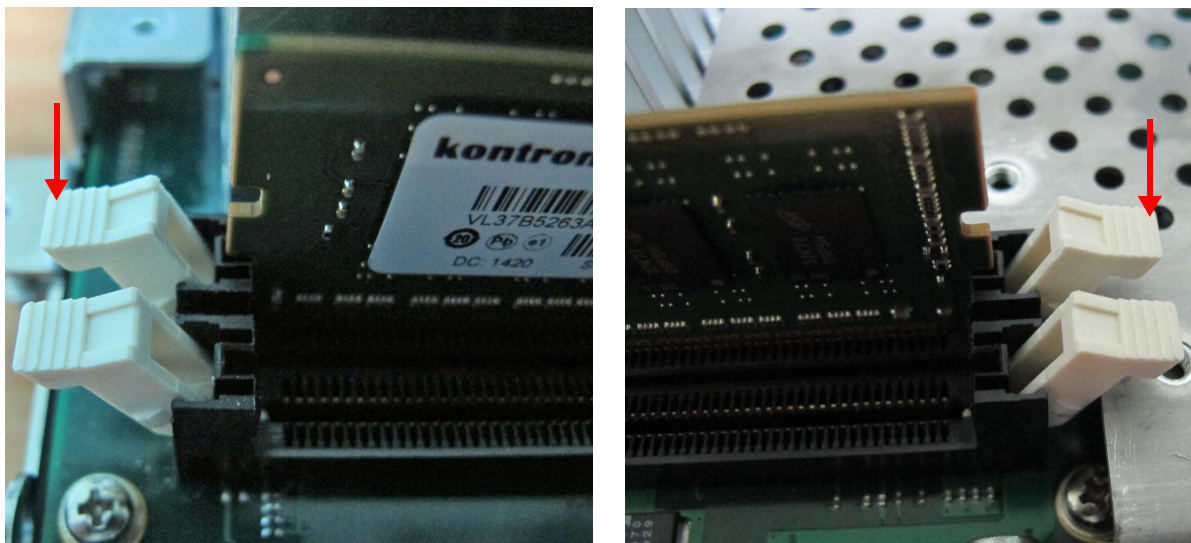
Figure 8-156 Removing the Module Memory DDR Circuit Boards
