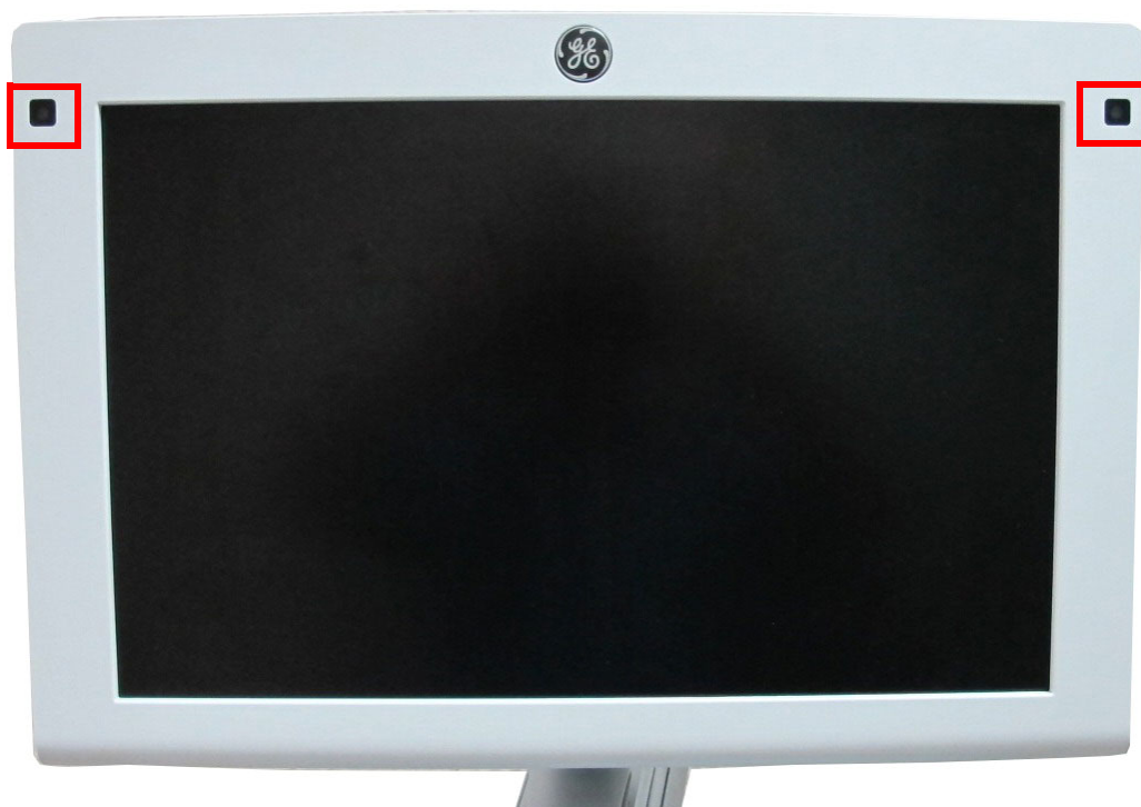
Figure 8-55 Location of Monitor Light Sensors on Monitor Front Panel
