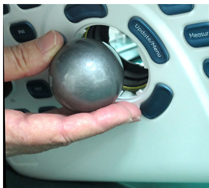
Figure 8-92 Removing the Mechanical Trackball
