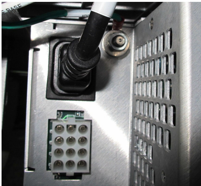
Figure 8-130 Printer Cable Plugged into AC Distribution Box
