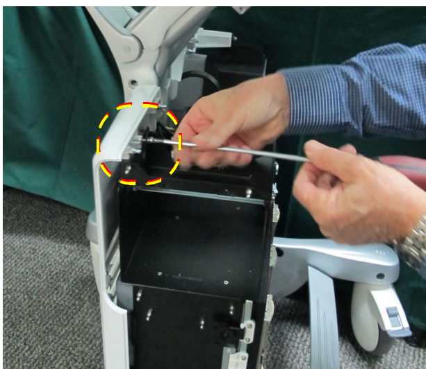
Figure 8-17 Right Rear Cover - Removing Securing Screws
