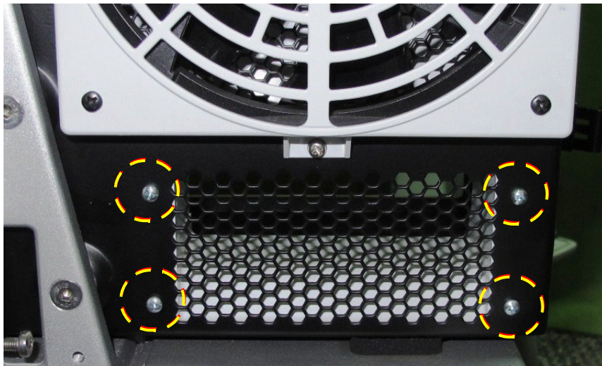
Figure 8-174 Plastic Air Sleeve Securing Screws (rear of Scanner)
