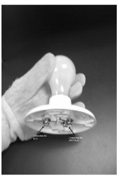
The picture shows an incandescent bulb with connecting plate. This bulb is used to ensure that wall power terminal provides a proper ground connection.
