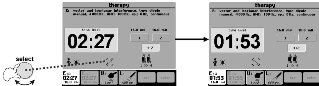
When rotating dipole, the unit automatically switches to diagnostic mode (Spectrum value = 0Hz). After 1 or 2 seconds the unit returns to therapeutic mode (Spectrum value = preset value).
