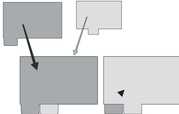
If more accessories are connected to one generator (e.g. two ultrasound heads connected to a single ultrasound generator), pressing the channel tab of the generator will switch between accessories.
