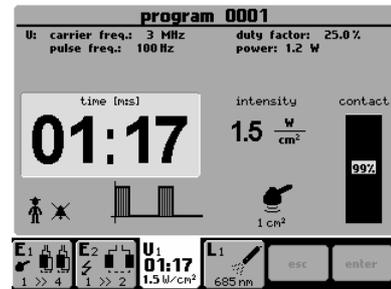
Insufficient contact between the ultrasound head and the tissue is indicated rapid blinking of the blue light ring on the head and blinking of the information on intensity and time on the channel tab of the corresponding ultrasound generator. This function is indicated by a figure symbol on the screen.
