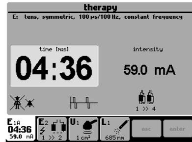
Disconnection of electric circuit (such as in case of wrong contact between electrode and patient) is indicated by blinking information about intensity and time on the corresponding channel tab, or by audio signalling.
