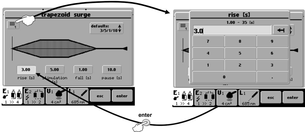
Set numerical values of the parameter that has been selected - “white” button on the picture above. Enter the value and press **enter (15)** to return to original screen. Press **esc (16)** to exit the screen. If you set the value that exceeds the allowed value range (allowed value range is stated on top of the screen), or if the unit cannot set the required value, the value will be rounded as close as possible to the allowed value.
