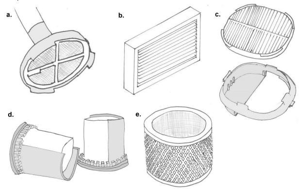
a. disc filter, common in suction machines, b. flat panel filter, common in incubators or ventilation systems, c. flat filter, shown with housing beneath, d. round sponge filter, common in nebulizers, e. cylindrical filter, common in engines and compressors.
