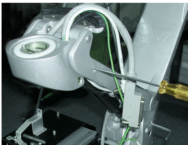
Figure 8-197 Supporting the Upper Gas Spring Bracket with a Screwdriver
