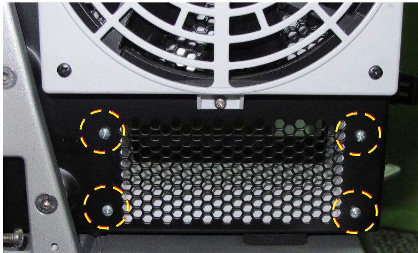
Figure 8-144 Plastic Air Sleeve Securing Screws (rear of Scanner)
