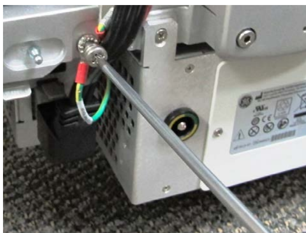
Figure 8-168 Disconnecting the Ground Cable
