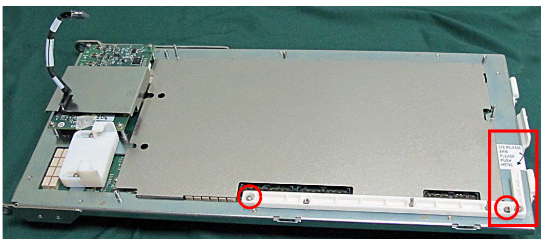
Figure 8-142 Location of CFE Release Arm
