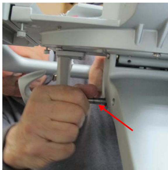
Figure 8-79 Remove Securing Pin
