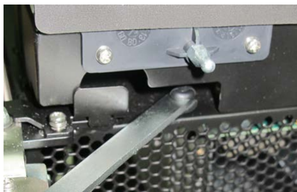
Figure 8-105 Securing the Cage Door with the Securing Arm
