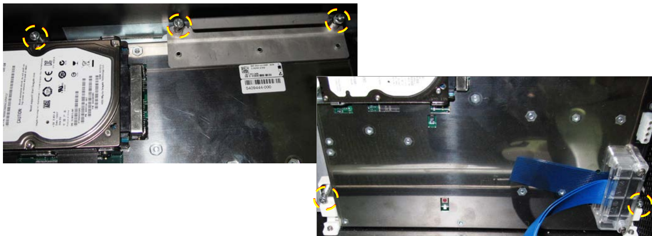
Figure 8-119 BEP Securing Screws
