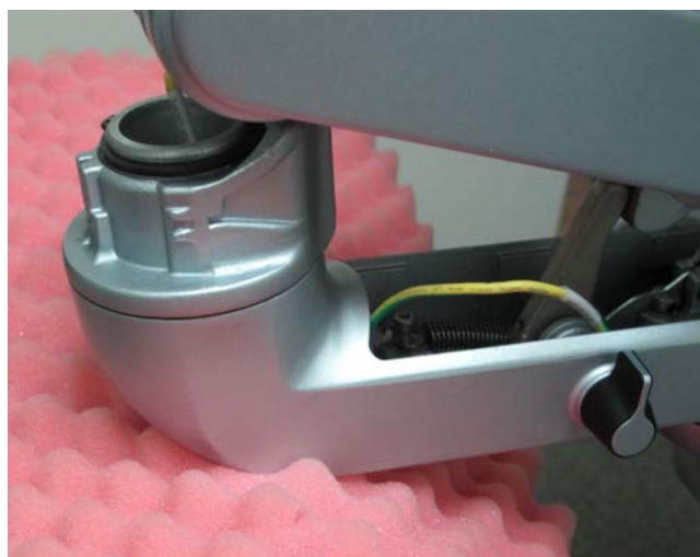
Figure 8-77 Protective Sponge Between Articulated Arm and System Handle
