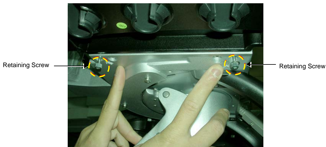
Figure 8-201 Probe Shelf - Viewed from Below indicating Retaining Screws
