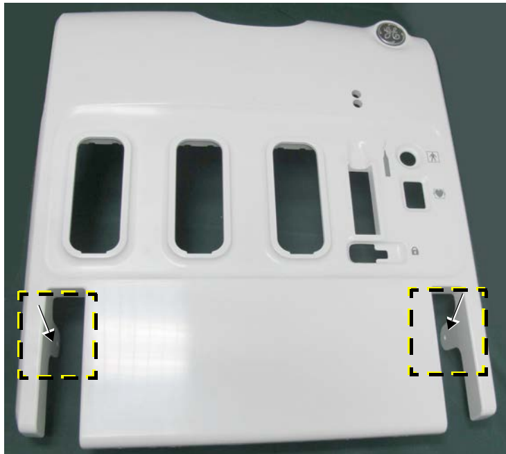
Figure 8-10 Front Cover - Securing Tabs
