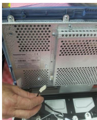
Figure 8-46 Routing and Connecting the Touch Screen Cables
