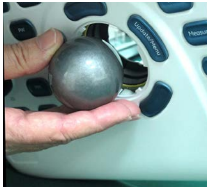
Figure 8-64 Removing the Mechanical Trackball
