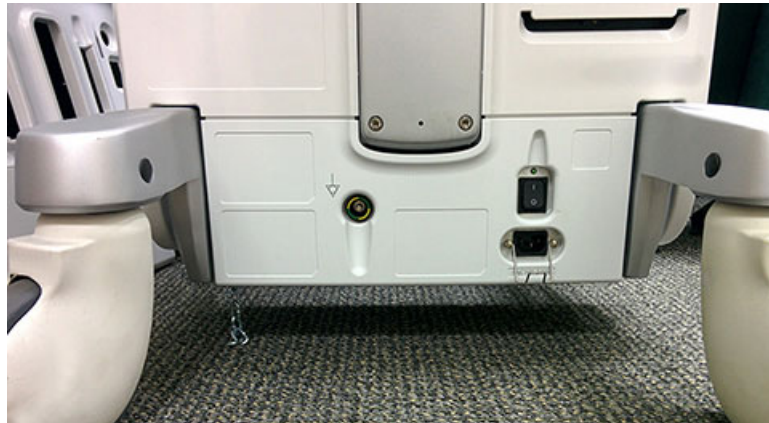
Figure 8-31 AC Distribution Box Cover Installed
