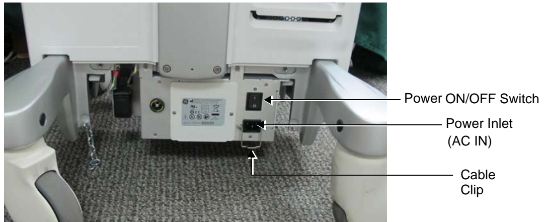
Figure 4-1 Power ON/OFF Switch and Power (AC IN) Socket - Rear Panel
