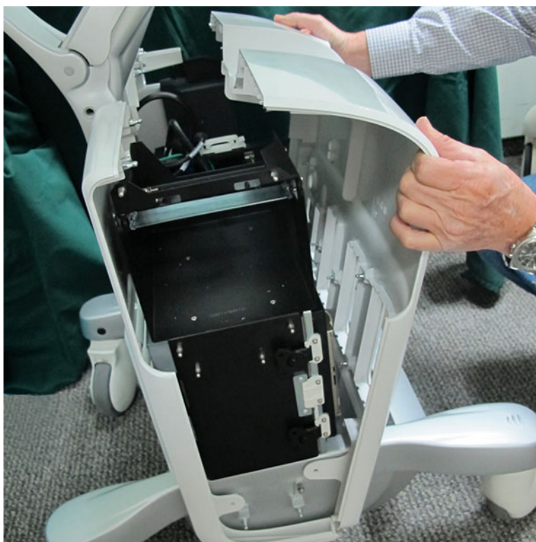
Figure 8-14 Removing the Front Cover
