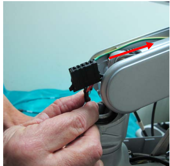
Figure 8-94 Threading the Display to OPIO Cable
