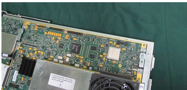
Figure 8-134 Front End Power Supply Removed
