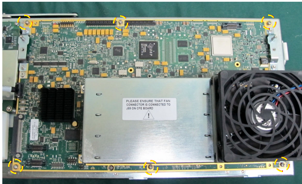
Figure 8-136 CFE Board showing 6 Retaining Screws
