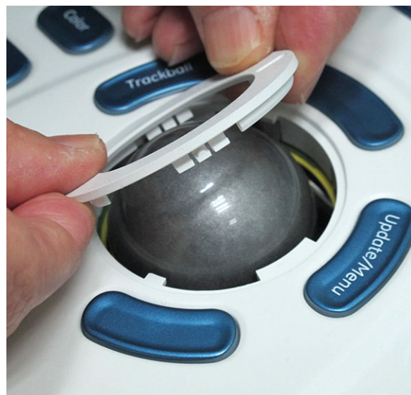
Figure 8-63 Removing the Mechanical Trackball Ring
