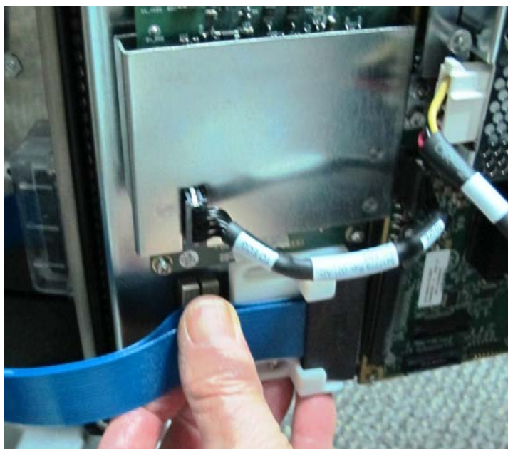
Figure 8-108 Releasing the HDR flat cable from the CFE
