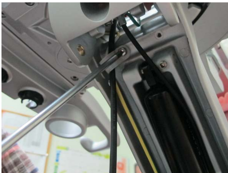
Figure 8-86 Cable Holder on Upper Section of Lower Arm Cover
