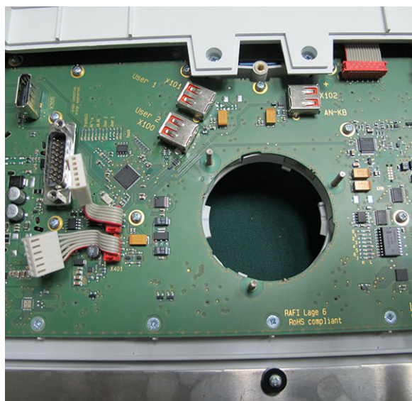
Figure 8-66 Trackball Board and Housing Removed
