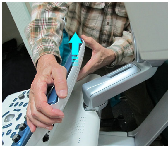
Figure 8-39 Removing the Touch Screen Rear Cover
