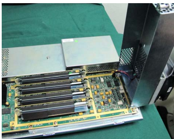
Figure 8-153 Opening the Metal Cover of the TRX32 Box
