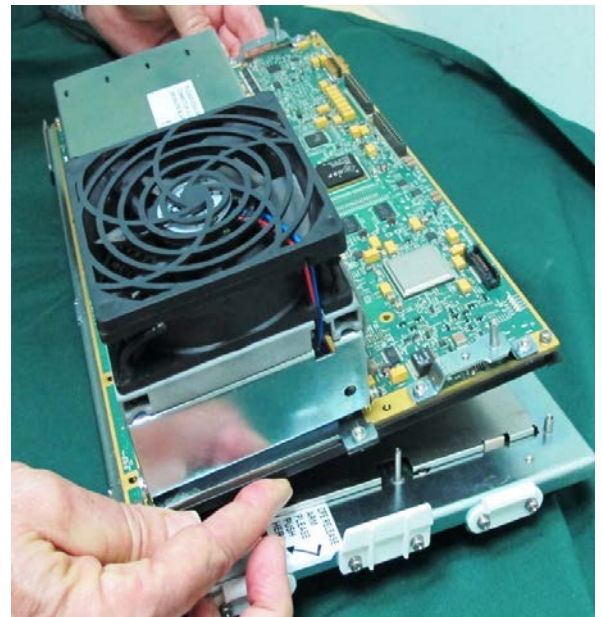
Figure 8-137 CFE Release Lever and Release of CFE Board
