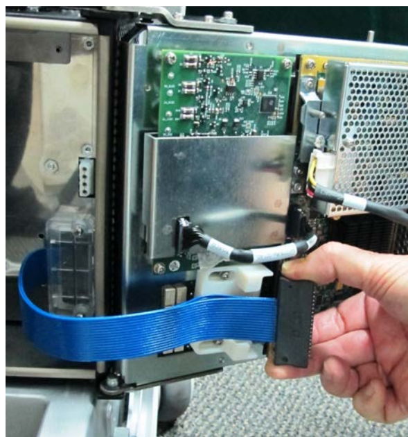
Figure 8-108 Releasing the HDR flat cable from the CFE
