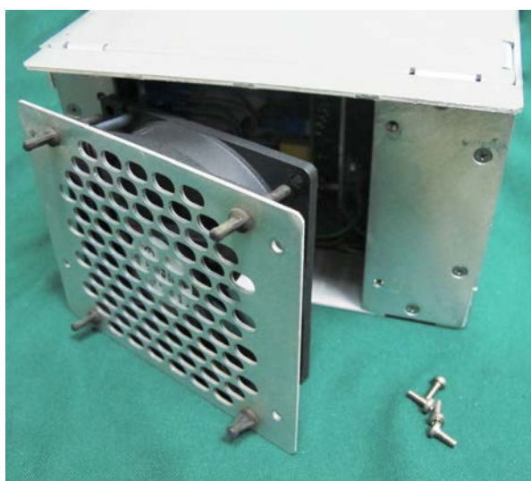
Figure 8-174 Disconnect the Fan Cable from the AC Distribution Box
