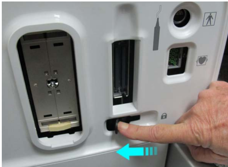
Figure 8-11 RS Probe Connector Lock - OPEN
