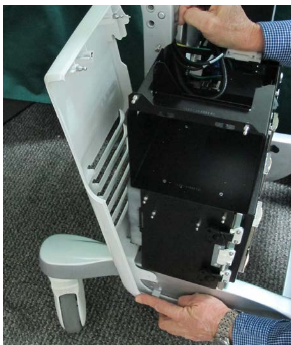
Figure 8-19 Removing the Right Rear Cover
