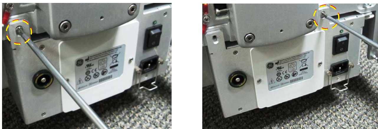
Figure 8-170 AC Box Supporting Screws
