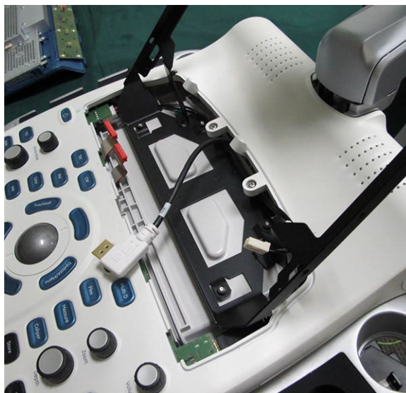
Figure 8-44 Removing the Touch Screen
