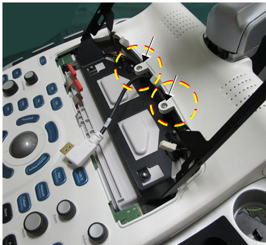
Figure 8-179 Removing Securing Screws
