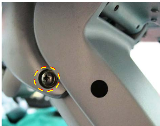
Figure 8-78 Lower Arm Securing Screws
