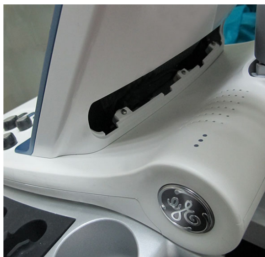
Figure 8-35 Removing the Touch Screen Service Cover
