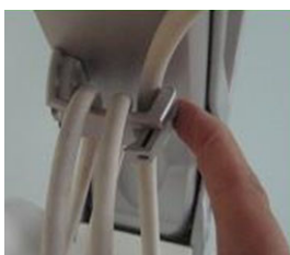
Figure 8-204 Opening the Cable Gate on Probe Cable Holder
