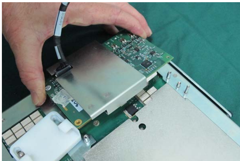
Figure 8-131 Removing the ECG Respiratory Module Assembly
