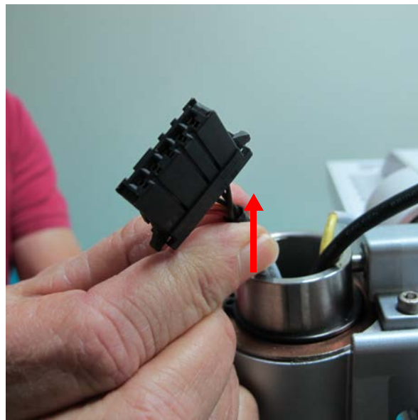
Figure 8-95 Threading the Display to OPIO Cable
