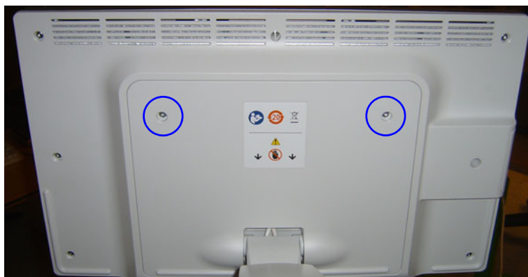
Figure 8-32 Monitor Rear Cover's fixing screws
