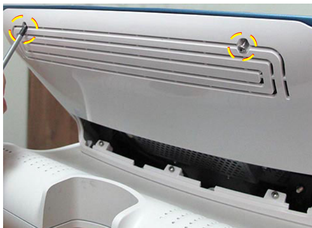
Figure 8-38 Removing the Rear Cover (Top) Securing Screws
