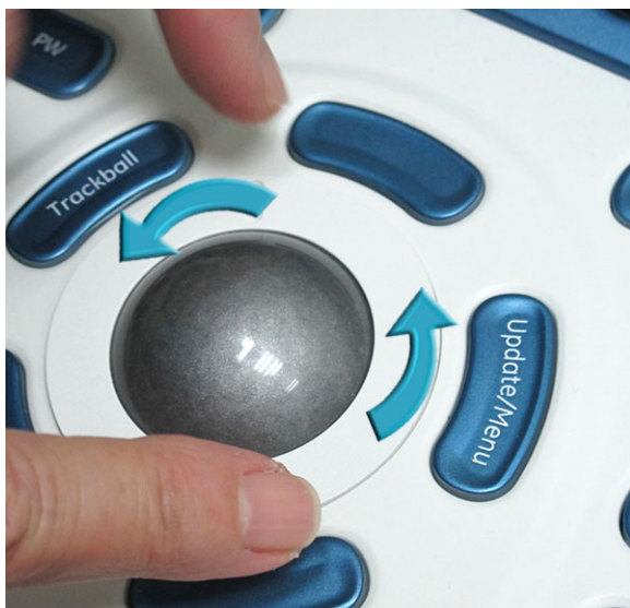
Figure 8-63 Removing the Mechanical Trackball Ring
