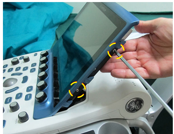
Figure 8-40 Removing the Touch Screen Securing Screws
