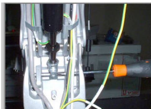
Figure 8-196 Tapping out the Lower Support Pin using a Punch
