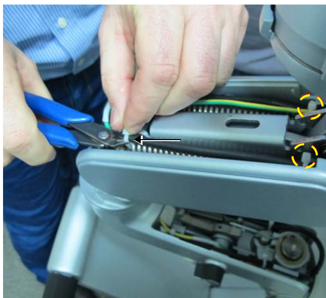
Figure 8-73 Cutting Tie-wraps on the Articulated Arm
