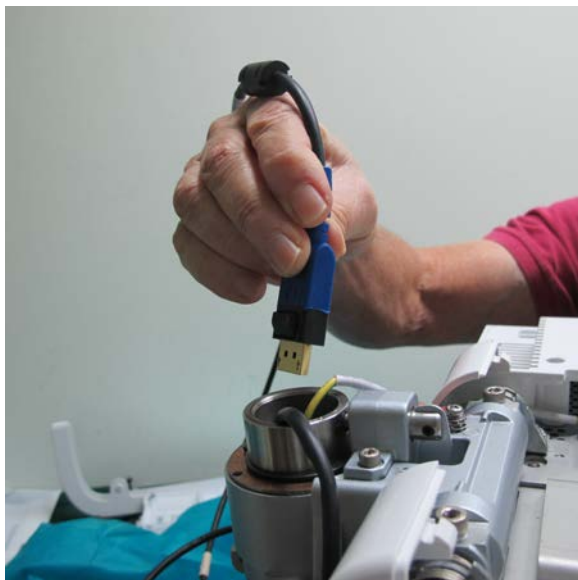
Figure 8-92 Feeding Cables through Top Aperture
