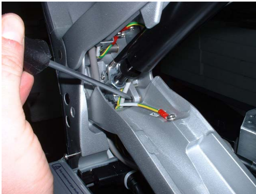
Figure 8-82 Tapping Out the Securing Pin
