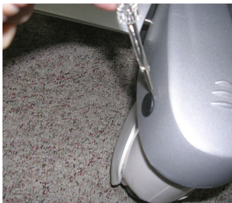
Figure 8-208 Removing the Screw Cap
