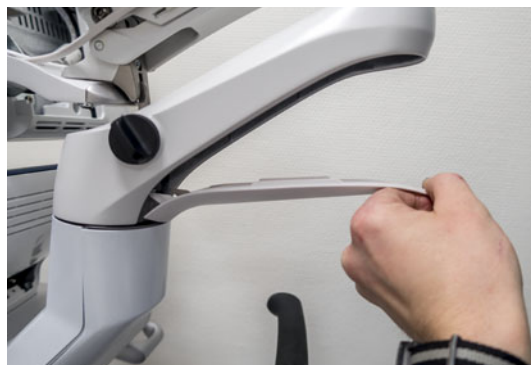
Figure 8-183 Remove the Lower Service Cover
