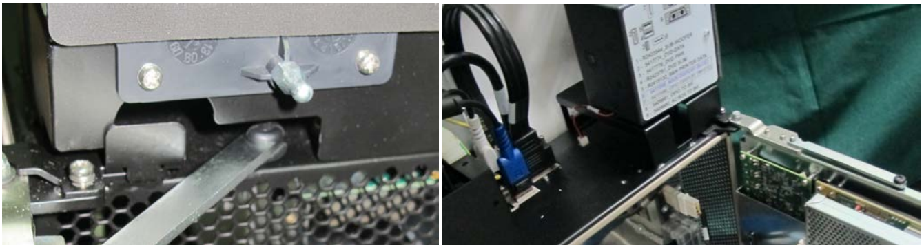
Figure 8-109 Releasing Cage Supporting Arm from Device Chassis
