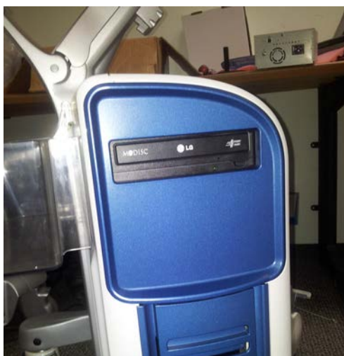
Figure 8-6 Removing the DVD Cover
