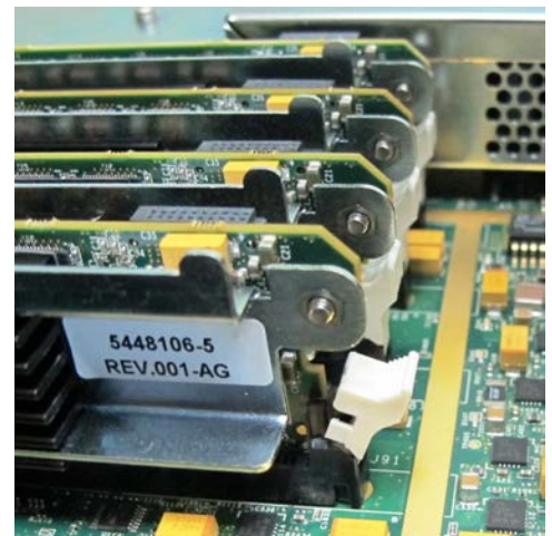
Figure 8-139 TRX32 Boards Secured with Plastic Holders
