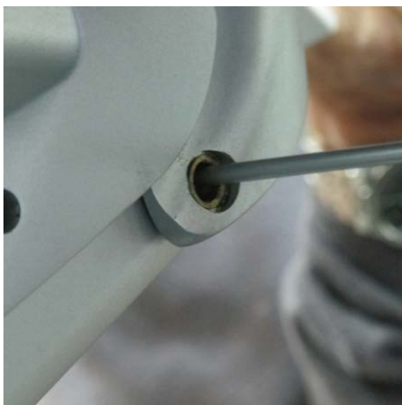
Figure 8-79 Remove Securing Pin
