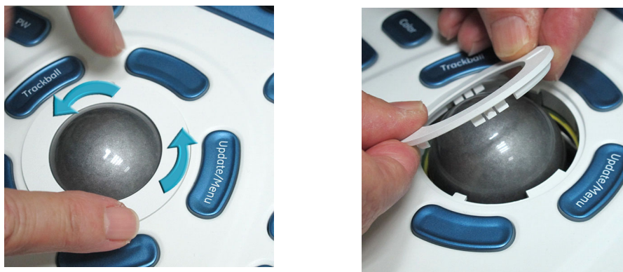
Figure 4-11 Removing Top Locking Plate and Rubber Dust Filter Ring
