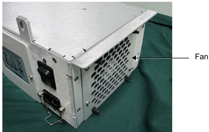
Figure 8-172 AC Distribution Box Fan - Location
