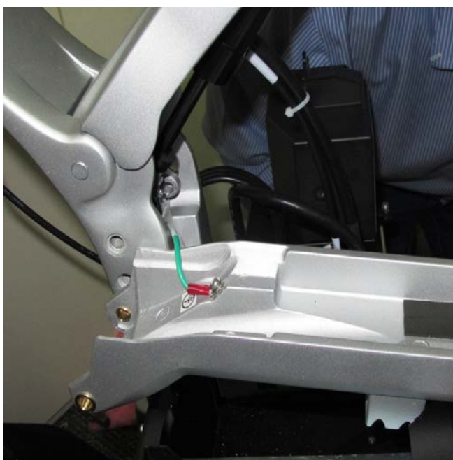
Figure 8-83 Lower Arm Cover Removed from System
