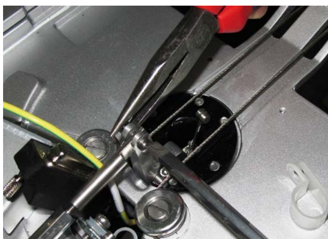
Figure 8-87 Releasing Up-Down Lever Shaft
