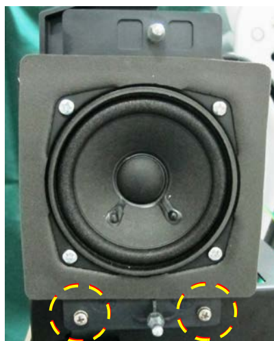
Figure 8-163 Loosening the Securing Screws
