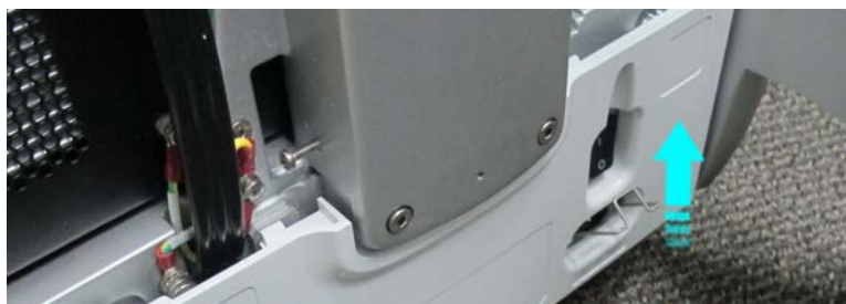
Figure 8-29 Removing the AC Distribution Box Cover
