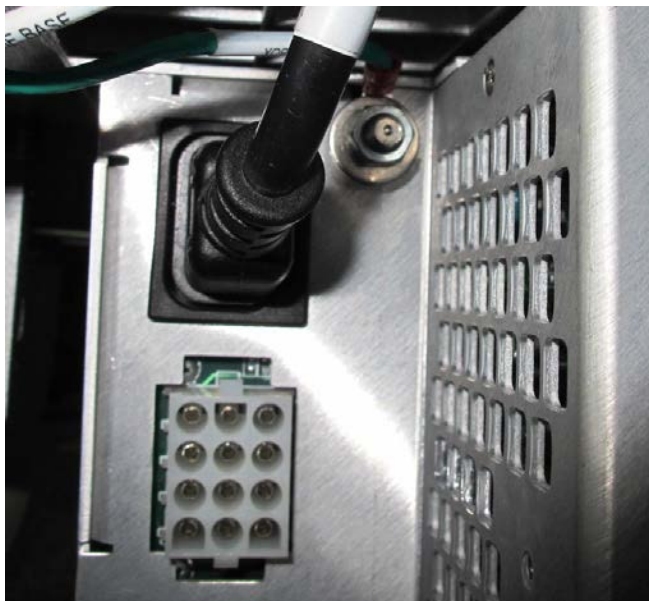
Figure 8-100 Printer Cable Plugged into AC Distribution Box
