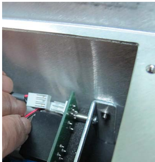
Figure 8-174 Disconnect the Fan Cable from the AC Distribution Box
