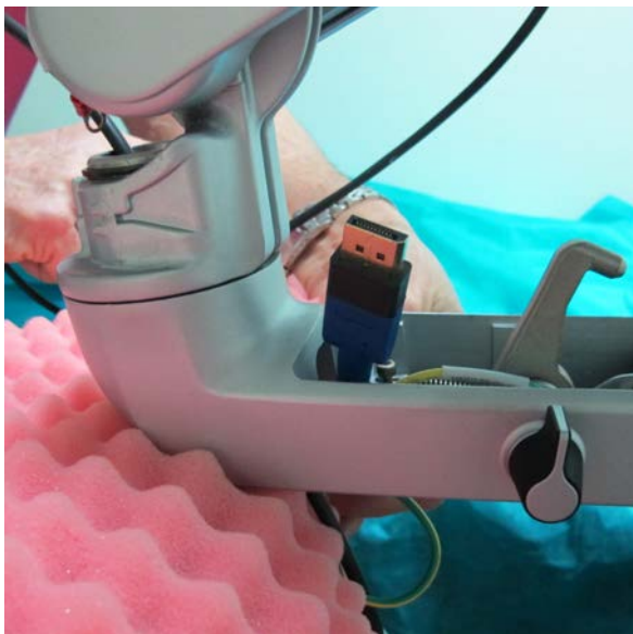
Figure 8-93 Feeding Cables through OPIO Aperture
