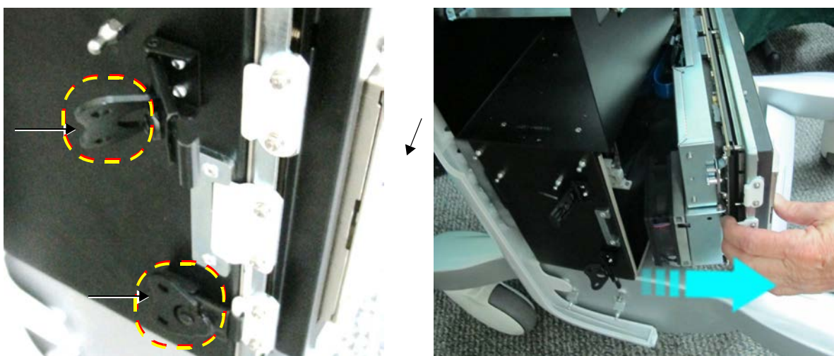
Figure 8-104 Unfastening the Latches and Opening the Cage Door
