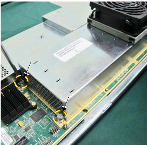
Figure 8-138 Opening the Metal Cover of the TRX32 Box
