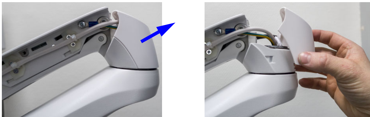
Figure 8-182 Remove the Vertical Service Cover
