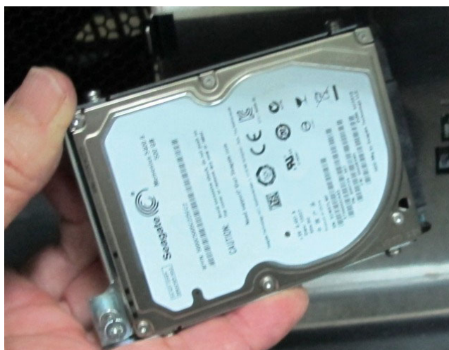
Figure 8-116 Removing the Hard Disk
