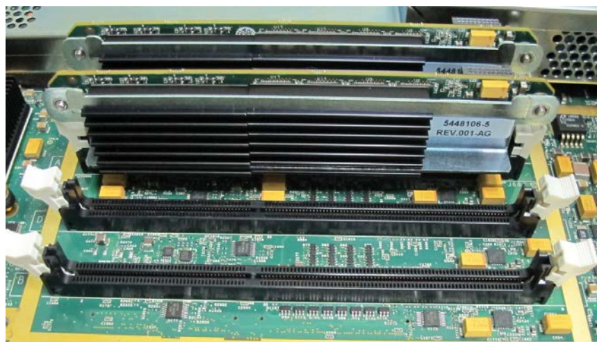
Figure 8-157 TR32X Grooves and Holders on the CFE Board
