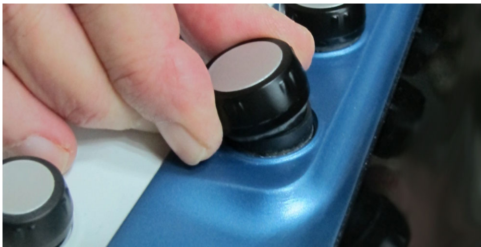
Figure 8-67 Removing a Rotary Knob
