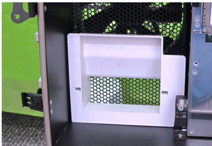
Figure 8-143 Location of Plastic Air Sleeve for CFE
