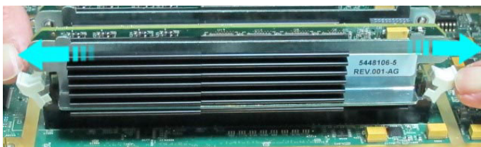
Figure 8-140 Removing a TRX32 Board
