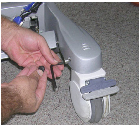
Figure 8-209 Removing the Securing Screw
