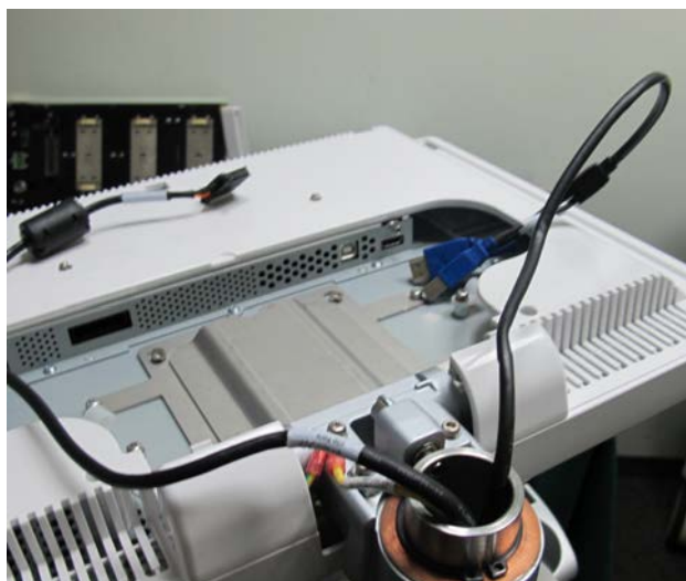
Figure 8-75 Monitor Cables Threaded Through Arm Aperture
