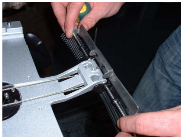
Figure 8-189 Protective Metal Plate Rotated 90 Degrees
