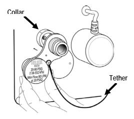
Figure 2–28: Attaching the Tethered Heliox Connector
