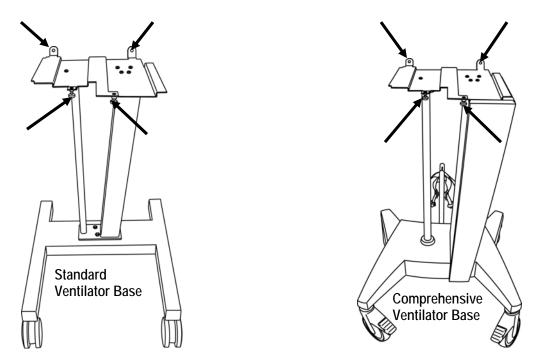
Figure 2-1: Basic and Comprehensive base attachment
