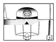
Figure 2-12: Completed installation of Filter / Water Trap combination
