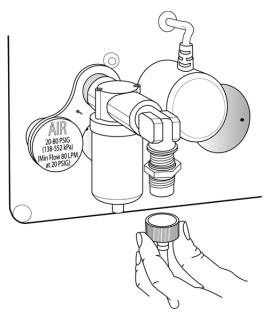
Attach the Air supply hose to the "Smart" connector fitting with the integral water trap/filter on the left of the back panel as shown in Figure 2–31.
