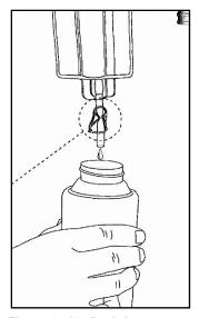
Figure 2-13: Draining water trap
