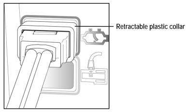
Figure 2–21: Variable Orifice Flow Sensor Attachment
