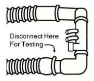
Figure 6-3: Disconnect Point for Calibration
