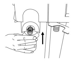
Figure 2–7: Insert exhalation filter
