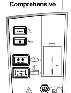
Figure 2–19: AVEA Front Panel Configurations Standard and Comprehensive
