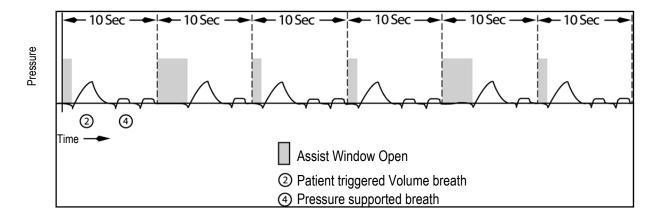
Figure 3-14: SIMV Waveform
