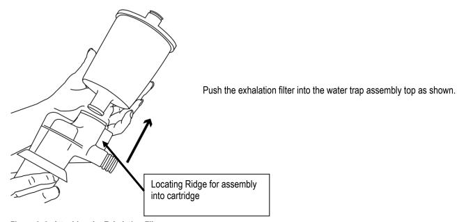
Figure 2-3: Attaching the Exhalation Filter
