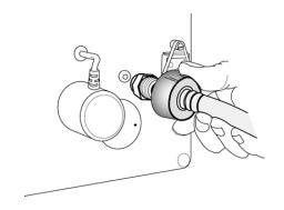
Figure 2-29: Connecting the O2 Hose
