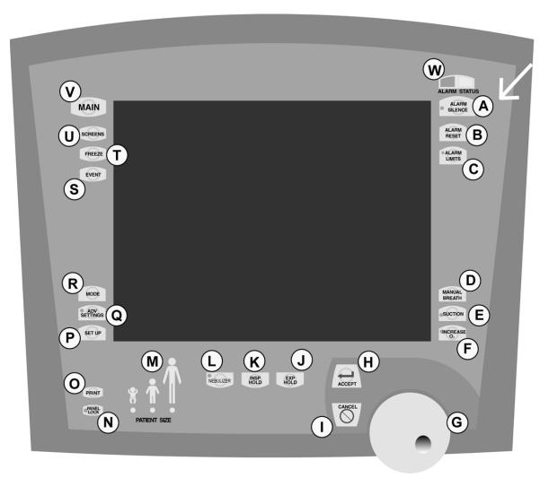
Figure 3.1b User Interface Module (English) Showing Button Labels
