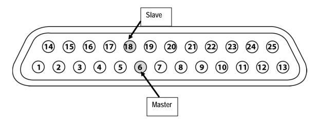
Figure 2–33: ILV Connection Pin Configuration
