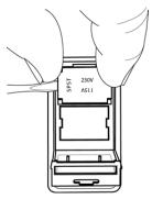
4. The fuse holder contains two fuses, 3.1 amps (for 100/120 volt lines) and 2.0 amps (for 230/240 volt lines) as shown in Table 8–1.
