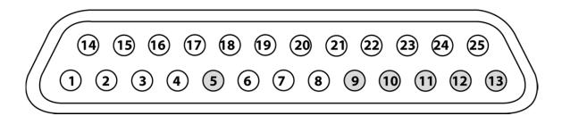
Figure 2-34: Analog Ground Pins
