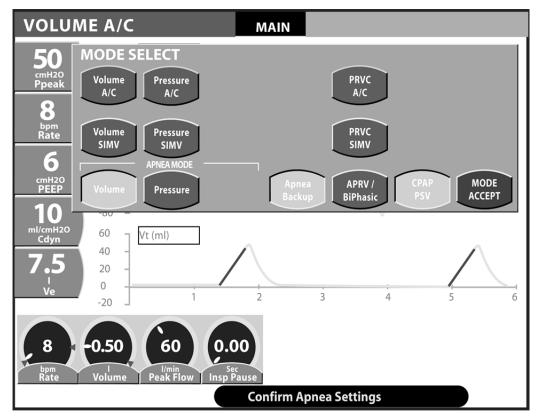
Figure 3-20: Volume Apnea Backup settings for CPAP Mode
