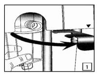
Figure 2–10: Inserting the Filter / Water Trap combination
