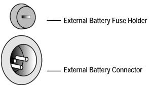
Figure 8-3: External Battery Connector and Fuse
