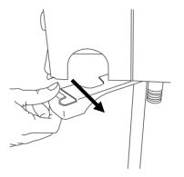
Figure 2-6: Open locking lever
