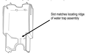
Figure 2-4: Exhalation Filter Cartridge Showing Locating Slot
