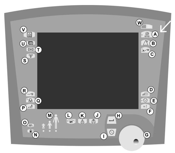
Figure 3.1a User Interface Module (International) Showing Button Icons
