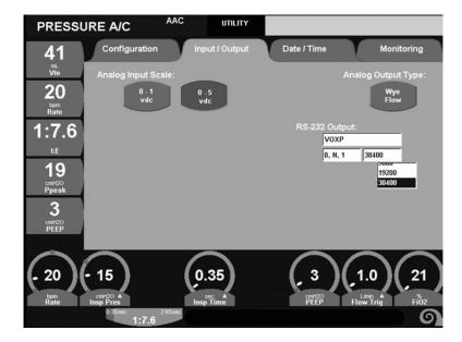
The ventilator has two RS-232 ports installed for bi-directional communication of data: RS-232 Ch1 is currently used for software updates as well as data communications to external systems.
