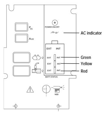
Figure 7–1: Front Panel Display Area. Comprehensive model shown.
