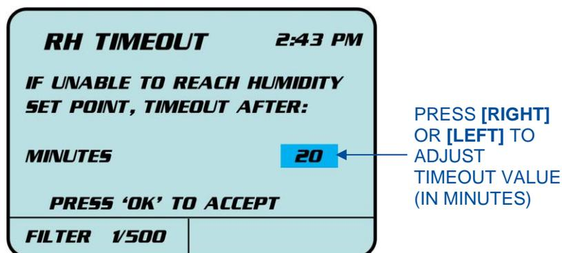
2. Press the **[RIGHT]** button to increase the timeout value in 5 minute increments, press **[OK]**.
