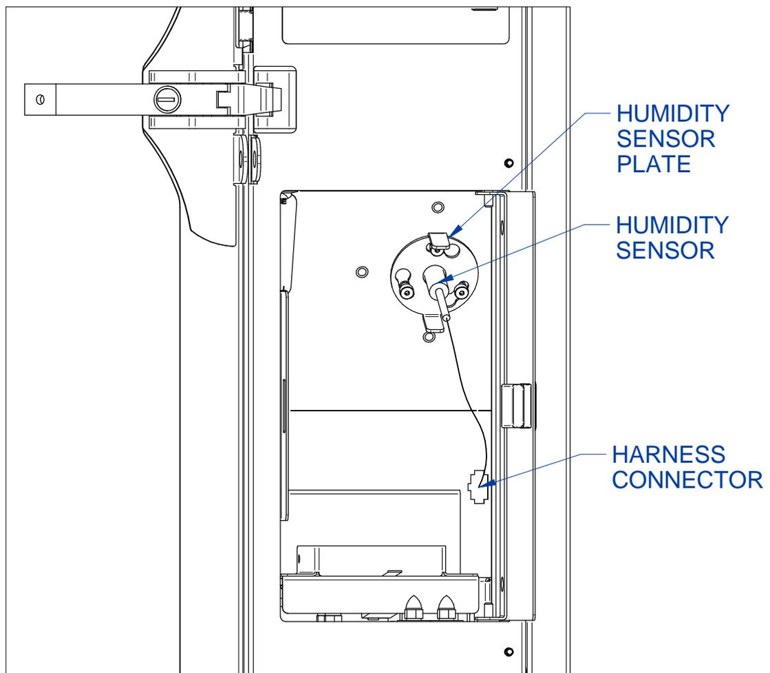
4. Disconnect the Harness Connector at the end of the Humidity Sensor from the thru-wall connector mate. To disconnect, press down on the small lever tab on the connector and pull the Harness Connector towards you.
