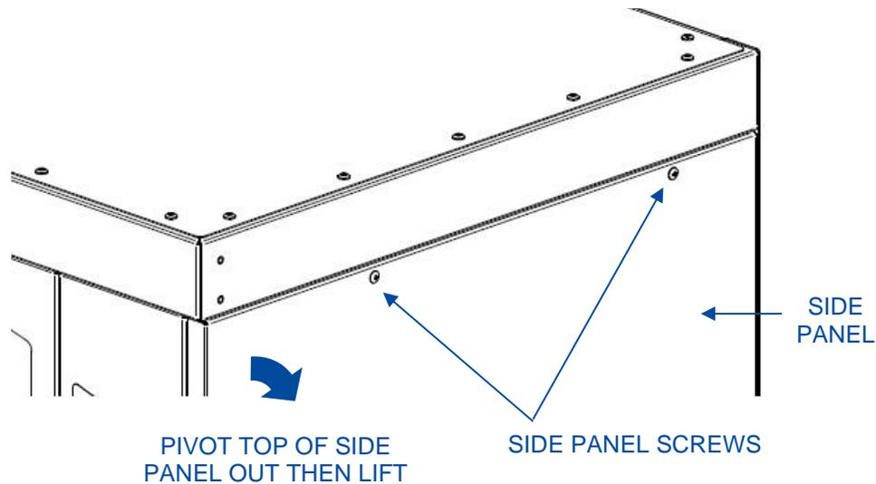
To remove the right Side Panel, locate and remove the two (2) Screws at the top of the right Side Panel. Pivot the top of the Side Panel away from the chamber. Then, lift Side Panel up to clear the pins at bottom of Side Panel from the holes in lower frame. See Fig. 7-15 above. Save the Screws and Side Panel for reassembly. **Note – Side Panel is heavy!** Lay the Side Panel flat while removed from the chamber, so it cannot fall over.
