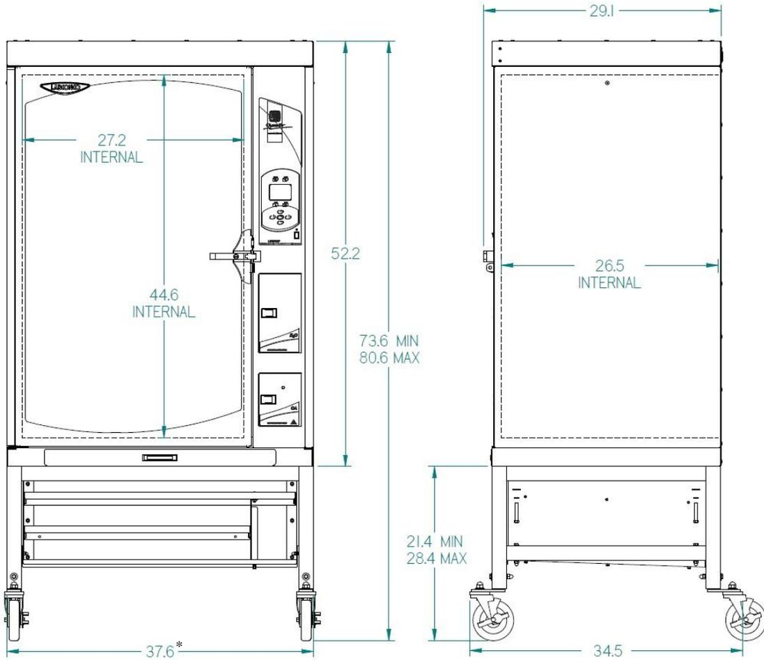
\*Locking Brake on Casters adds 1.0 inch to this dimensions.
