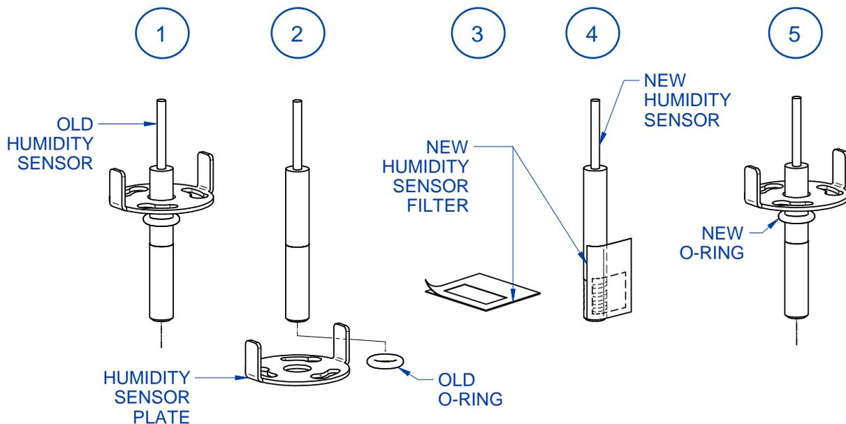
8. Identify the components inside the new Humidity Sensor Kit (P/N 3179230). The kit includes a new Sensor, Sensor Filter, and O-Ring.
