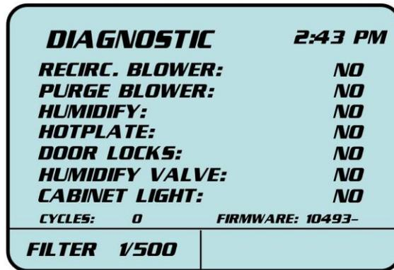
Use **[UP]** and **[DOWN]** to select a component to test, then press **[RIGHT]** to start the test. The **NO** next to that component will change to **YES** while active. Each component will activate for 30 seconds (when doors closed). The expected result for each component test is listed below:
