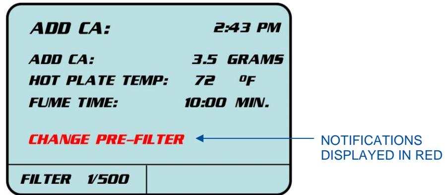
This is just a reminder notification, not an error or alert. Alerts are shown in the bottom right corner, and a Fuming Cycle cannot begin if an Alert is shown. If a notification is displayed, the Fuming Cycle will still begin when **[START]** is pressed.
