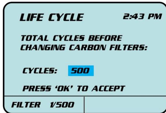
Using the UP/DOWN Buttons, adjust the Filter Life Cycle number as desired between 200 and 500 Cycles in 50 Cycle increments. Press **'OK'** to accept.
