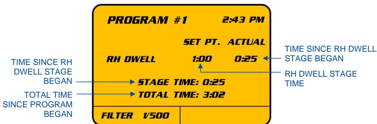
During the RH Dwell stage, the air is circulated inside the chamber. Additional humidity will not be added during this stage, so do **NOT** open the Main Door or the CA Chamber Door.
