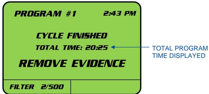
After the Fuming Cycle is complete, this screen will be displayed, along with an audible beep and flashing chamber light, for 30 minutes or until the Main Door is opened. Upon completion of the Fuming Cycle the doors will unlock automatically, so that evidence and the used CA tin can be removed.
