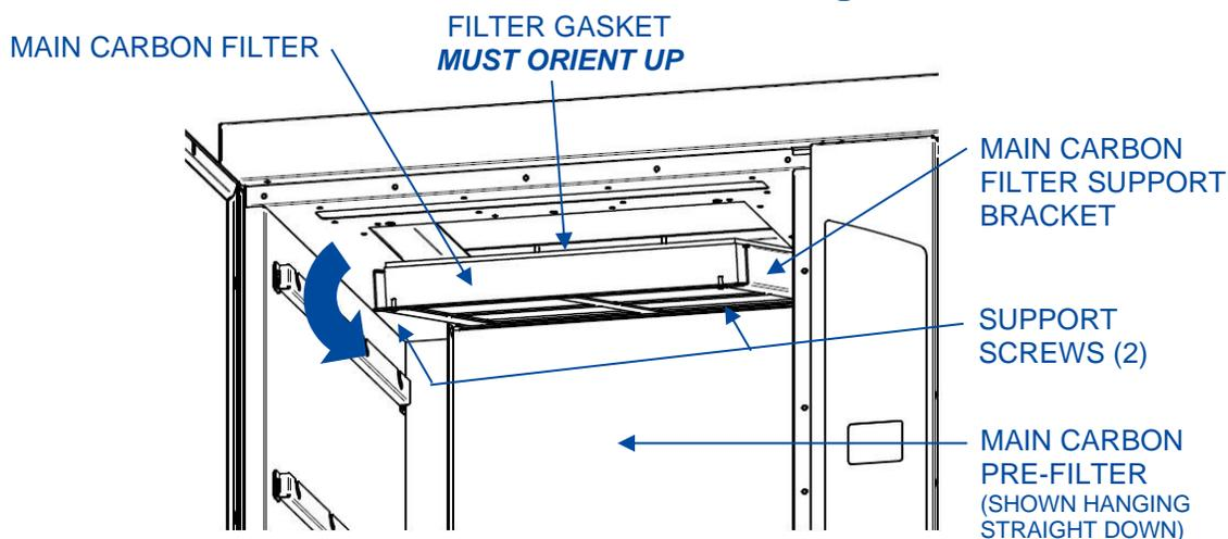
6. After new Carbon Filters are installed, the Filter Life Gauge needs to be reset to zero. On the Main Menu screen, Select **SERVICE**, and press **[OK]**. Enter Password: **[UP] [DOWN] [LEFT] [RIGHT] [OK]**. After entering the Servicer password, select **FILTER**, and press **[OK]**. Accept the Warning by pressing **[OK]**, then select **YES** on reset option, and finally press **[OK]**, to reset Filter Life (see Fig. 7-6).
