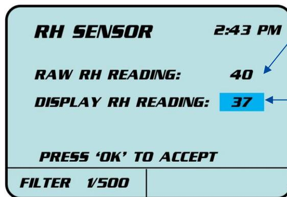
**NOTE!** DISPLAY READING CAN ONLY BE ADJUSTED +20%/-10% FROM RAW READING
