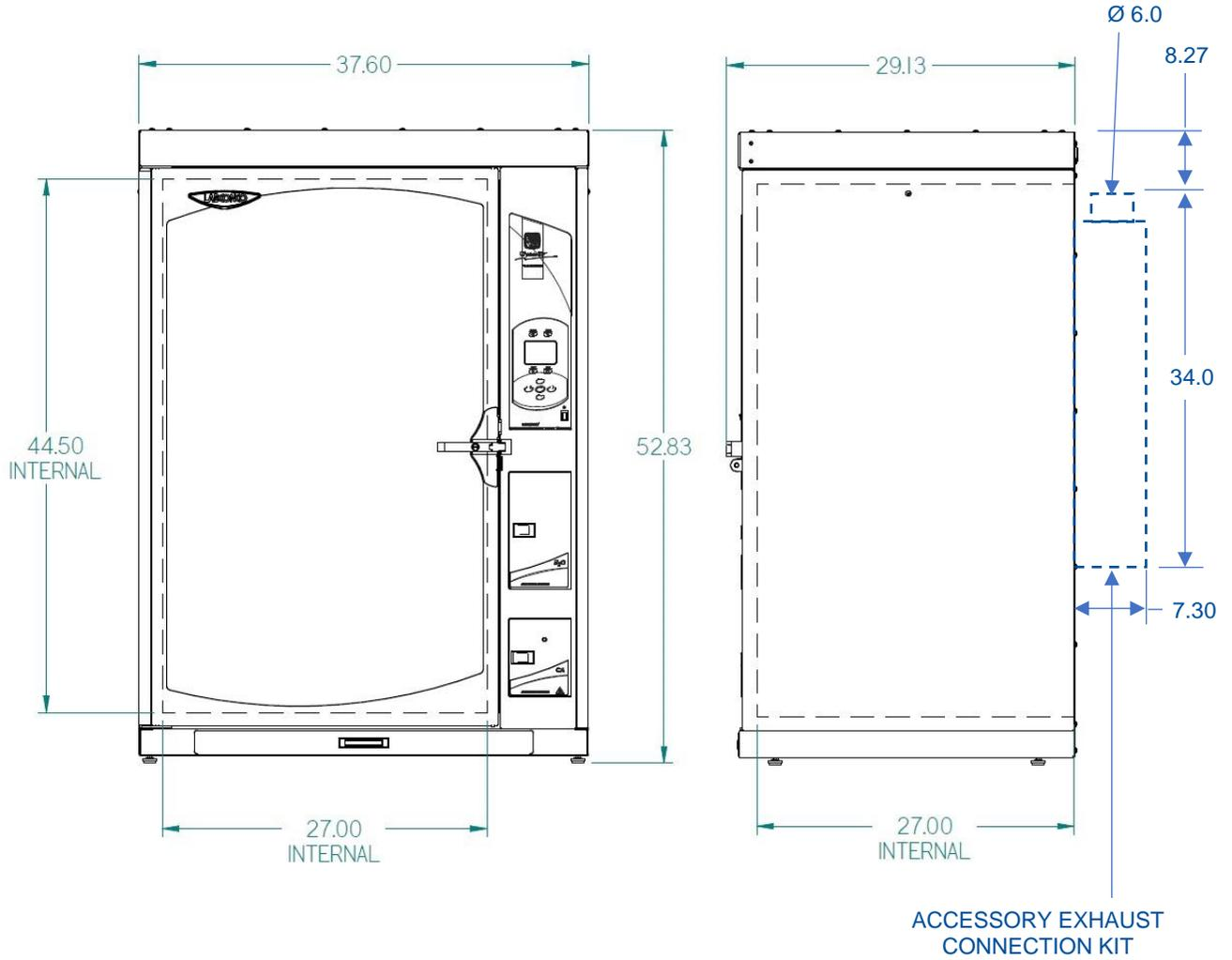
The External and Internal Dimensions of the CApture BT Fuming Chamber mounted on the Accessory Stand (P/N 3182900) are shown in Fig. B-2.
