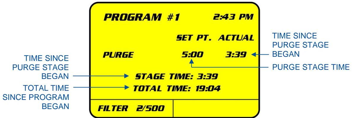
The Purge stage is the final stage in a Fuming Cycle. During this stage, you will hear the exhaust blower turn on to pull the fumes inside the chamber through the Main Carbon Filter. This stage has a minimum time of 4:00 to ensure all CA vapors are removed. Until this stage is complete, the doors will remain locked.
