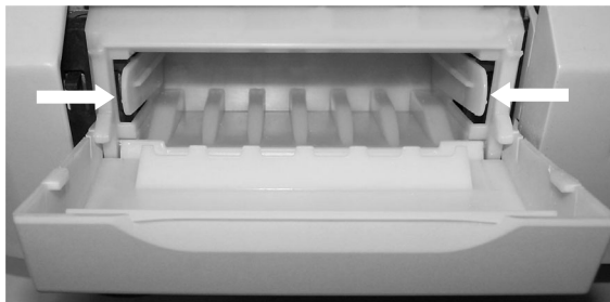
Fig. 6-8: Removing the strip preparation tray
