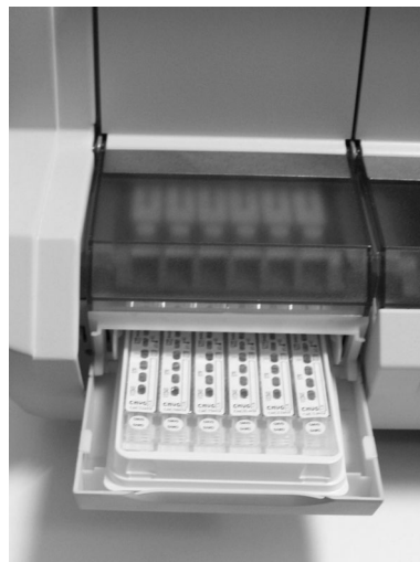
Fig. 2-7: Reagent strips placed on the strip preparation tray with their boat
