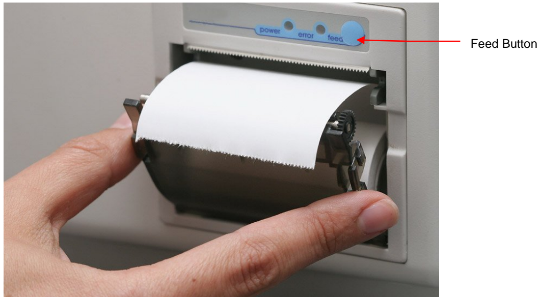
Figure 45 - Insert Paper Roll into printer
