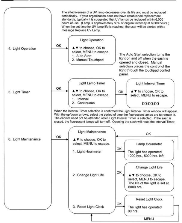
The fluorescent light intensity will wane with time. This maintenance feature is a convenient reminder to replace the light periodically. Reset the clock when the light is replaced. A reminder will appear on the display when the set Light Life is reached.
