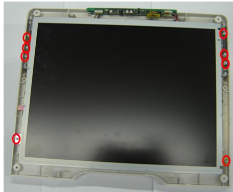
Figure 7-45 Disassemble the LCD Screen (1)
