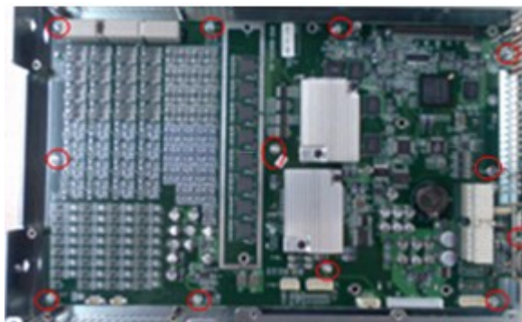
Figure 7-25 Disassemble the Main Board
