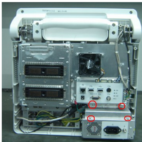
Figure 7-22 Disassemble the Main Board Assembly (1)
