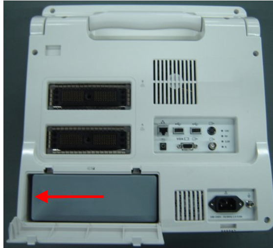
Figure 7-3 Disassembly of Battery (2)
