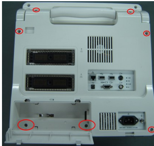
Figure 7-4 Disassembly of Rear Cover Assembly of Main Unit (1)
